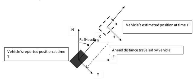
Figure XI-1 GNSS Position Extrapolation
