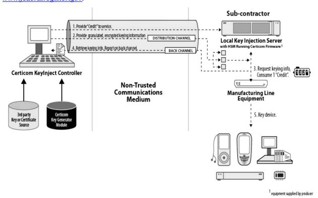
Figure V-4 Secure device manufacturing in an untrusted environment
