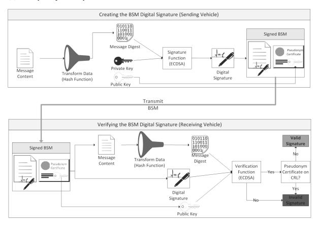
Figure III-9 BSM Digital Signature Generation
