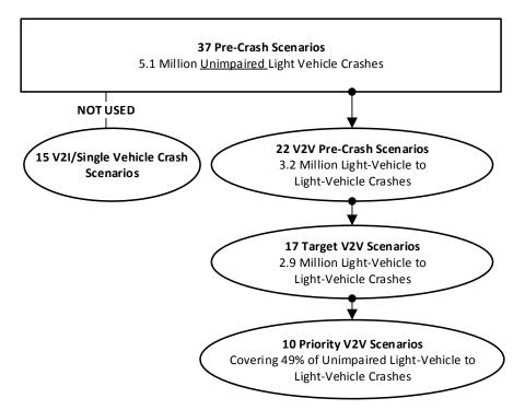
Figure II-2 V2V Pre-Crash Scenario Breakdown<sup>16</sup>
