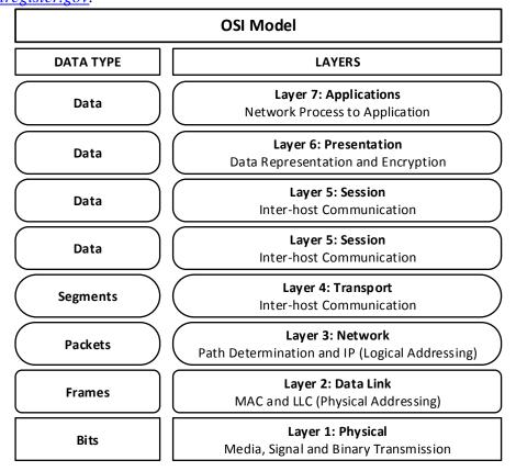
Figure III-5 OSI Stack
