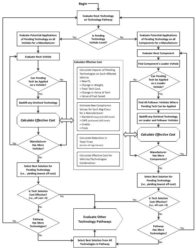
Figure 10. Determination of "Best Next" Technology Solution
