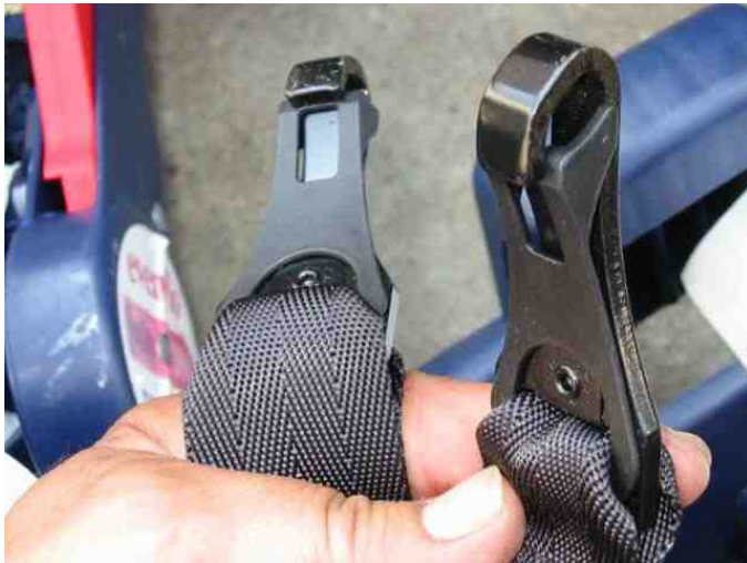
Typical Soft Anchor, Lower LATCH Attachments
