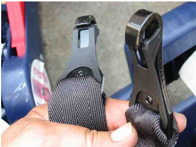
Typical Soft Anchor, Lower LATCH Attachments
