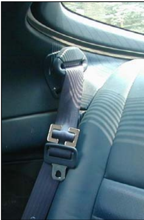
Locking clip correctly positioned on belt webbing near sliding latch plate
