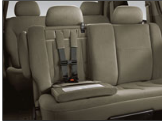
Older 5-point harness type of integrated CRS (typically seen in many older minivans)
