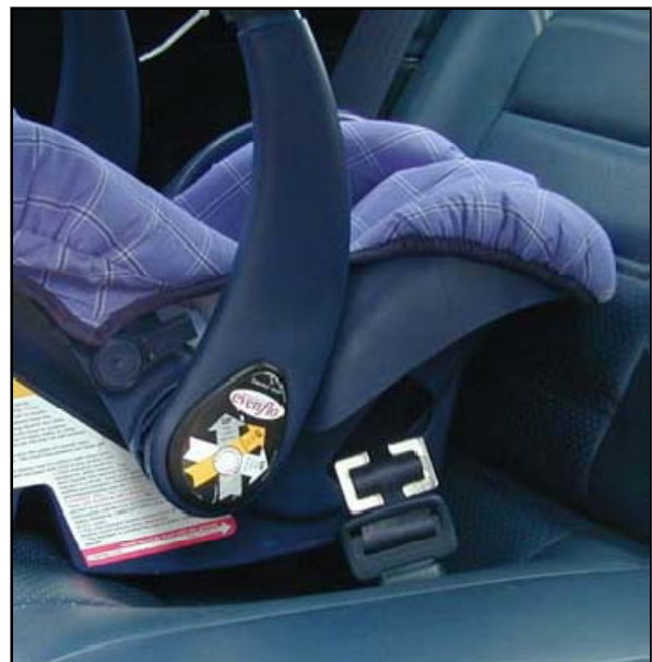
Locking clip correctly positioned on belt webbing near sliding latch plate
