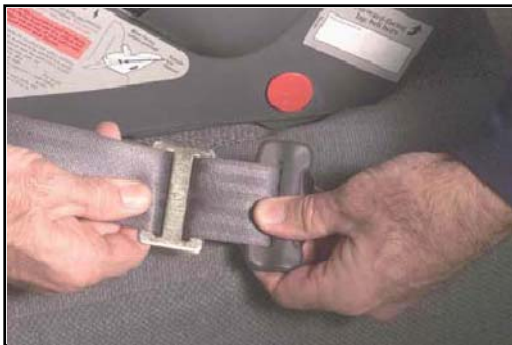
Locking clip affixed to belt webbing no more than 1 inch above latch plate
