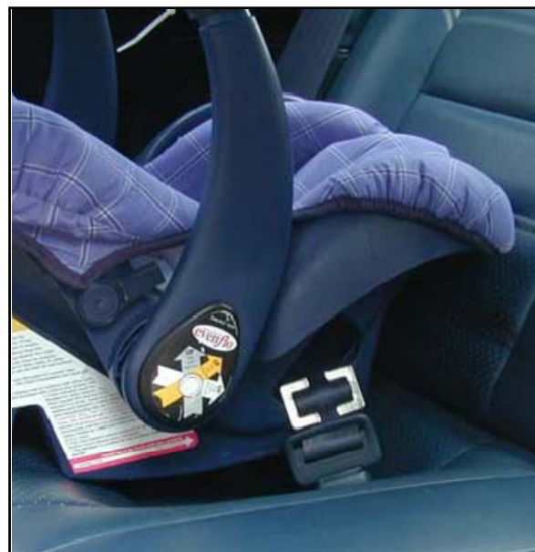
Locking clip correctly positioned on belt webbing near sliding latch plate
