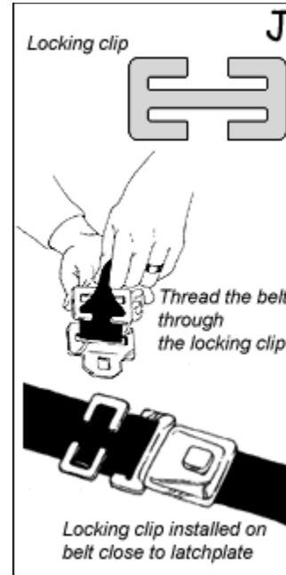
General instructions on how to position locking clip
