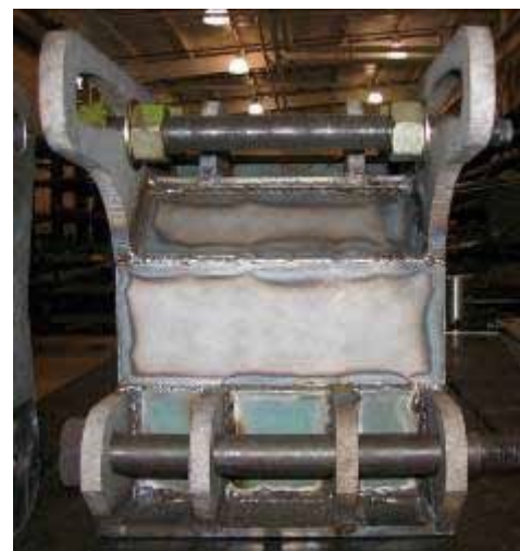
Figure 4.20: Left: 8 th and 9 th steps have been completed and jiggling has been removed. Right: 12 th step has been completed; cover plates were welded in place. Note: Jigs holding the Lower Adjustment Brackets should be left in when welding is taking place on the Inboard Beam. Free play tolerances were lost when those jigs were removed and welding operations performed.
