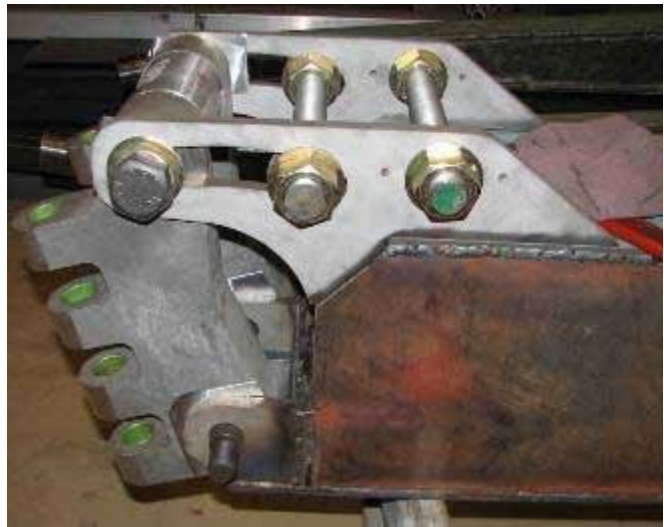
Figure 4.19: Left: 1 st step complete clamps have been removed. Right: 7 th step, critical placement of the Lower Adjustment Brackets. Hinges, all thread, and shims are used to jig into place. Consider tack welding on some straps across the brackets to further constrain warping.
