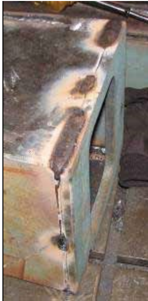
Figure 4.3: Left: Base Plate is added to the end. Middle: Base plate is welded to the Outboard Beam in the locations that the Hinge Brackets will overlap. Right: Hinge Brackets are being jugged up to weld. The bolts shown in the photo were removed and an aluminum jig was inserted into the holes to assure alignment, see Figure 4.4 (Middle).
