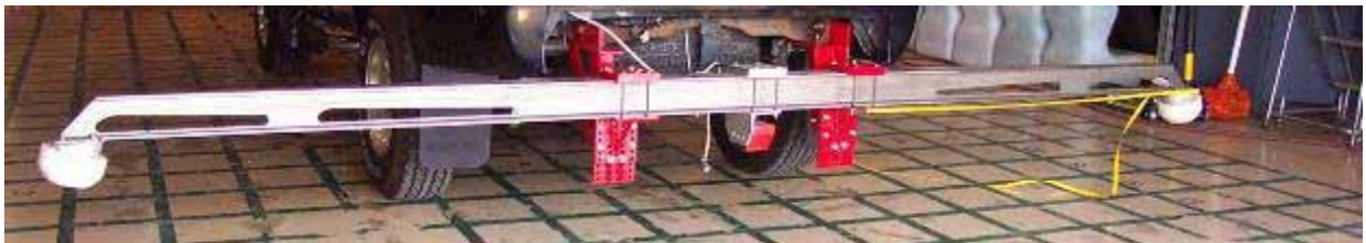
Figure 3.4: Photo shows example of NHTSA's light vehicle titanium outriggers. Outrigger has hemispherical skid pucks mounted at the ends of the outrigger. The pucks are made of Ultra-High Molecular Weight (UHMW) plastic and they have been found to be a very light and durable especially when compared to castors assemblies.
