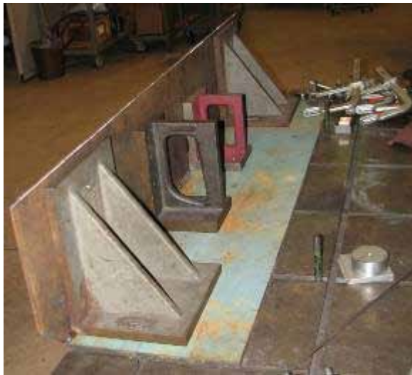
Figure 4.19: Left: 1 st step complete clamps have been removed. Right: 7 th step, critical placement of the Lower Adjustment Brackets. Hinges, all thread, and shims are used to jig into place. Consider tack welding on some straps across the brackets to further constrain warping.
