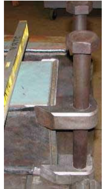
Figure 4.3: Left: Base Plate is added to the end. Middle: Base plate is welded to the Outboard Beam in the locations that the Hinge Brackets will overlap. Right: Hinge Brackets are being jugged up to weld. The bolts shown in the photo were removed and an aluminum jig was inserted into the holes to assure alignment, see Figure 4.4 (Middle).
