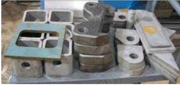
Figure 4.18: Left: Small parts needed to assemble the new outriggers. Right: Large plates that are welded together to make up the shell of the Inboard Beam.
