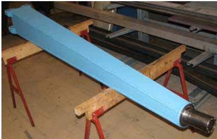
Figure 4.7: Finished welded and painted Outboard Beam.
