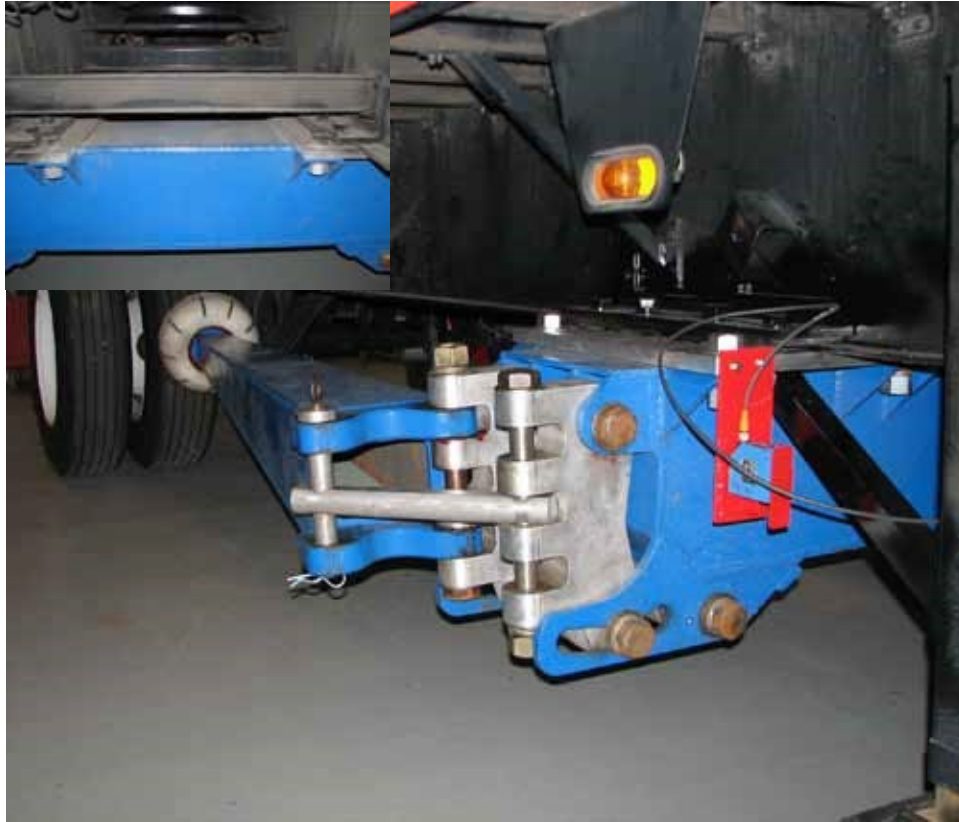
Figure 5.1: Center: shows the main beam of the new outriggers mounted to a 28ft. flatbed type trailer. The main trailer rails are clamped on the outside and insides Upper Left: Shows the inside flanges of the trailer main rails were clamped and bolted to the outrigger adapter plate.
