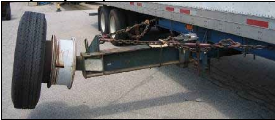
Figure 3.3: Photo of the UMTRI outrigger truck wheel/tire axle assembly; it uses a dual wheel with one tire mounted on the outer rim.
