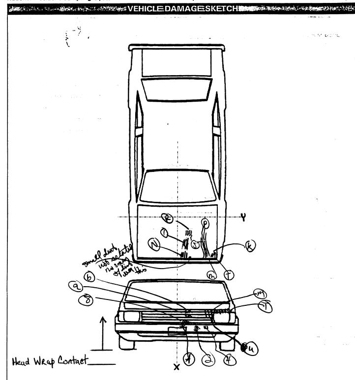
NOTES: Sketch all pedestrian contacts, include the size and depth in centimeters. Locate the pedestrian contacts from the intercept point of the centerline (lateral) and the front axies (longitudinal) in centimeters. Annotate observations which might be useful in reconstructing the accident (e.g., grass in tire bead, direction of striations, scuff on sidewalls, etc.).
