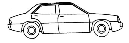
NOTES: Sketch all pedestrian contacts, include the size and depth in centimeters. Locate the pedestrian contacts from the intercept point of the centerline (lateral) and the front axles (longitudinal) in centimeters. Annotate observations which might be useful in reconstructing the accident (e.g., grass in tire bead, direction of striations, scuff on sidewalls, etc.).
