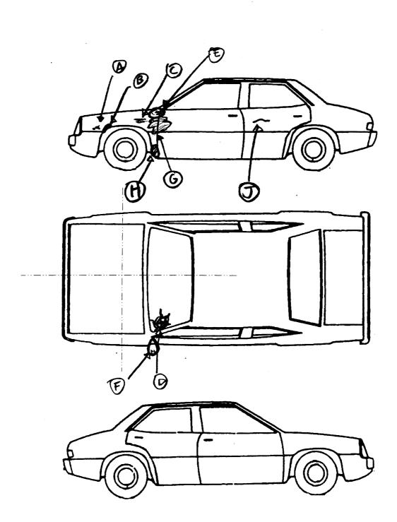
NOTES: Sketch all pedestrian contacts, include the size and depth in centimeters. Locate the pedestrian contacts from the intercept point of the centerline (lateral) and the front axles (longitudinal) in centimeters. Annotate observations which might be useful in reconstructing the accident (e.g., grass in tire bead, direction of striations, scuff on sidewalls, etc.).
