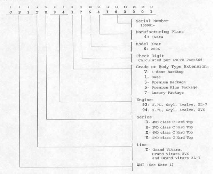
Note: 1. JS3: Make code for SUZUKI (Suzuki Iwata production)
