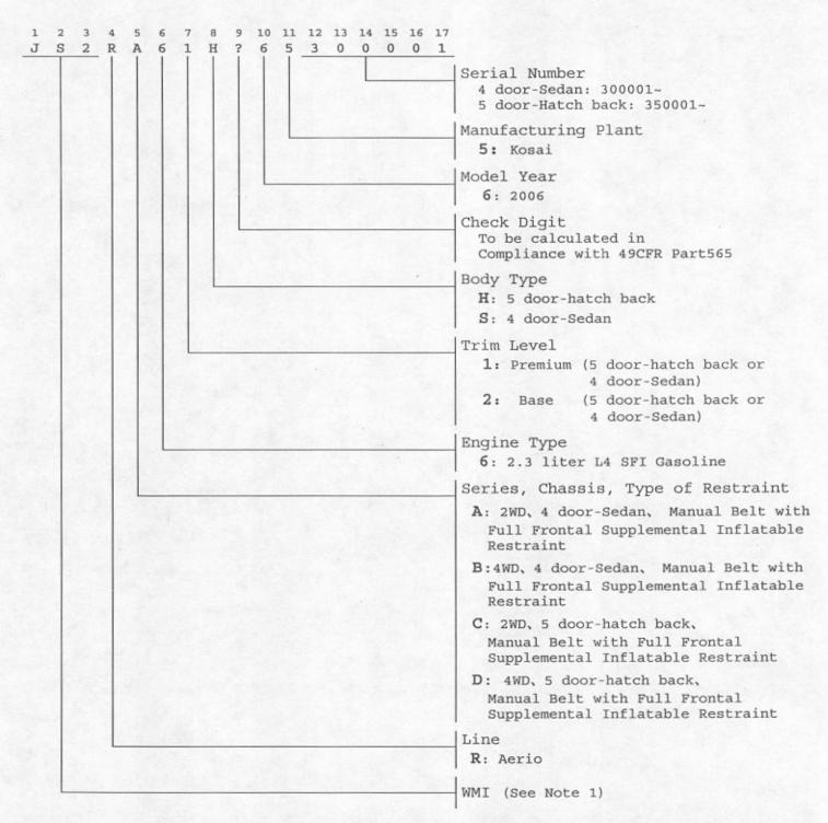
Note: 1. JS2: Make code for SUZUKI (Suzuki Kosai production). Vehicle for sale in U.S. and Canada
