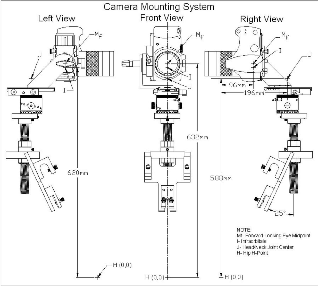
**Figure 23. Camera Mounting System, Three Views, with Coordinates (M<sub>f</sub>, I, J, H)**
