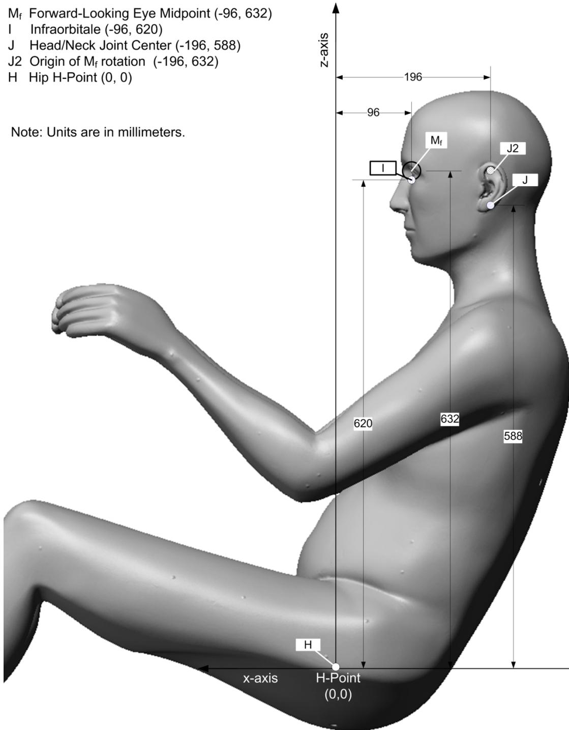
**Figure 4. Coordinates of the Forward-Looking Eye Midpoint (M<sub>f</sub>) and Joint Center (J) of Head/Neck Rotation of a 50th Percentile Male Driver with respect to the H-Point (H) in the Sagittal Body Plane.**
