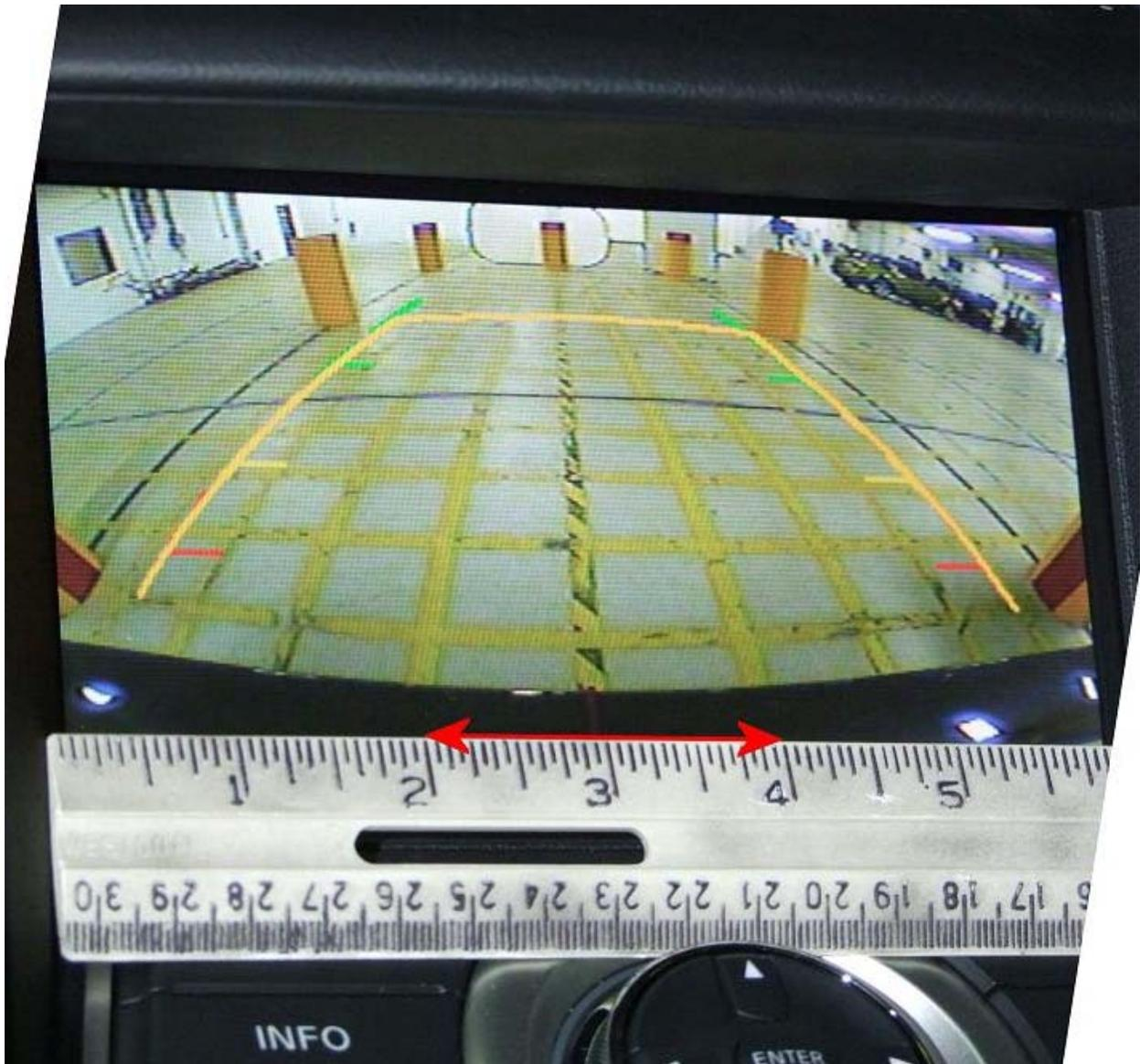
Figure 13. Field of View and Image Quality Assessment Photo for the 2010 Nissan Maxima
