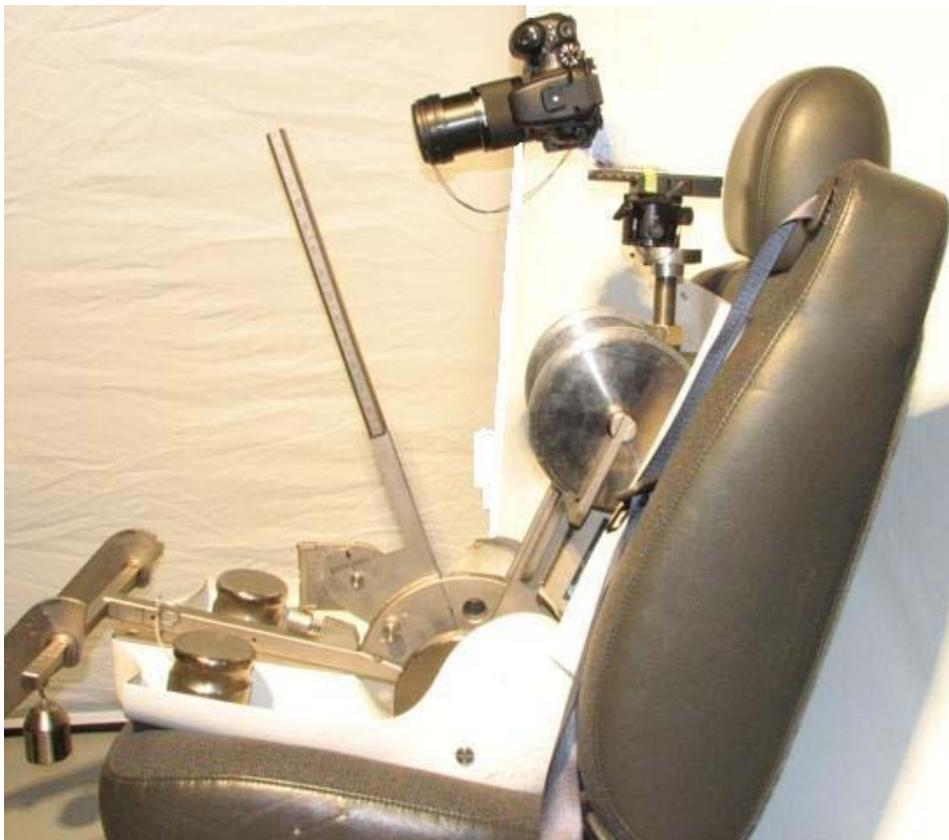
**Figure 5. Rearview Image Measurement Fixture**
