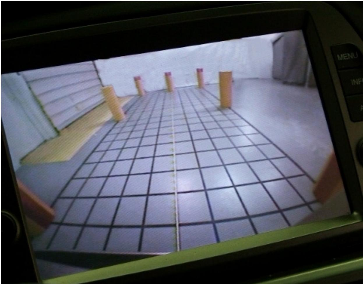
**Figure 8. Test Object Arrangement as Displayed in Rearview Image**
