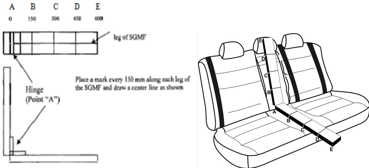
Figure 1. SGMF sketch (left), SGMF positioned in a vehicle rear seat.
