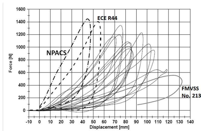
**Figure 3. Dynamic force-displacement curves of seat cushions on vehicle rear seats (black thin) and ECE R.44 seat foam (black-dashed), NPACS seat foam (black-dashes and dots), and FMVSS No. 213 seat cushion (black bold).**
