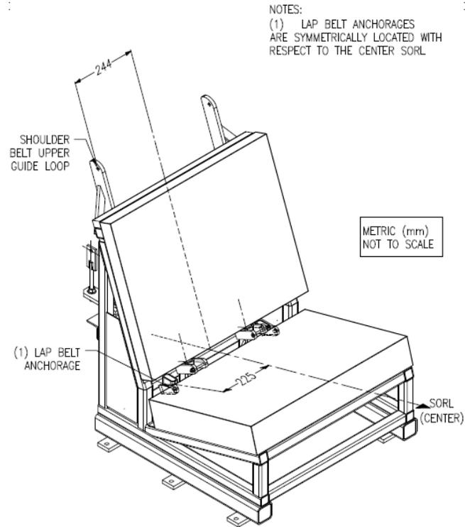
SEAT ORIENTATION REFERENCE LINE AND SEAT BELT ANCHORAGE POINT
