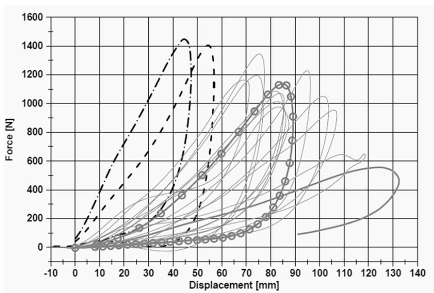
**Figure 4. Dynamic force-displacement (stiffness) of ECE R.44 seat foam (black-dashed), NPACS seat foam (black-dashes and dots), FMVSS No. 213 seat cushion (dark grey solid), seat cushions on vehicle rear seats (light grey solid), and the proposed NHTSA-Woodbridge seat cushion (solid with circles).**
