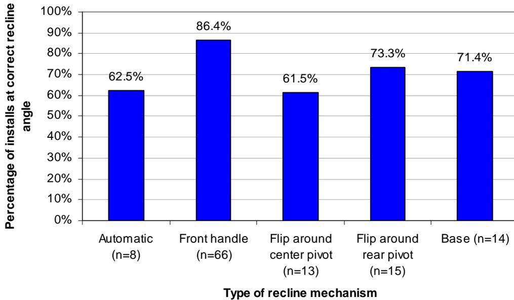
**Figure 26. Percentage of installs at correct recline angle.**
