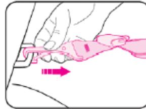
Pull on the end of the LATCH belt while pressing down on the center of the child restraint. Use your hand or knee to press on the child restraint. **LATCH belt must be tight.**
