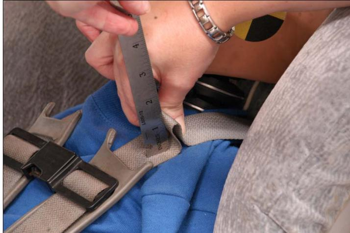
**Figure 8. Measuring amount of harness slack.**
