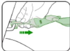
5 Press down and tighten LATCH belt
