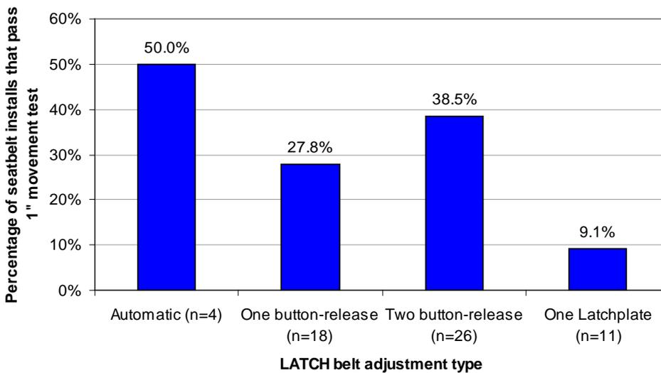
**Figure 19. Percentage of seatbelt installations passing 1" test for tightness by LATCH adjuster type.**
