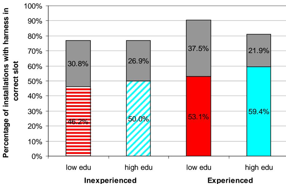
**Figure 25. Percentage of installations with harness in correct slot by subject education and experience. Lower part of each bar indicates correct slot selection, while upper part of bar indicates slot chosen was allowed for the RF or FF mode.**
