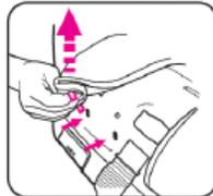
Now you can see the LATCH belt, which is attached to the child restraint but can be moved to each belt path.
