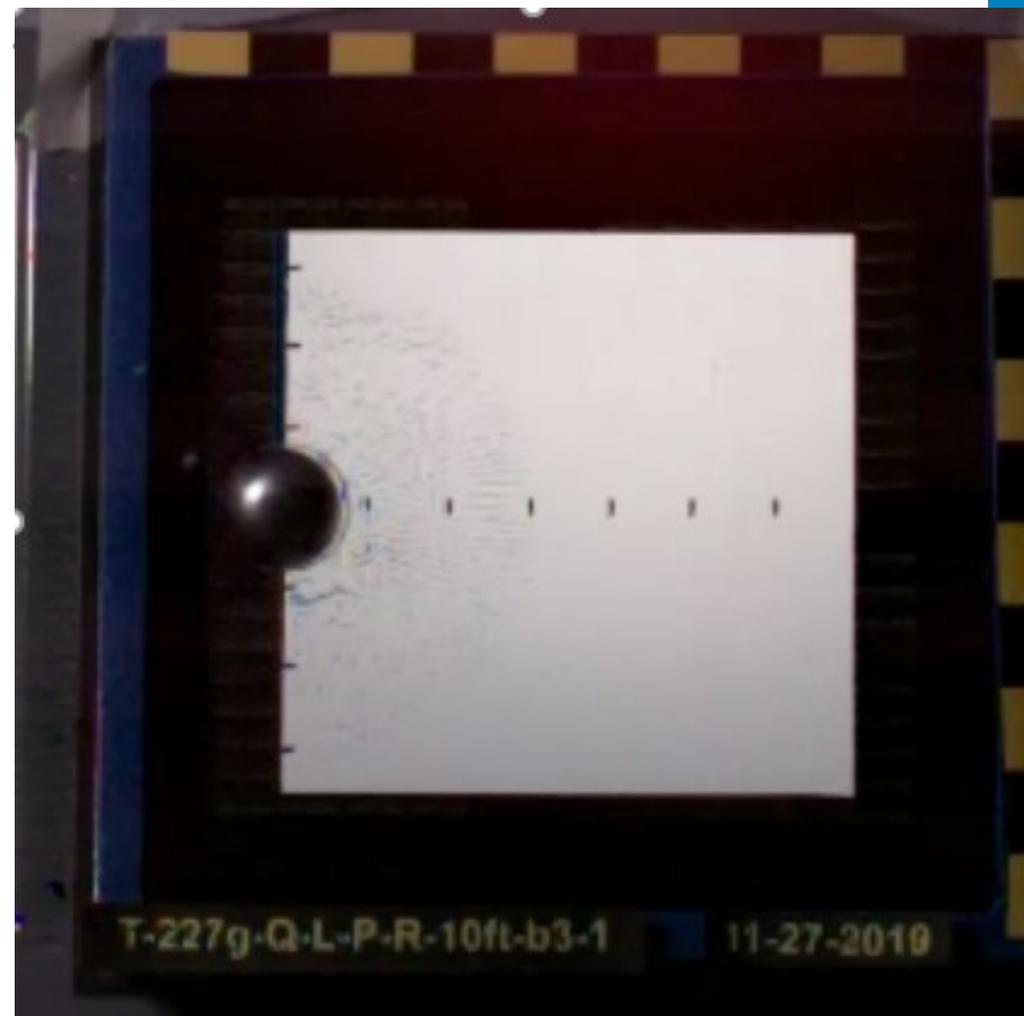
Still image of fracture – fracture can be seen moving outward from initiation point
