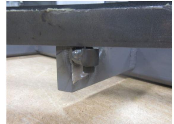
Screws to attach Rear Quarter Frame to Frame Fixture
