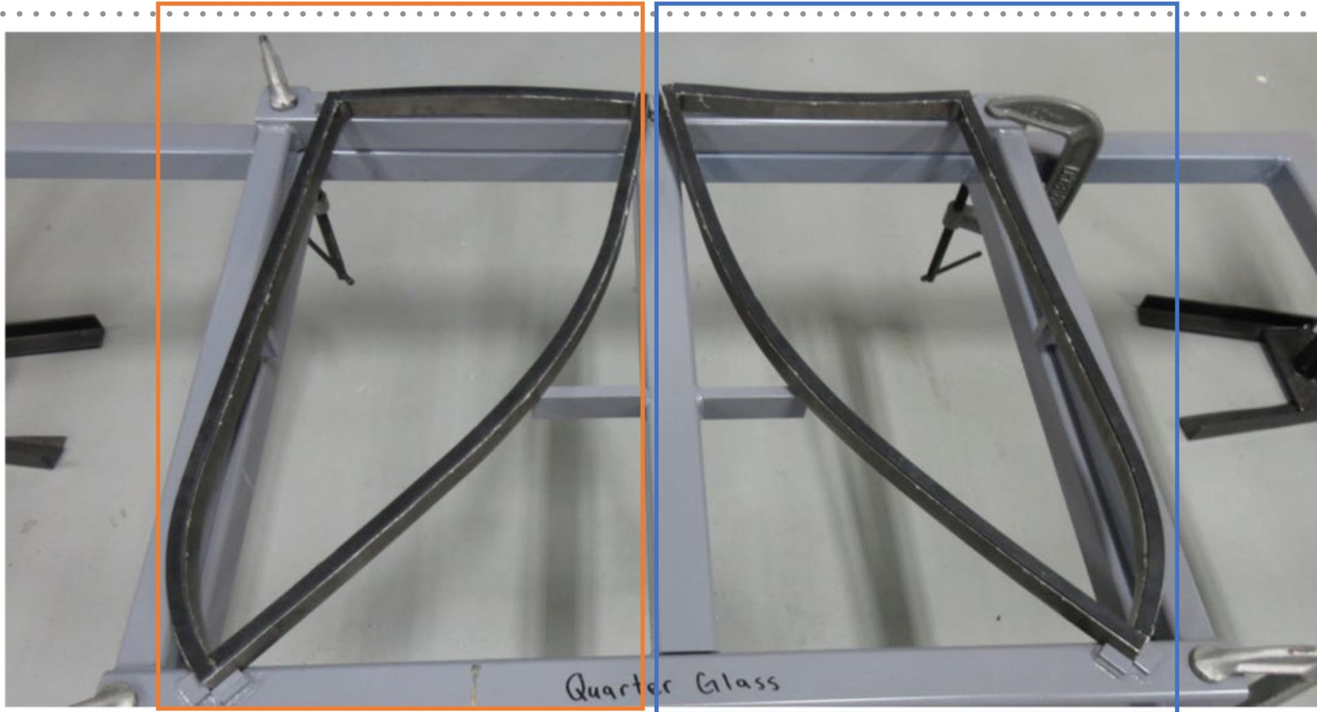
Depending on the type of test to be run (ball vs shot bag) the glass will be oriented to either impact the exterior or interior surface. The opposite side frame will be used as the top frame for the test
