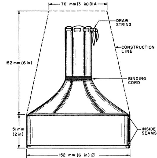
NOTE: Bag to be made of 0.79 mm (1/32 in) thick flexible leather. Use lead shot, BB size (4.57 mm in diameter). Total weight of bag and shot to be 4.961 to 5.018 kg (11 lb ± 1 oz).
