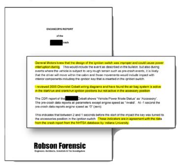
Thus, Shipp concluded: "General Motors' improper design resulted in a vehicle that was defective in a manner that caused the airbag to not deploy in a crash that General Motors has determined should have had an airbag deployment."
