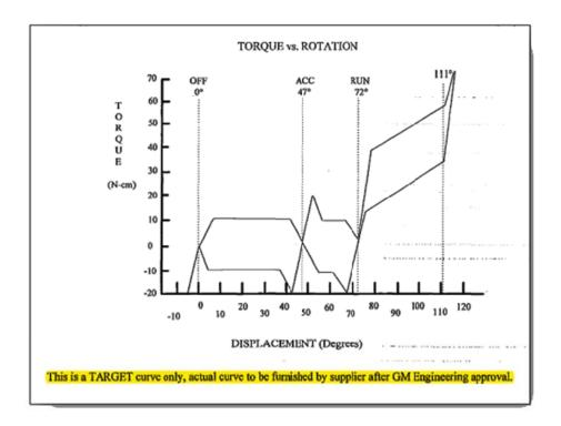
Section 3.2.2.3 described the desired feel of the switch – "smooth, with clearly defined detents" – and also provided that "[f]inal switch tactile feel is subject to GM Engineering approval." The Specification was revised in 1998 and 1999, without changes to the parameters for the torque required to rotate from Run to Accessory. 113
