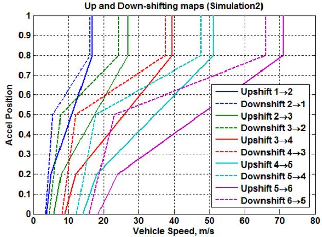
“gb\_ctrl\_dmd\_n\_gen\_eng\_mot\_not\_included\_detail.m” is created to match the shifting map based on test data.
