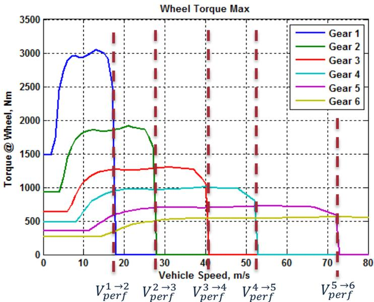
Maximum engine torque at wheels and performance upshift speeds
