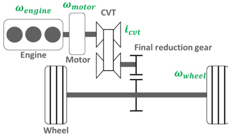
The engine and motor speed can be controlled independently of the vehicle speed, owing to the CVT's continuously variable feature
