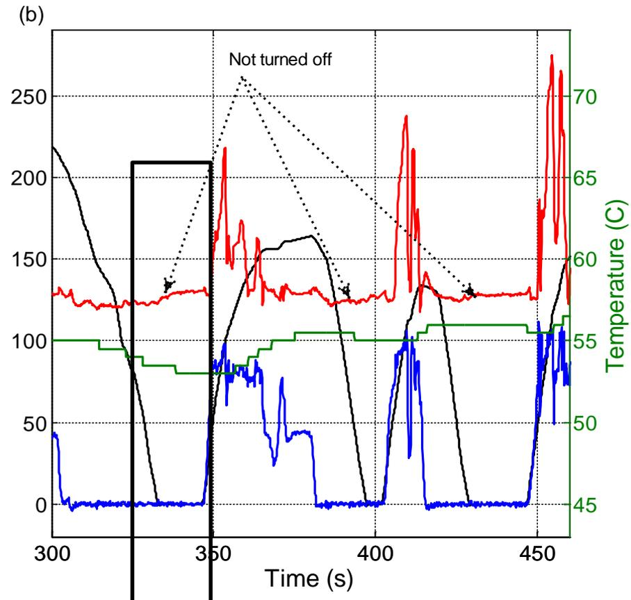
The engine is not turned off if the coolant temperature is low.
