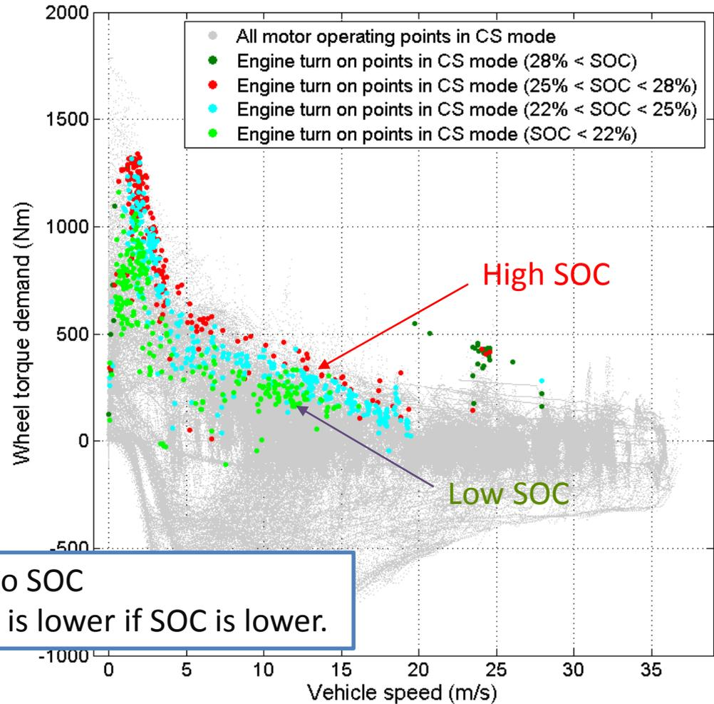
Threshold line is changed according to SOC
