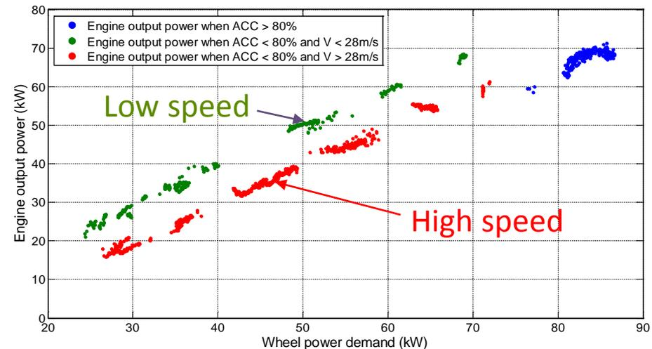
In CD mode, the engine is basically not used. However, the engine is mostly turned on for highway driving, so this special control concept is necessary for highway driving.
