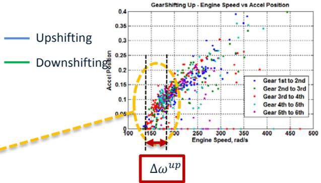
Design of upshifting and downshifting speed curves for two adjacent gears
