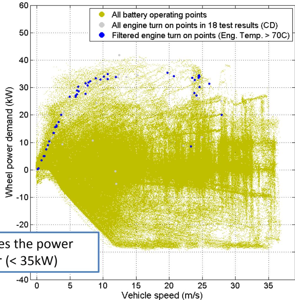
Engine turn on when the vehicle requires the power exceed battery maximum output power (< 35kW)
