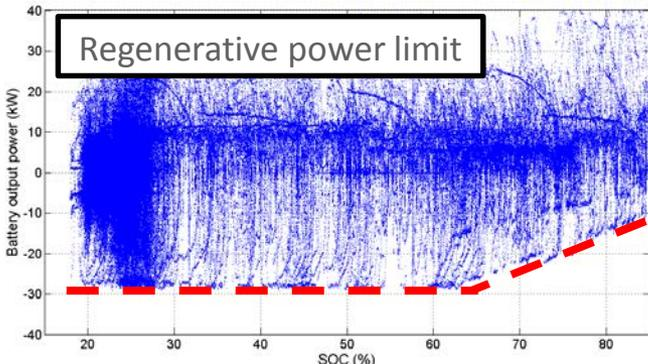
The battery in PHEV is constrained by SOC. (not observed in HEV due to SOC range)
