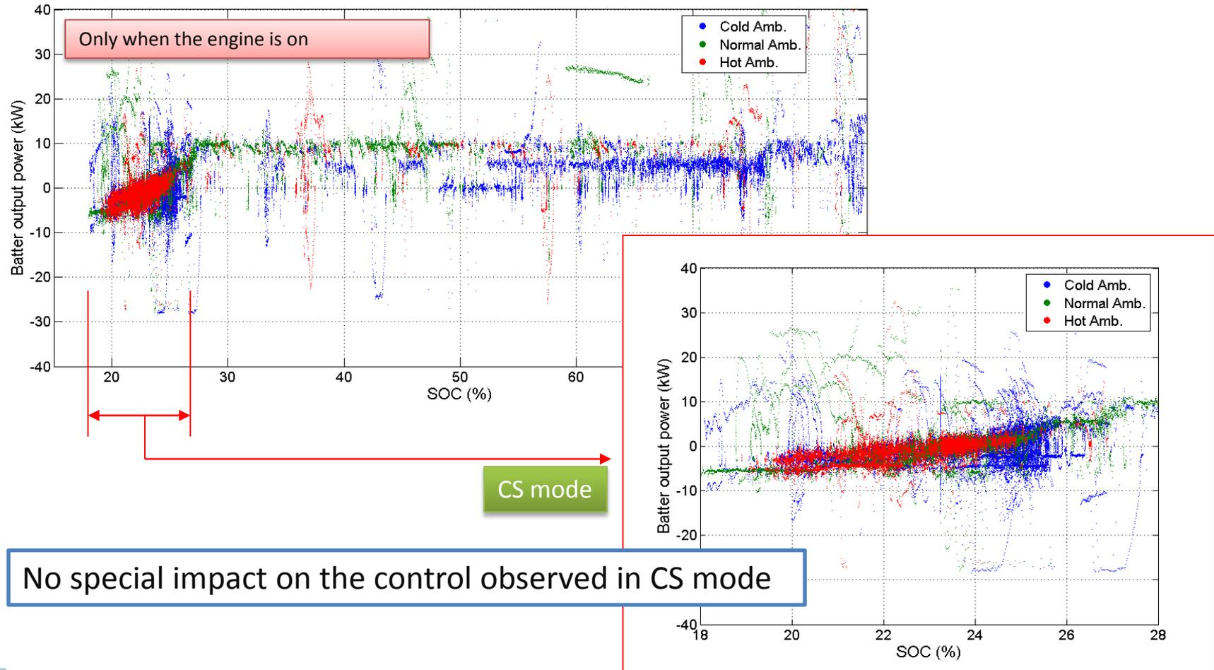
No special impact on the control observed in CS mode
