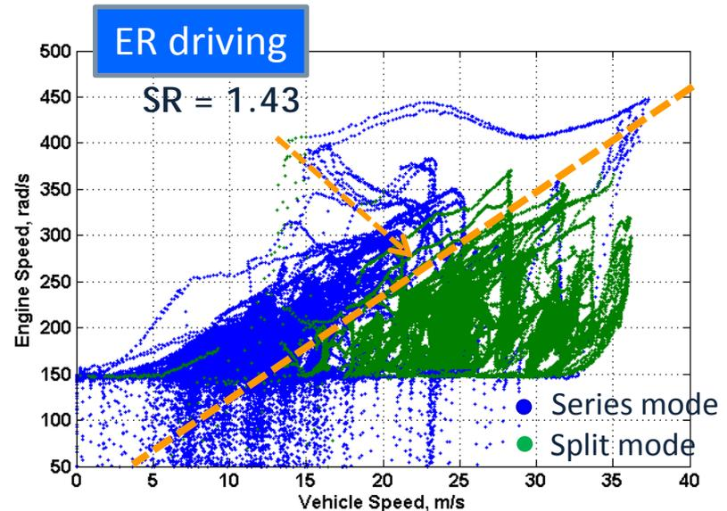
After we convert ER driving results into new map by using vehicle speed and engine speed indexes, the mode selection rule can be defined based on the speed ratio
