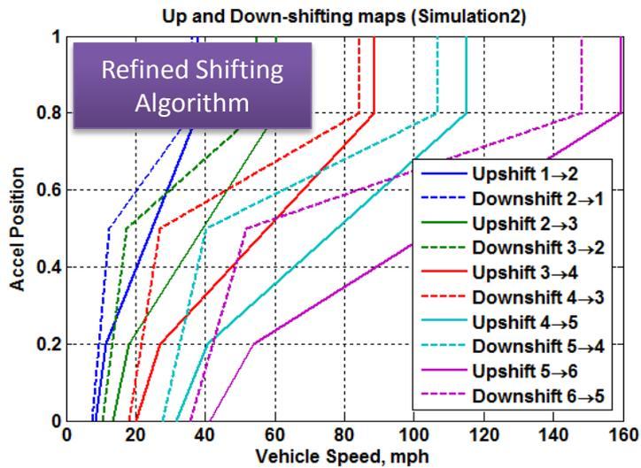
New shifting speed curves for a default light-duty vehicle in Autonomie
