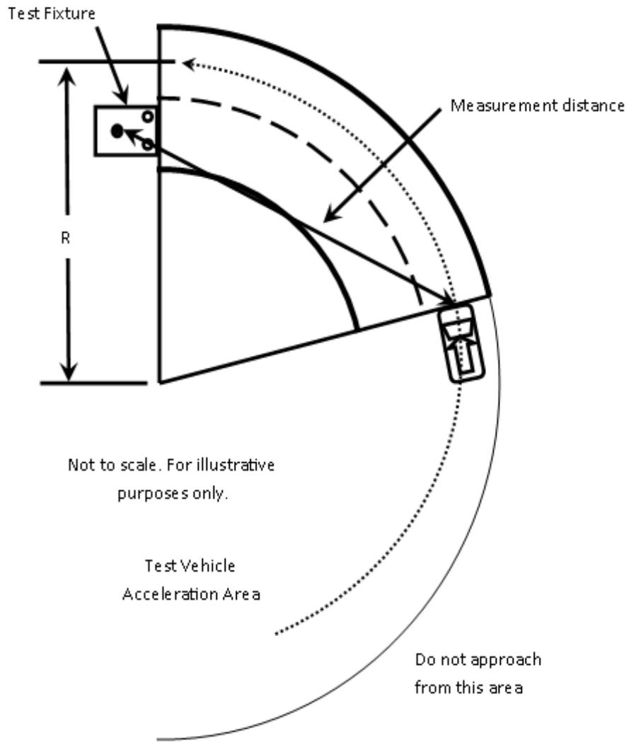
Figure 29 Left Curve Test Scenarios
