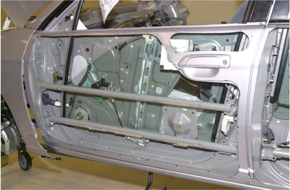
**Figure 3-7: Lightweight, tubular front door intrusion beams (2007 Civic)**
