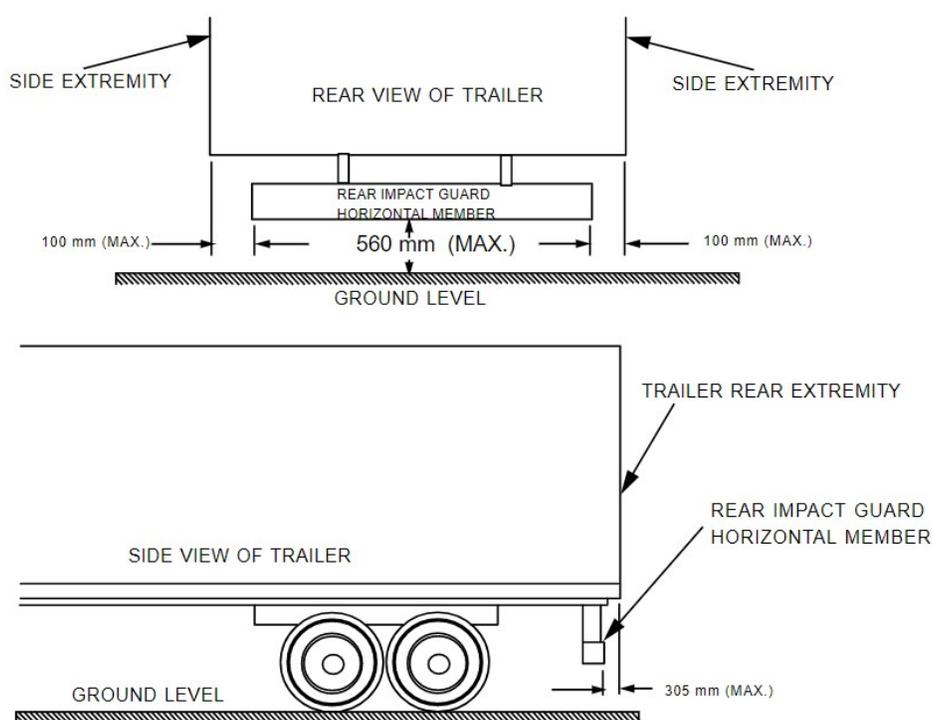
**Figure 3: FMVSS No. 224 configuration requirements**
