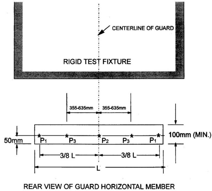
Figure 1: FMVSS No. 223 quasi-static test loading locations
