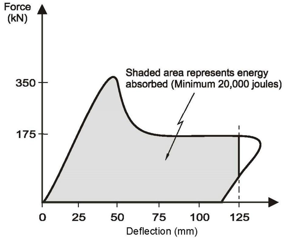
**FIGURE 3: UNIFORM DISTRIBUTED LOAD APPLICATION TEST**
