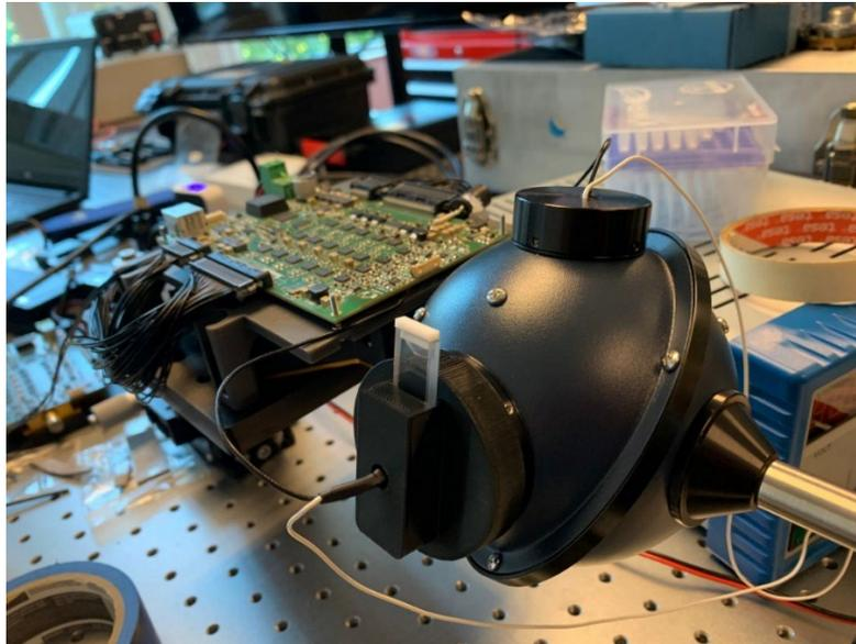
**Figure 8. The sensor setup includes a 3" integrating sphere, laser package, and electronic board**
