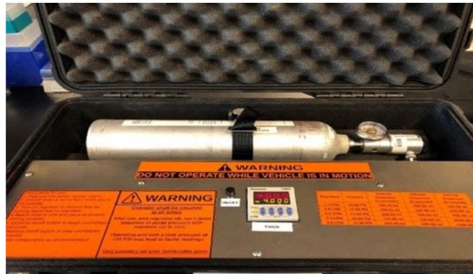
**Figure 10. Portable Gas SCD**
