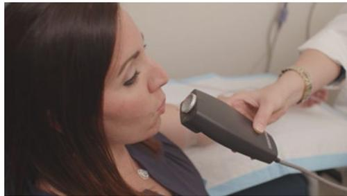
**Figure 13. Human subject testing using the DADSS breath sensor**
