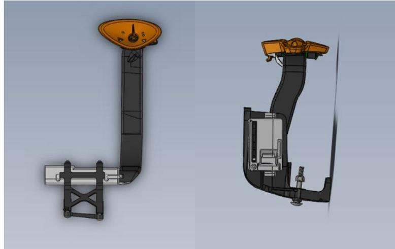
**Figure 11. Design of breath sensor delivery systems (snorkels) from the breath inlet port to the sensor**
