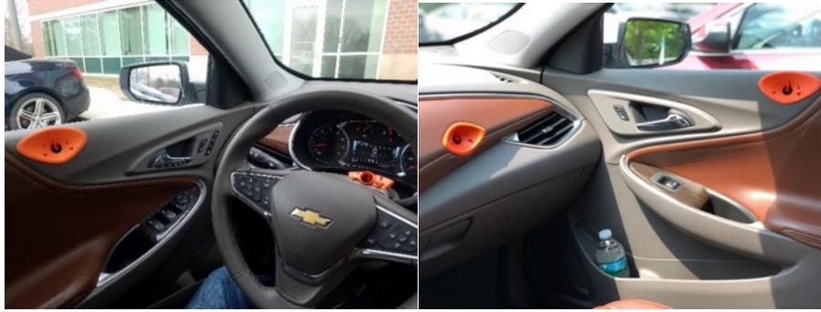
**Figure 15. Position of the breath sensors on the driver (left) and passenger sides of the vehicle**
