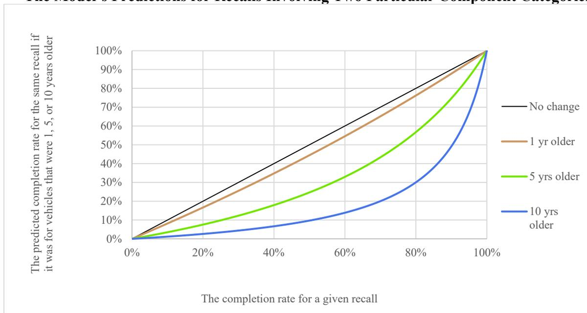
The graph indicates the effect of vehicle age, with a 5-year increase in age reducing a completion rate of 80% to below 60%. Note, however, that the data available to NHTSA cannot indicate the extent to which the vehicle age effect is truly a function of age or whether other factors—such as the demographics of owners of new vehicles or new vehicle warranty programs—play a significant role.
