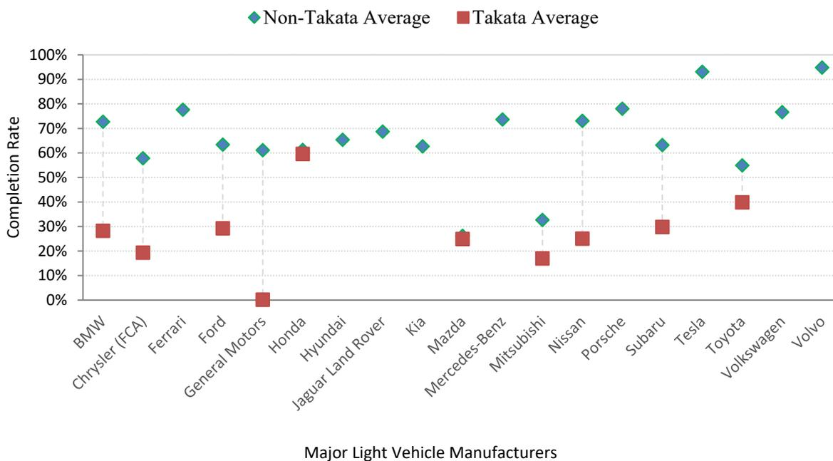
As shown in Figure 1b, the massive Takata air bag recall has had an adverse impact on the completion averages for many of the major manufacturers' recall rates. Due to the size of the collective manufacturers' recall programs, replacement parts supply was a significant problem.
