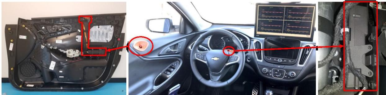
**Figure 9. Platform development 2017 Chevrolet Malibu integrated with the breath-based sensors.**
