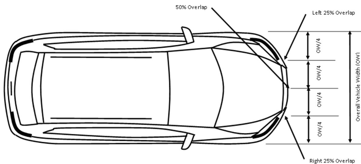
For the scenarios involving a pedestrian crossing from the right, two overlap conditions are proposed: A more challenging test condition of 25 percent overlap and a 50 percent overlap to ensure system robustness. The 25 percent overlap tests are performed only under daylight conditions, while the 50 percent overlap tests are performed in all lighting conditions. For the
