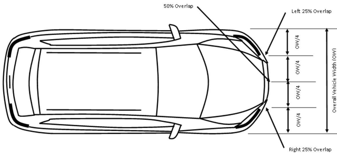
Figure 2. Setup for Lead Vehicle Automatic Emergency Braking
