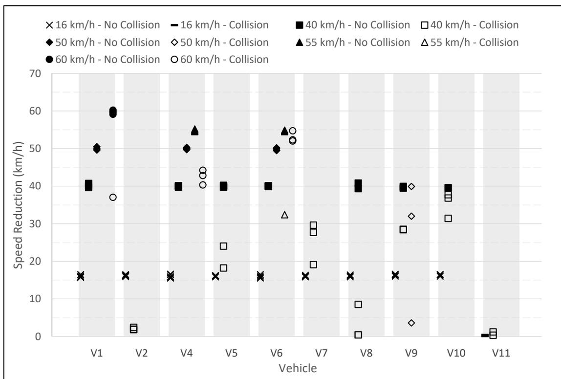
NHTSA upper beam testing using the stationary pedestrian along path scenario under dark lighting conditions resulted in one vehicle, V4, being able to avoid collision in all tests at speeds up to and including 55 km/h (34 mph). The vehicle achieved an average speed reduction of 48 km/h (30 mph) in three other tests conducted at 60 km/h (37 mph). Two other vehicles avoided collision in all tests at 40 km/h (25 mph) (See Table 33).
