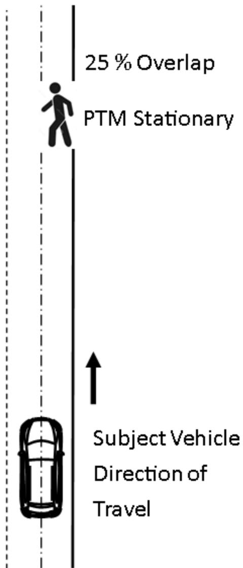
Figure 7. Setup for Pedestrian Along-Path Moving
