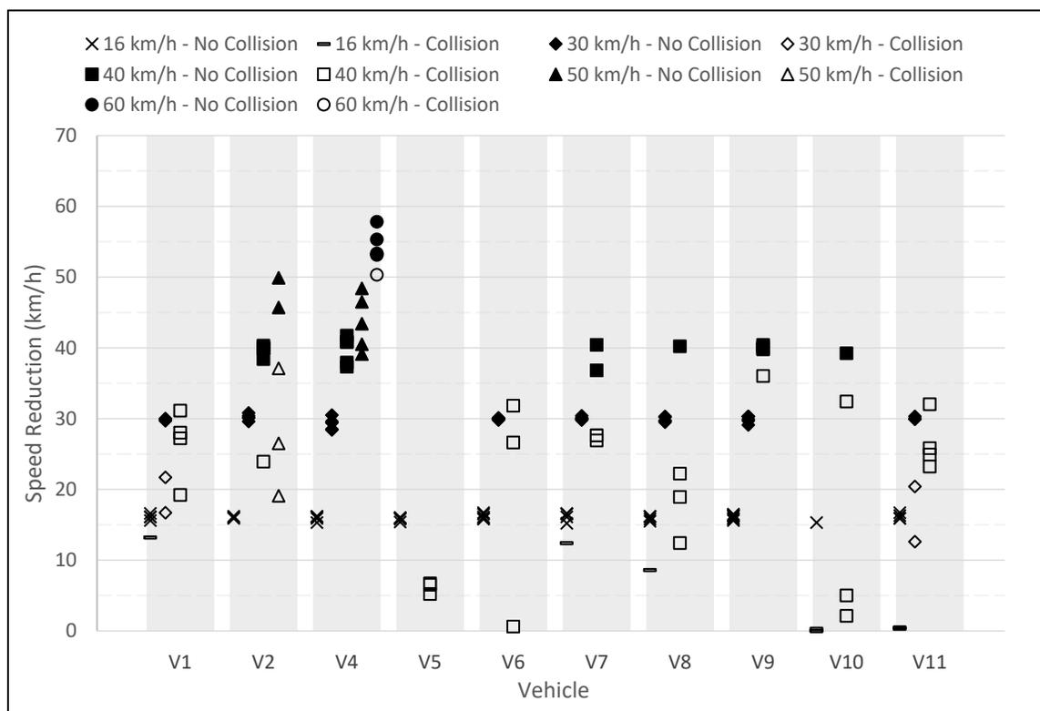
NHTSA's testing of the running adult pedestrian scenario (pedestrian surrogate travelling at 8 km/h (5 mph)) from the left was performed at speeds from 40 km/h (25 mph) to 60 km/h (37 mph) with a 50 percent overlap during daylight.<sup>190</sup> The results showed that five vehicles made no contact with the pedestrian surrogate in at least one test conducted at 60 km/h (37 mph) and
