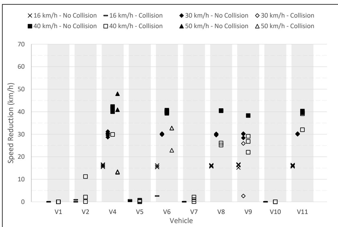
Testing for the obstructed running child (child pedestrian surrogate travelling at a speed of 5 km/h (3 mph)) scenario with a 50 percent overlap for the daylight condition found one vehicle that avoided collision in all tests up to 50 km/h (31 mph) and in four out of five tests from 60 km/h (37 mph). Another vehicle avoided collision in all but one test up to 40 km/h (25
