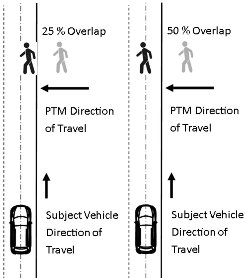
Figure 4. Setup for Pedestrian, Crossing Path, Left
