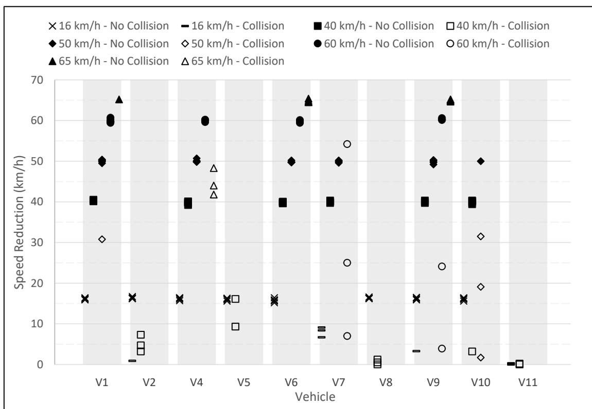
Testing for the dark upper beam along path pedestrian test mannequin moving scenario produced better performance than when testing for the dark upper beam stationary scenario. In the along path moving scenario, the test mannequin moves away from the subject vehicle at a
