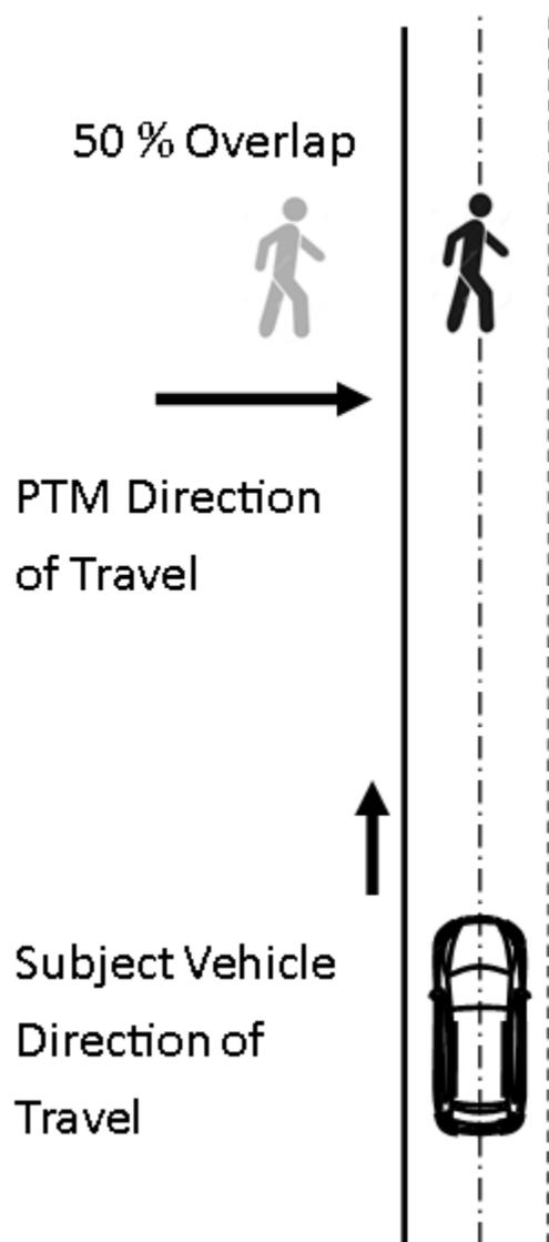
Figure 5. Setup for Pedestrian, Obstructed
