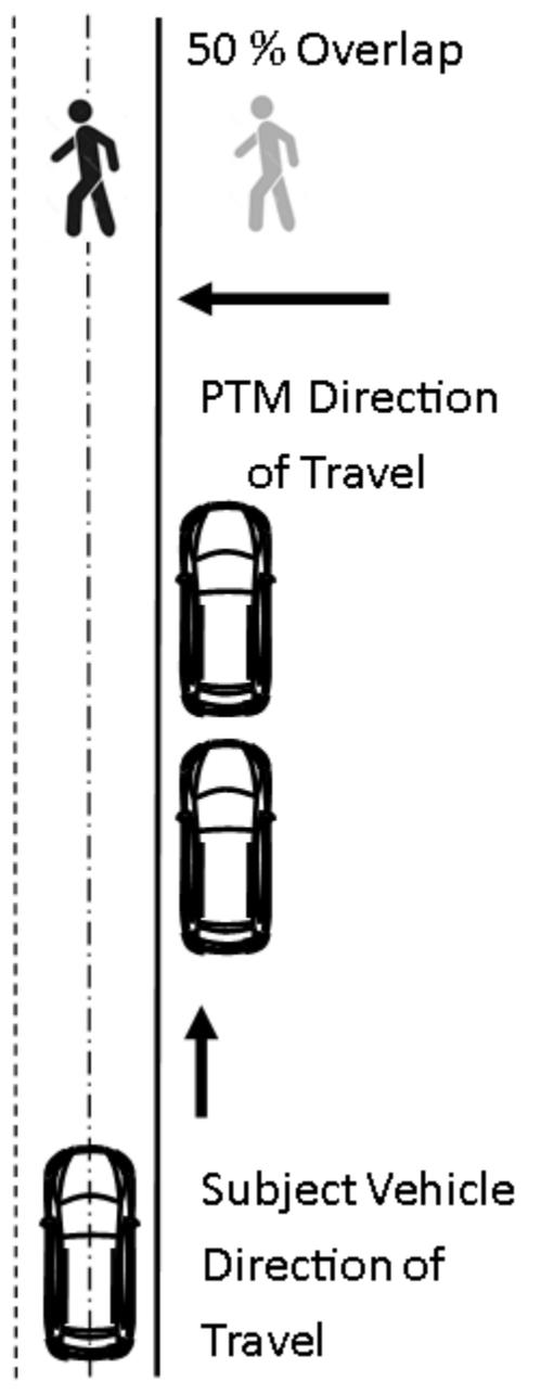
Figure 6. Setup for Pedestrian Along-Path Stationary
