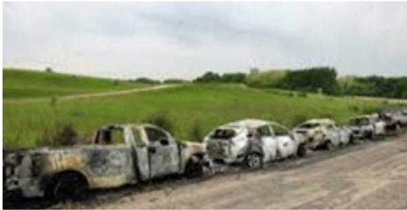
2011 Chevy Volt Latent Battery Fire at DOT/NHTSA Test Facility
