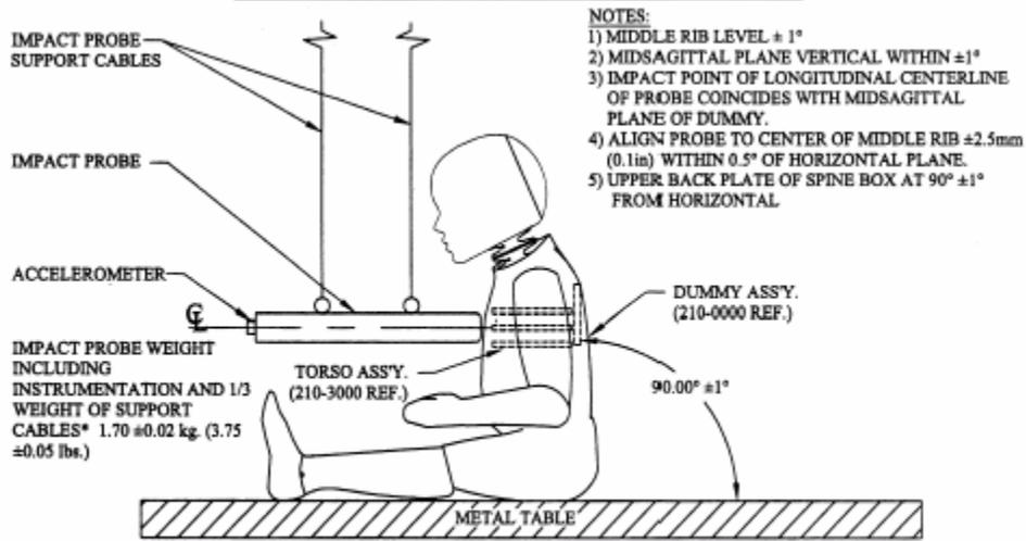
\* 1/3 WEIGHT OF PROBE SUPPORT CABLES AND THEIR ATTACHMENTS TO THE IMPACT PROBE NOT TO EXCEED 5% OF THE TOTAL IMPACT PROBE WEIGHT.
