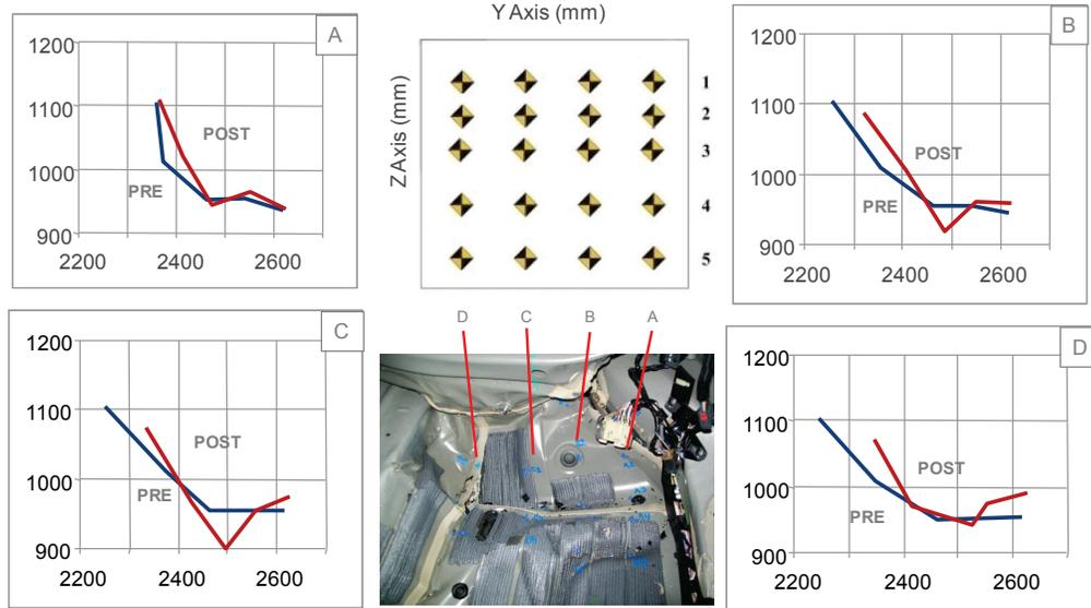
**Figure 18 - Passenger Side Toe Pan Intrusion From Pole35 Baseline (Test #090922)**
