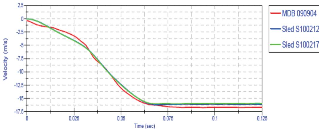
**Figure 35 - Velocity Profile Comparison Between Vehicle CG and Sled Tests**
