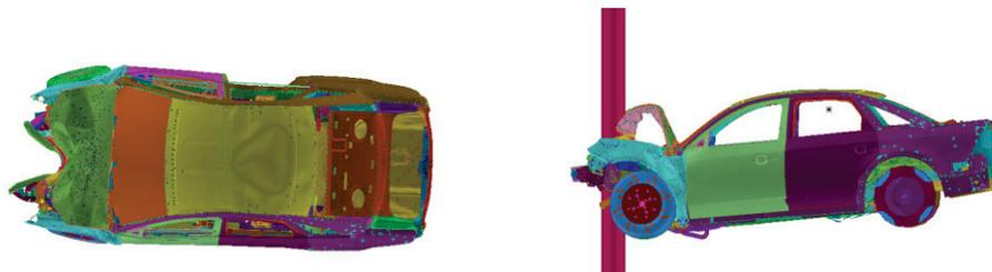
**Figure 9 - Top and Side View of PVP Centerline Pole at 35 mph**
