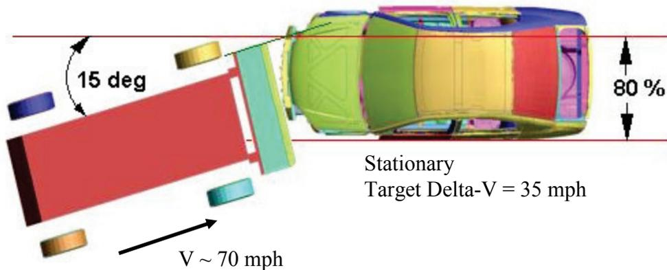
**Figure 10 - 15 Degree PDOF, 80-Percent Overlap MDB-to-Vehicle Analysis Setup**
