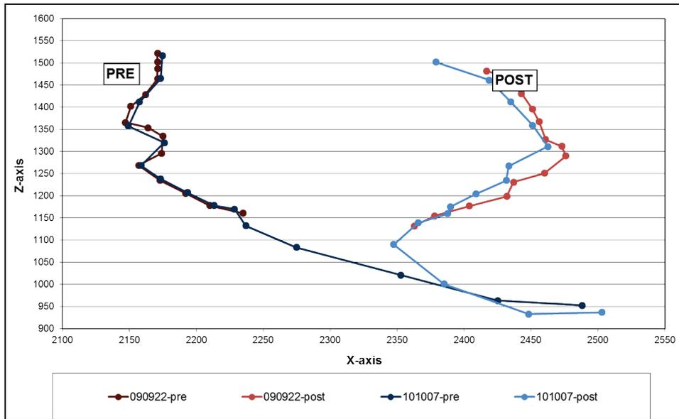
Figure 48 - Dash Panel Intrusion Profile – Passenger Side, Pole35
