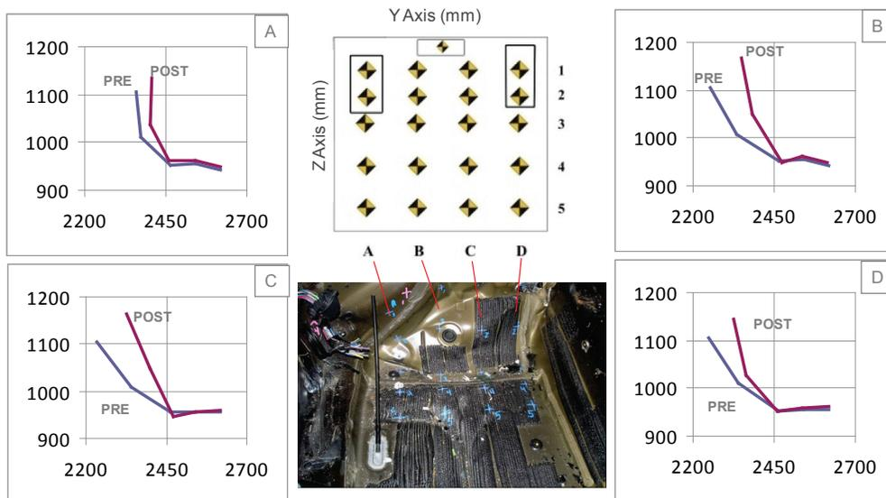
Figure 15 – Driver Side Toepan Intrusion From MDB35 Baseline (Test #090904)
