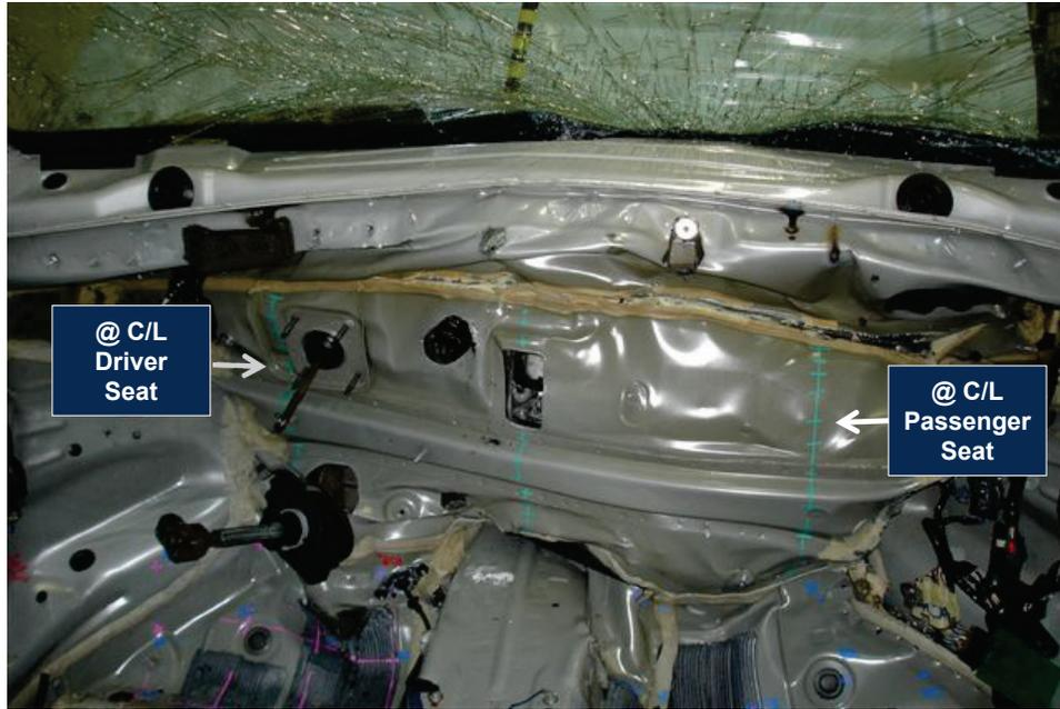
Figure 39 – Photograph of Measurement Points Used in Dimensional Analysis
