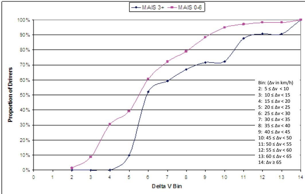
Figure 2 - Cumulative Distribution of Drivers in Pole/Tree Crashes by Delta-V
