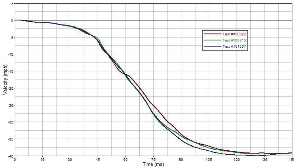
Figure 46 - Longitudinal Velocity Time History, Pole35
