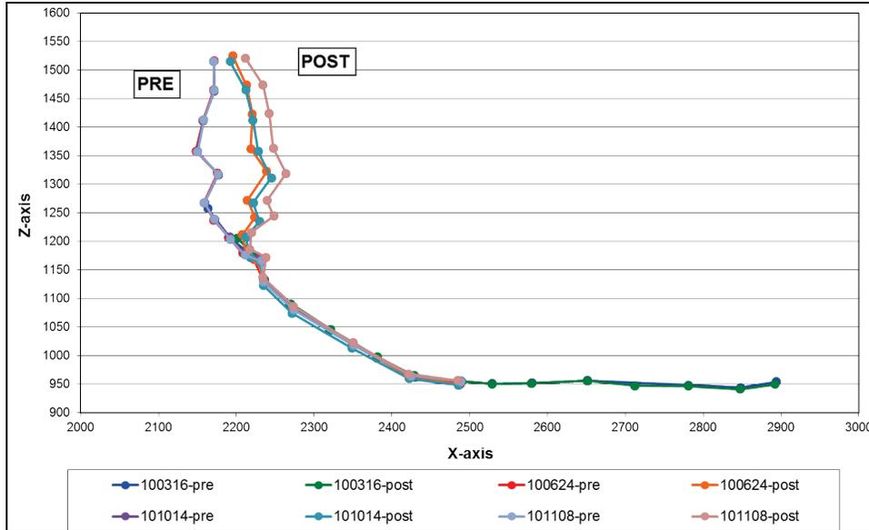
Figure 45 - Dash Panel Intrusion Profile – Passenger Side, MDB25
