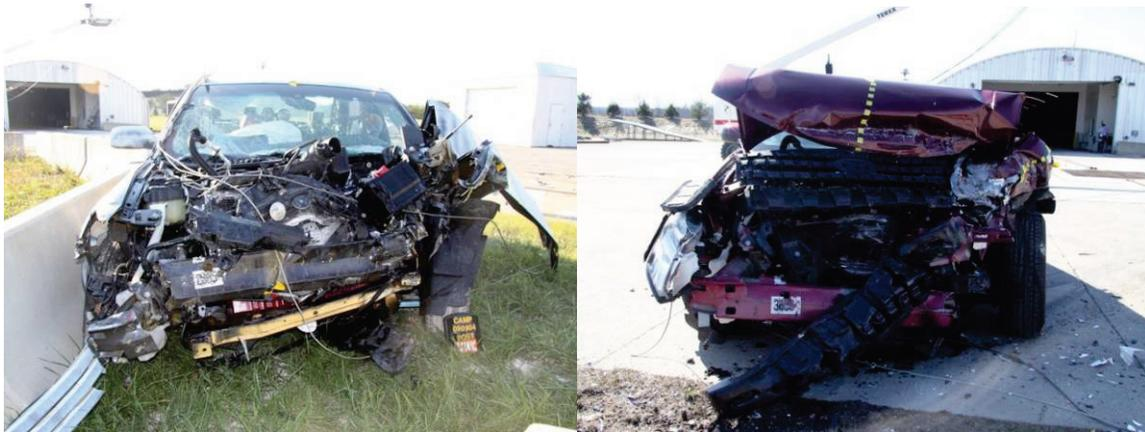
**Figure 19 - Post-Test Photographs of PVP: MDB35 Test #090904 (Left) and MDB25 Test #100316 (Right)**
