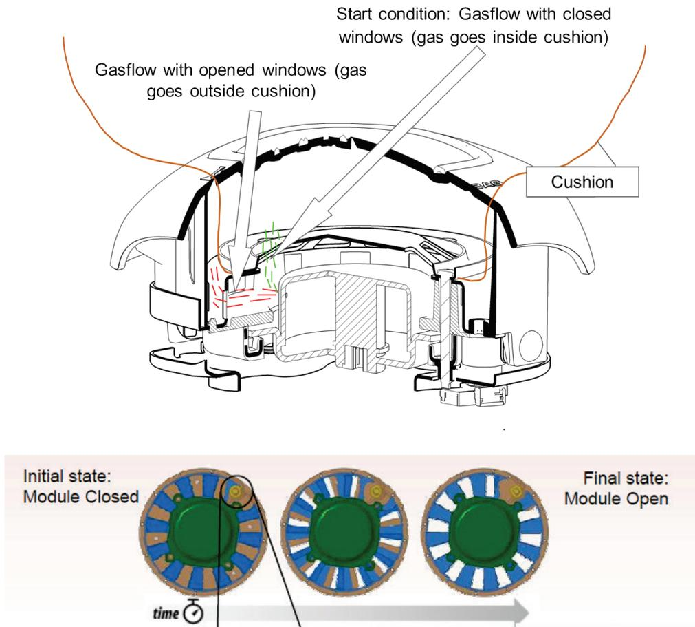
Figure 21 - Driver Air Bag Module With PVM Functionality
