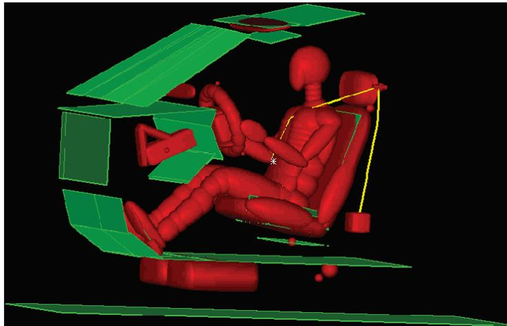
**Figure 6 - CAE Front Occupant System MADYMO Model**
