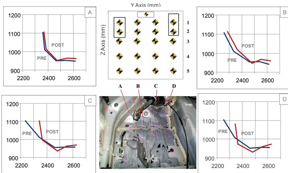
Figure 17 - Driver Side Toepan Intrusion From Pole35 Baseline (Test #090922)
