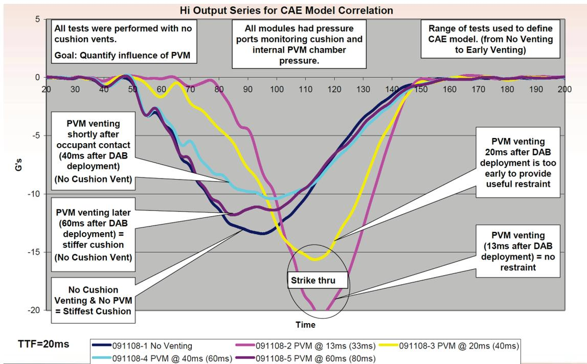
**Figure 22 - Pendulum Testing Illustrating the Effect of Various PVM Open Times on Response**
