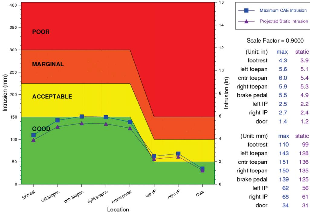
Figure 7 - Interior Compartment Intrusions for the 35 mph Centerline Pole Impact Plotted with IIHS Guidelines for Rating Occupant Compartment Intrusion (40 mph ODB)
