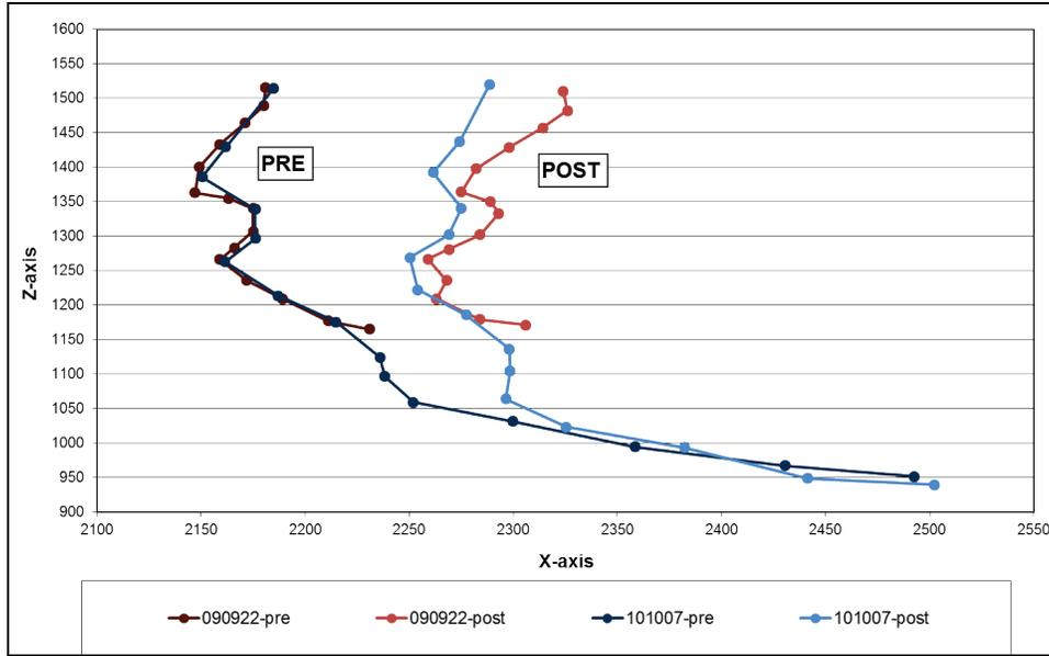
Figure 47 - Dash Panel Intrusion Profile – Driver Side, Pole35
