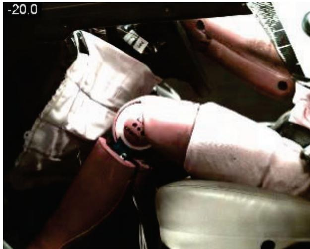
**Figure 29 - Pre-Positioned ARS KAB, Prior to Inflation (HIII 50M)**
