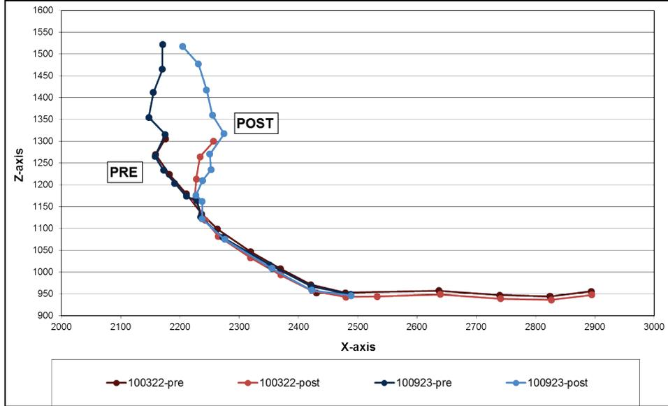
Figure 51 - Dash Panel Intrusion Profile – Passenger Side, Pole25
