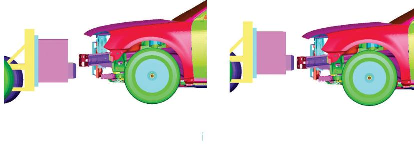
**Figure 11 - MDB and Target Vehicle Bumper Alignment**
