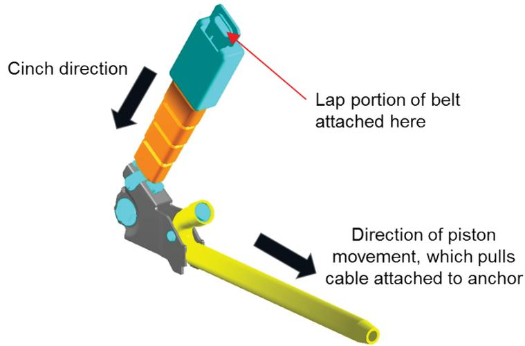
**Figure 32 - Lap Anchor Pretensioner**
