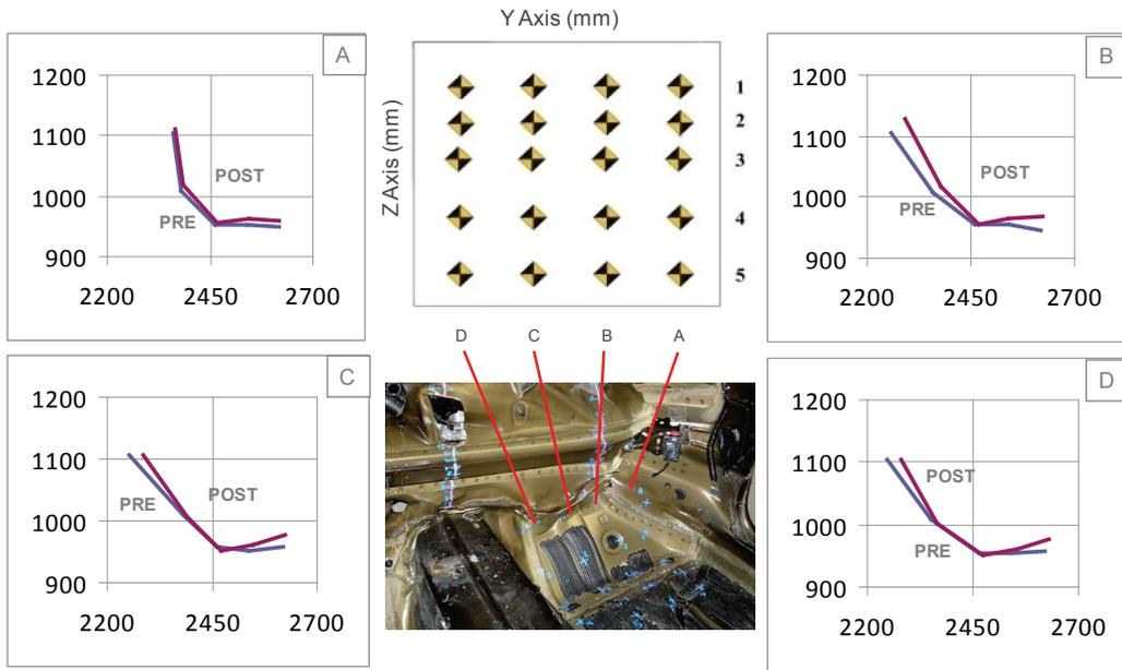
Figure 16 – Passenger Side Toepan Intrusion From MDB35 Baseline (Test #090904)
