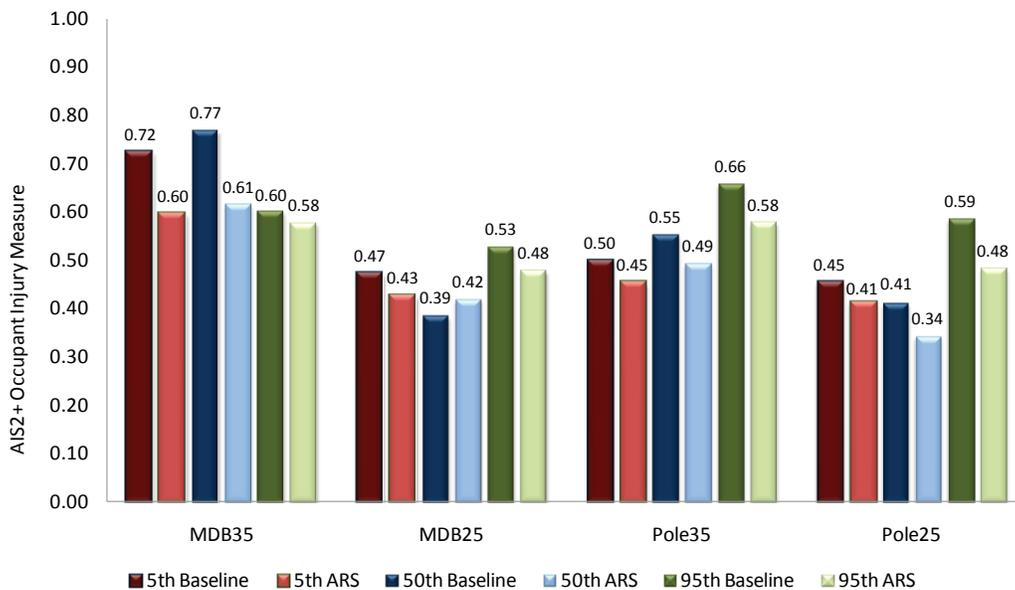
**Figure ES2 – Combined AIS2+ Occupant Injury Measure, PVP Versus ARS, All Drivers**
