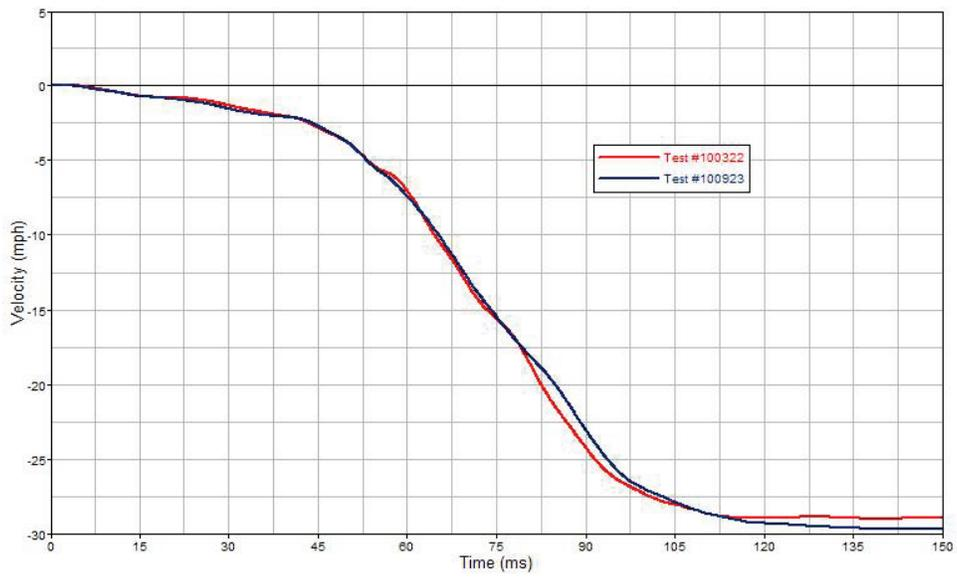
Figure 49 - Longitudinal Velocity Time History, Pole25
