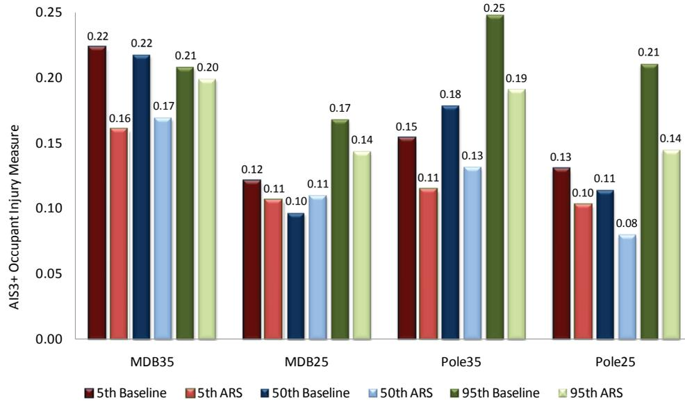
**Figure ES1 – Combined AIS3+ Occupant Injury Measure, PVP Versus ARS, All Drivers**
