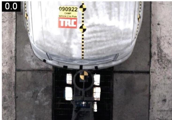
Figure 14 - Vehicle-to-Pole Test Configuration
