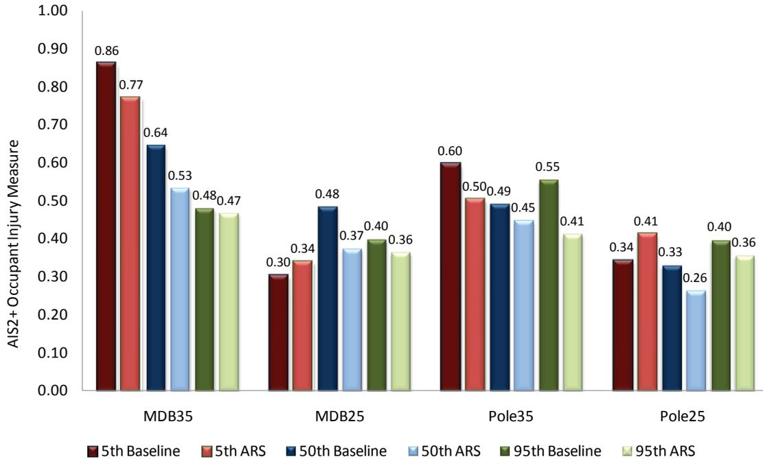
Figure 72 - OIM-AIS2+, PVP Versus ARS, All Front-Outboard Passengers
