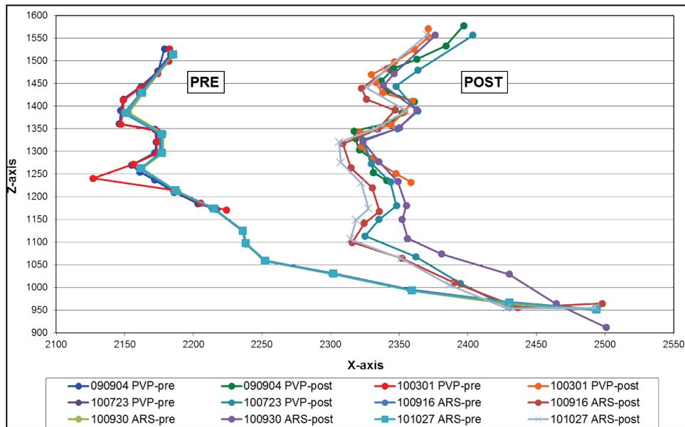
Figure 40 - Dash Panel Intrusion Profile – Driver Side, MDB35
