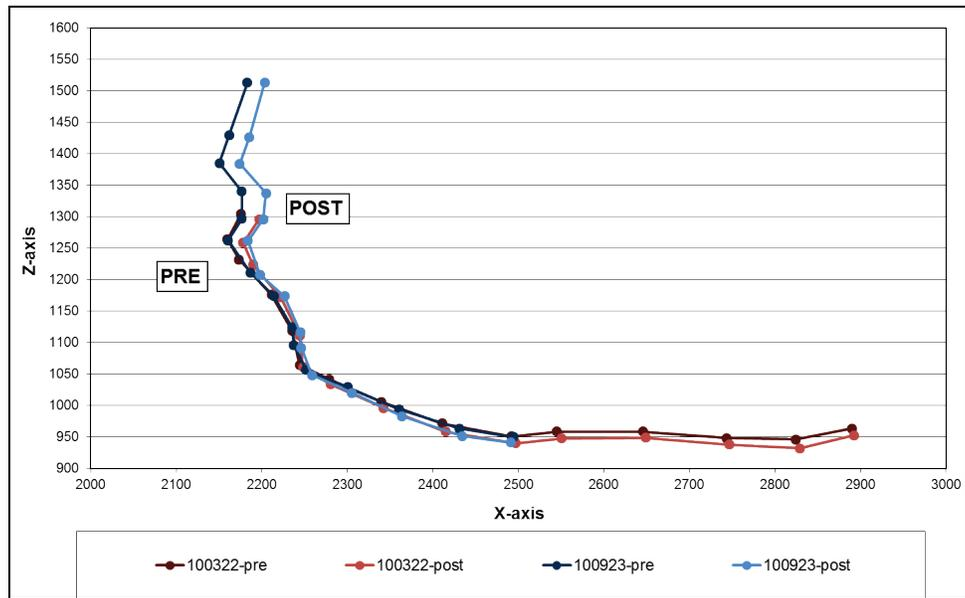
Figure 50 - Dash Panel Intrusion Profile – Driver Side, Pole25
