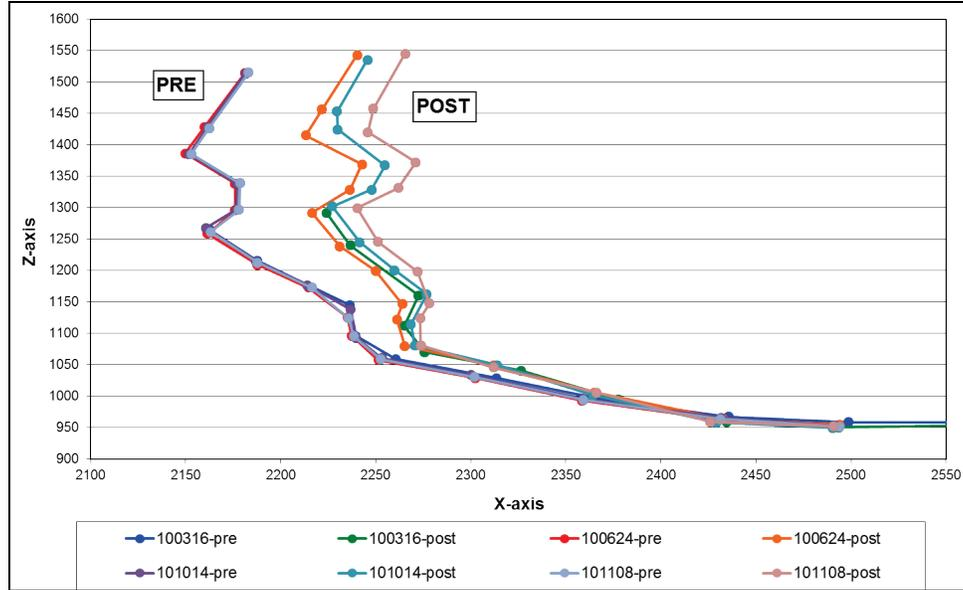
Figure 44 - Dash Panel Intrusion Profile – Driver Side, MDB25
