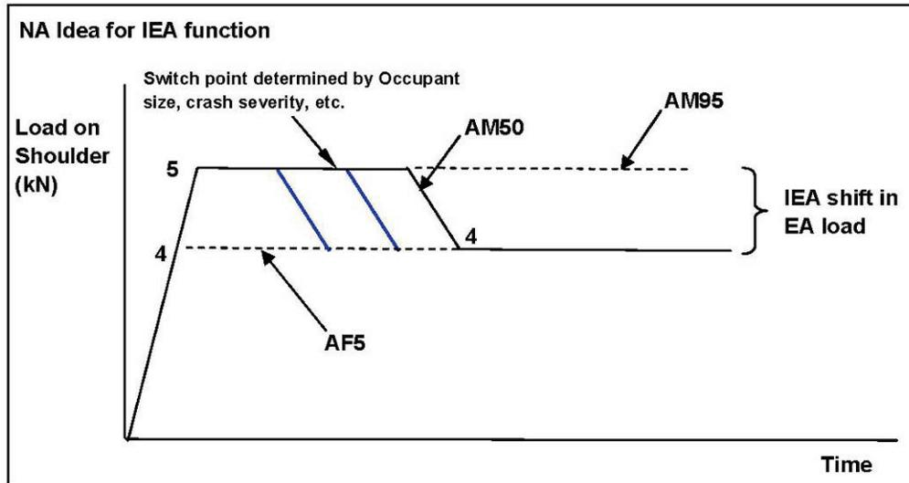
**Figure 31 - Load Curve Scenarios for the Dual-Stage, Adaptive Load Limiter Device**
