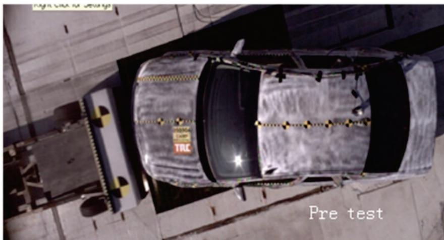
**Figure 13 - MDB-to-Vehicle Test Configuration**
