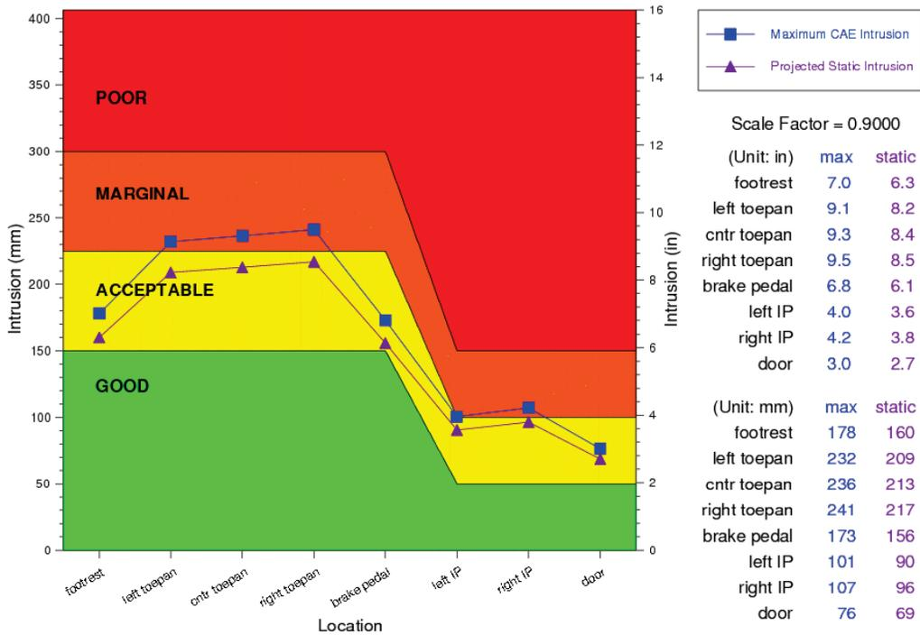
Figure 8 - Interior Compartment Intrusions for the 40 mph Centerline Pole Impact Plotted With IIHS Guidelines for Rating Occupant Compartment Intrusion (40 mph ODB)
