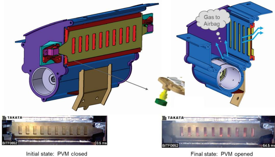
**Figure 24 - Passenger Air Bag Module With PVM Functionality**
