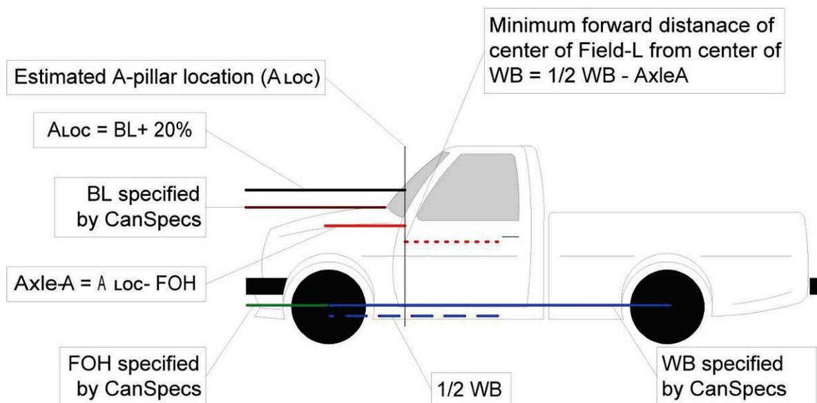
**Figure 9: Estimating the A-pillar Location**
