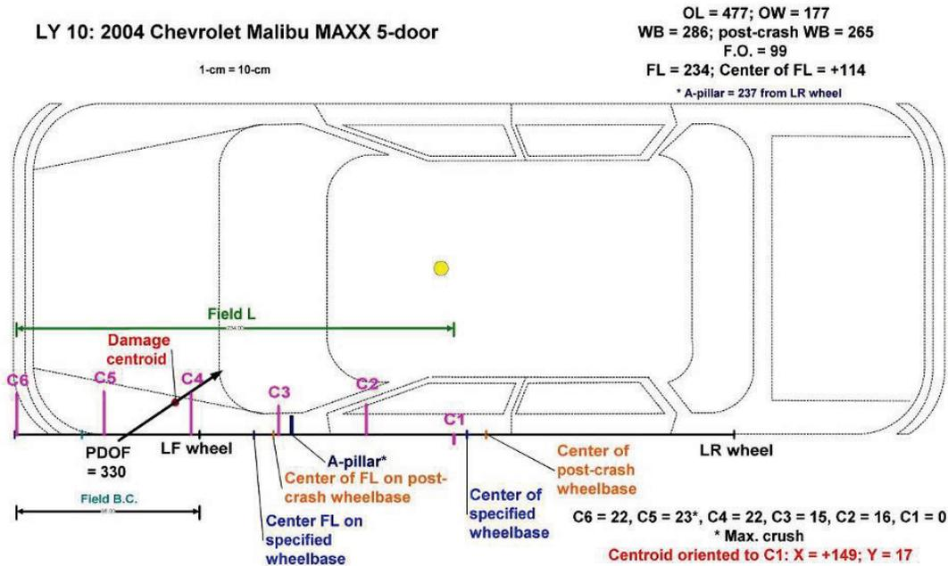
**Figure 7: Oblique 'LY' Small-Overlap Impact**
