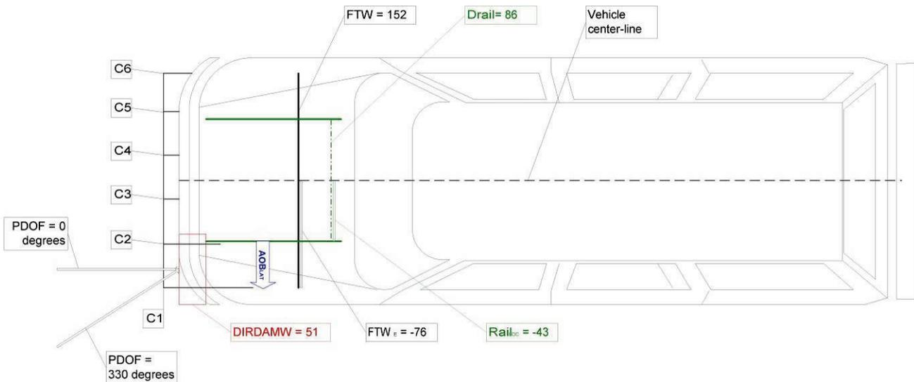
Figure 6: Crush Criteria Applied to Generic Compact SUV Model
