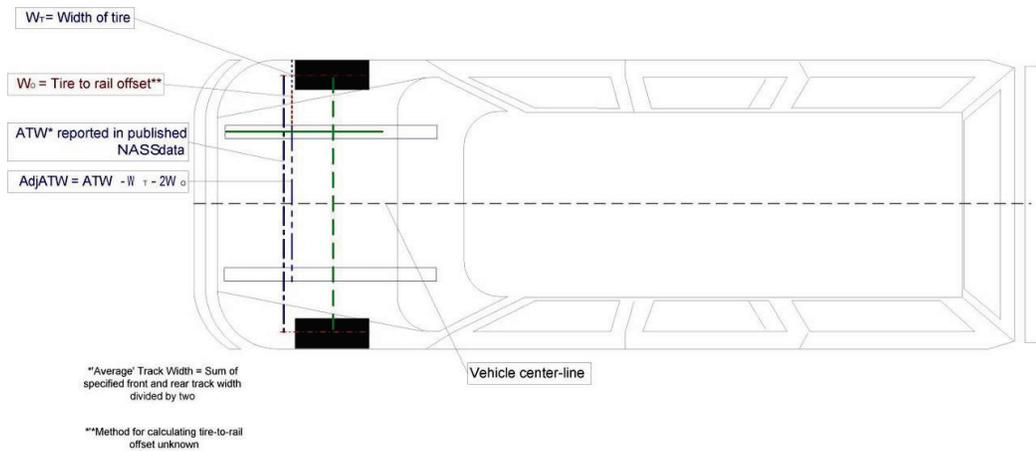
**Figure 3: “Adjusted ATW” Definition of SOI**
