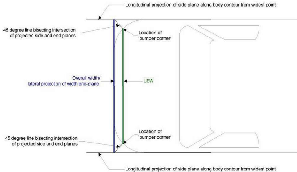
**Figure 4: Determination of Undeformed End Width (UEW).**
