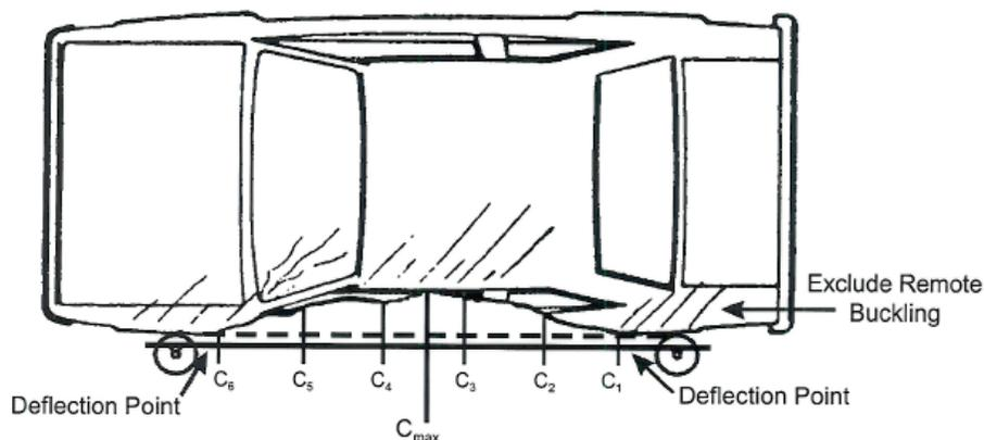
**Figure 8: Field Protocol for Documenting a Crush Profile for a Side Impact**
