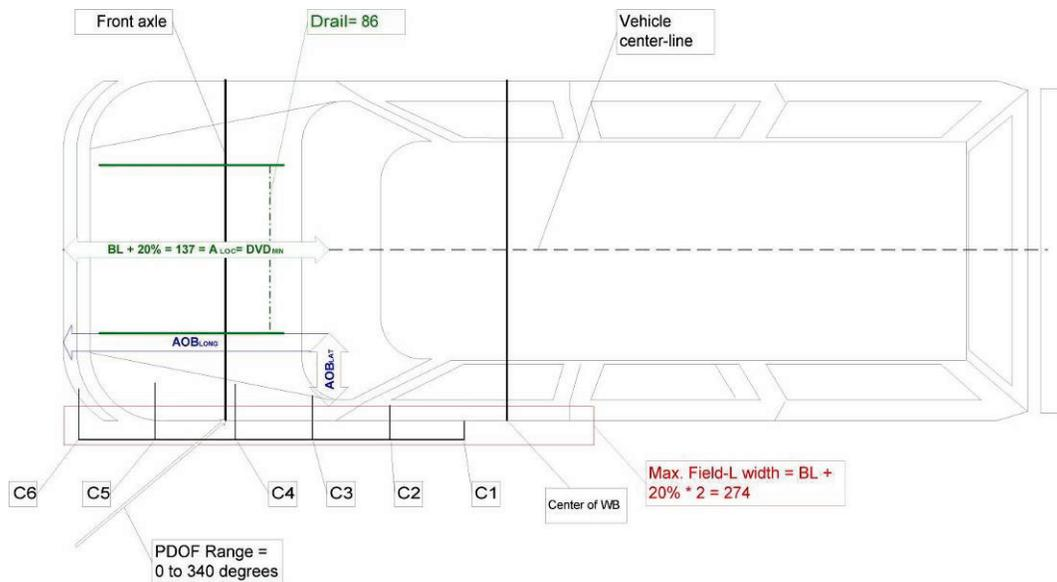
**Figure 10: Locating the Center of the Crush Profile Relative to the Area Outboard of the Longitudinal Members**
