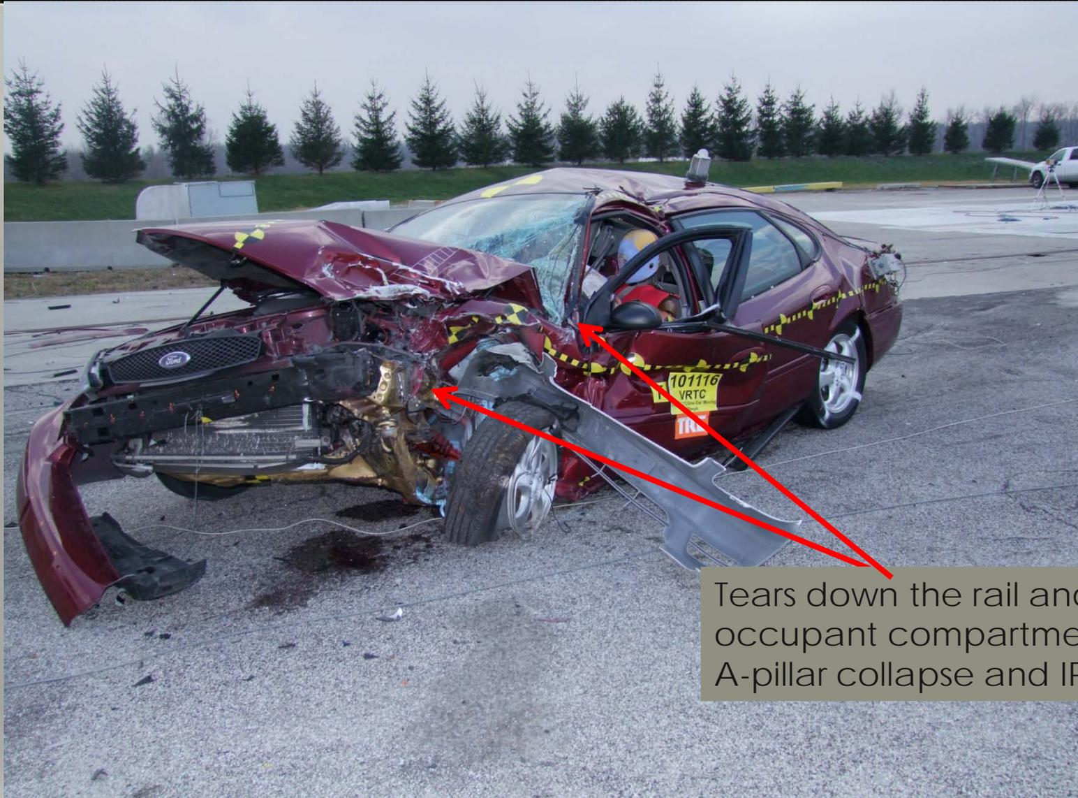
Tears down the rail and engages occupant compartment causes A-pillar collapse and IP intrusion
