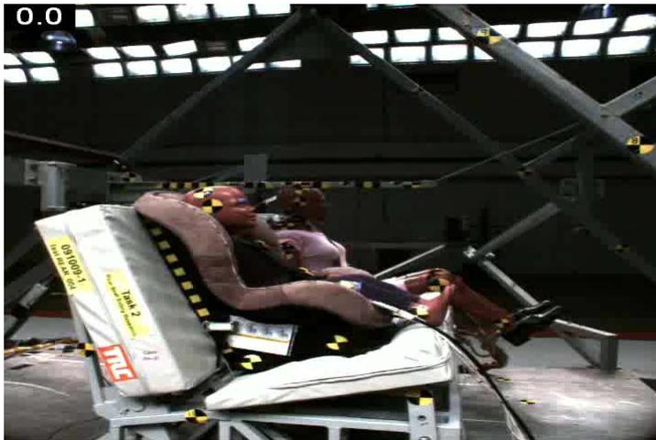
Test # 4: Thin, Wedge, Soft, 16°; Head X = 352 mm from normally seated
