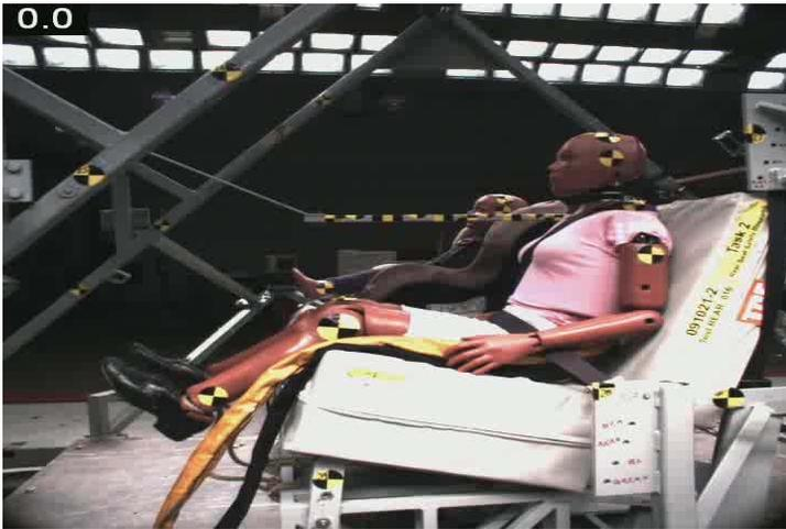
Test # 16: Thick, Flat, Hard, 16°; Head X = 472 mm from normally seated
