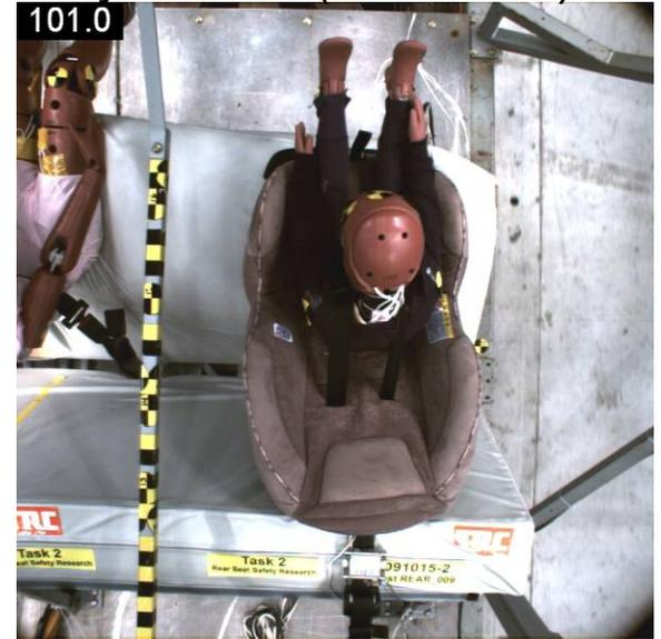
Test # 4: Thin, Wedge, Soft, 16°; Head X = 352 mm from normally seated
