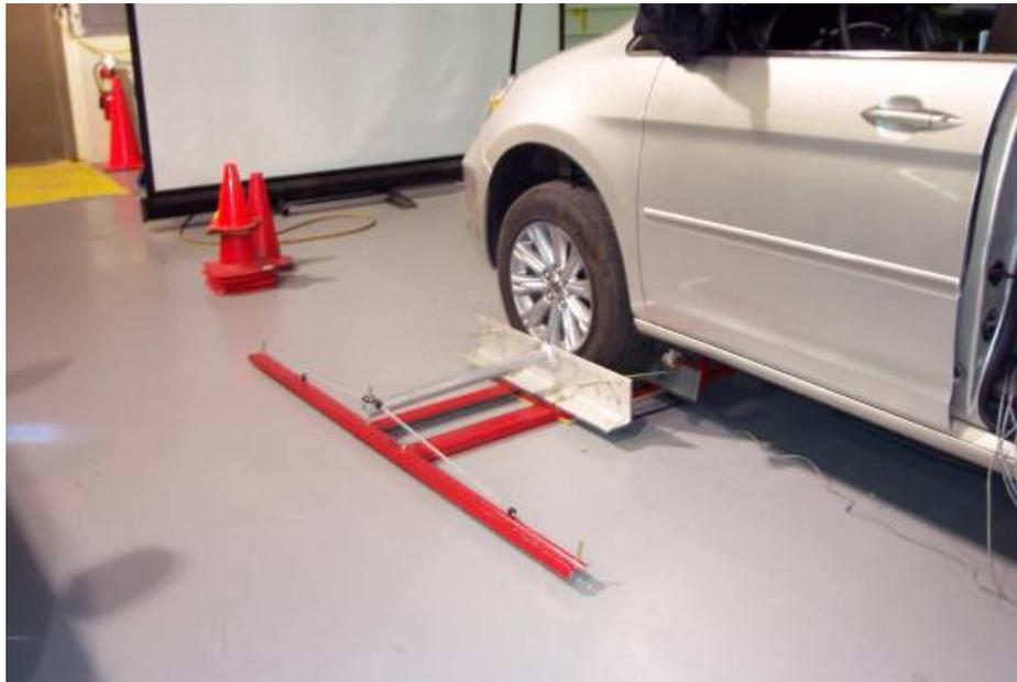
Figure 7. Steering Apparatus Installed on Front Tire
