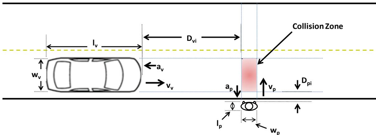
**Figure 77. Vehicle-Going-Straight/Pedestrian-Crossing-Road Pre-Crash Scenario Configuration**
