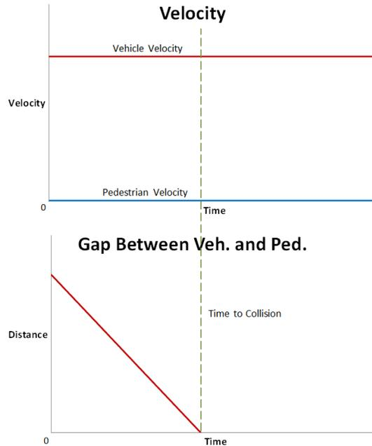
**Figure 70. Timeline of Vehicle-Going-Straight/Pedestrian-in-Road Pre-Crash Scenario**
