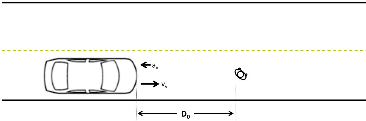
**Figure 69. Vehicle-Going-Straight/Pedestrian in Road Pre-Crash Scenario Configuration**
