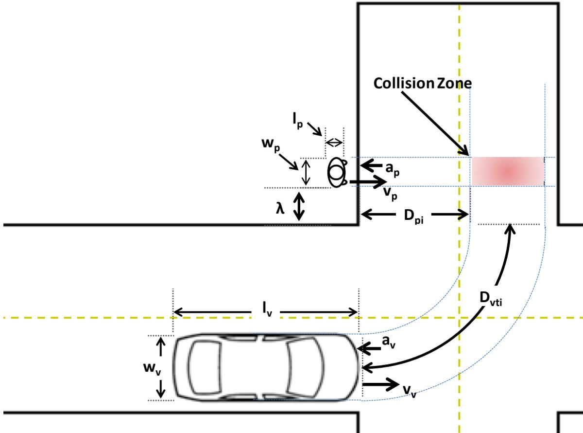
**Figure 81. Vehicle-Turning-Left/Pedestrian-Crossing-Road Pre-Crash Scenario Configuration**
