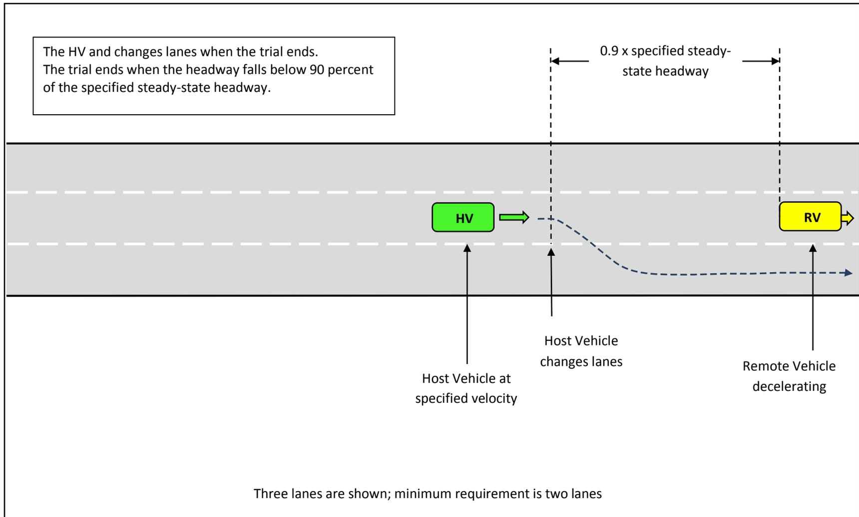
**Figure A-7 - EEBL-3 Test Course Graphic, End of Trial (not to scale)**
