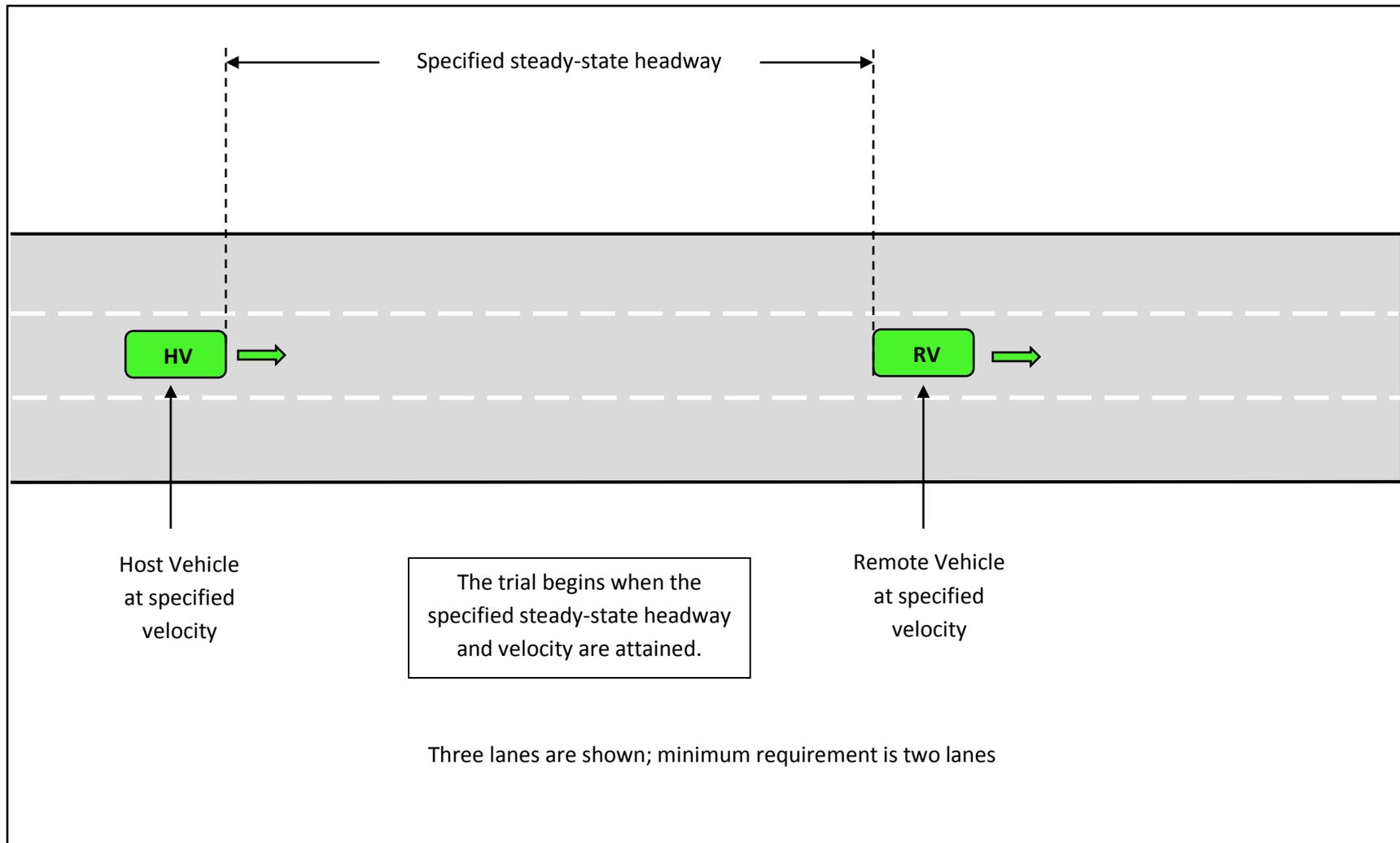
Figure A-16 - EEBL-8 Test Course Graphic, Initial Conditions (not to scale)
