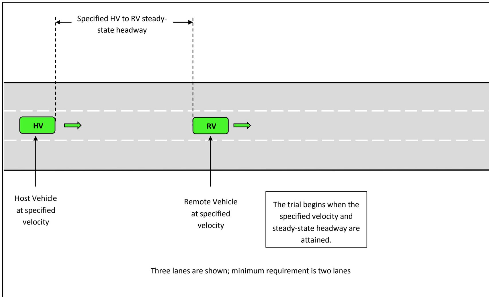
Figure A-6 - EEBL-3 Test Course Graphic, Initial Conditions (not to scale)
