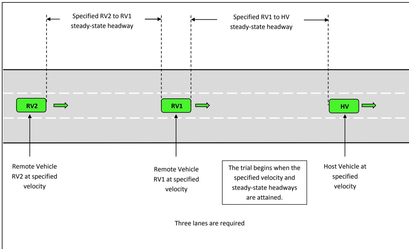
**Figure A-4 - EEBL-2 Test Course Graphic, Initial Conditions (not to scale)**
