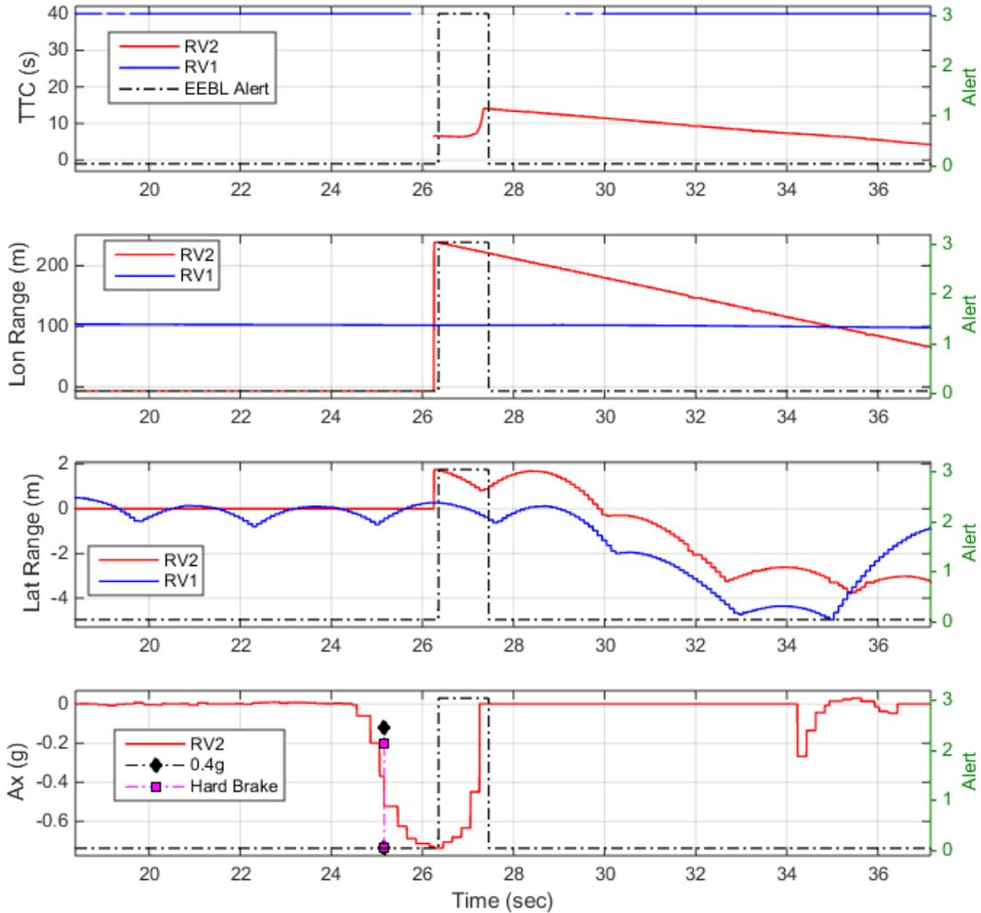
**Figure 14: Example EEBL-5 Results - HV Drives Into EEBL Alert Range – Test 1267**
