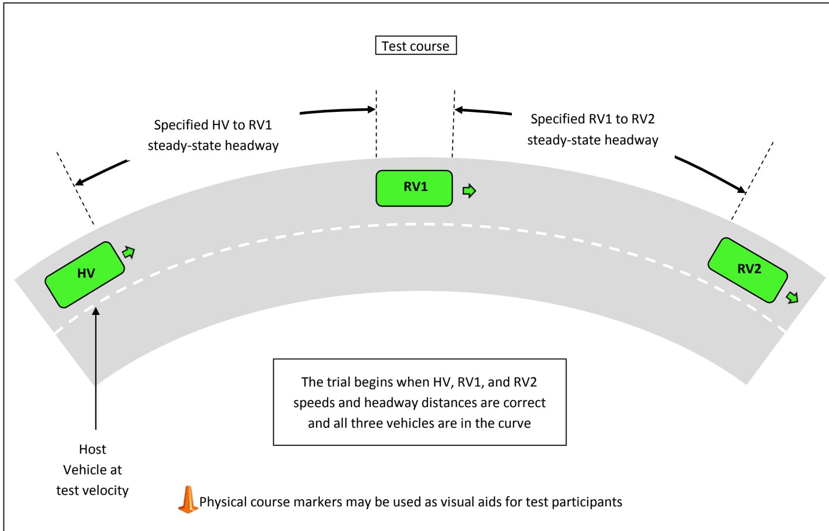
**Figure A-10 - EEBL-5 Test Course Graphic, Initial Conditions (not to scale)**
