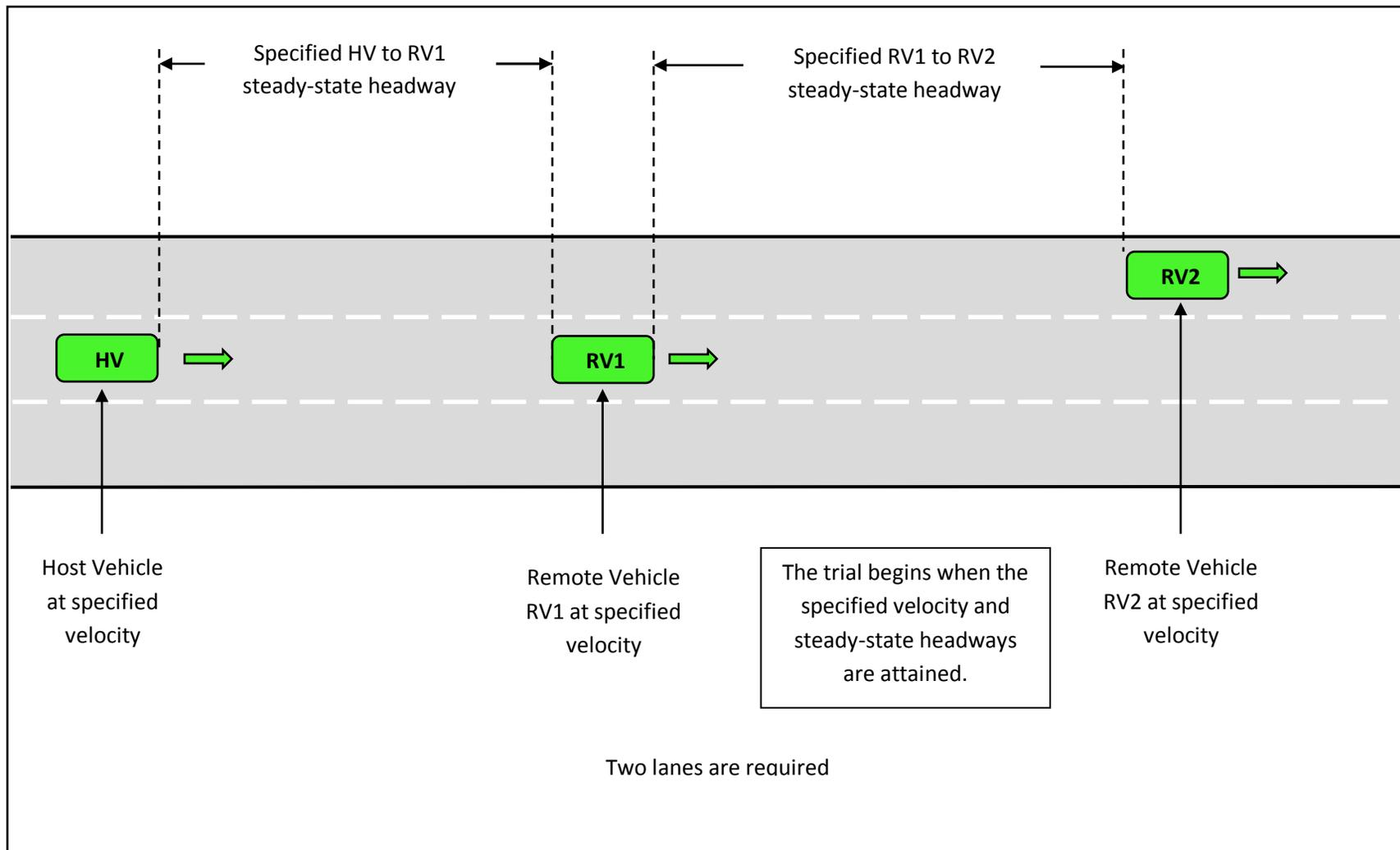
Figure A-8 - EEBL-4 Test Course Graphic, Initial Conditions (not to scale)
