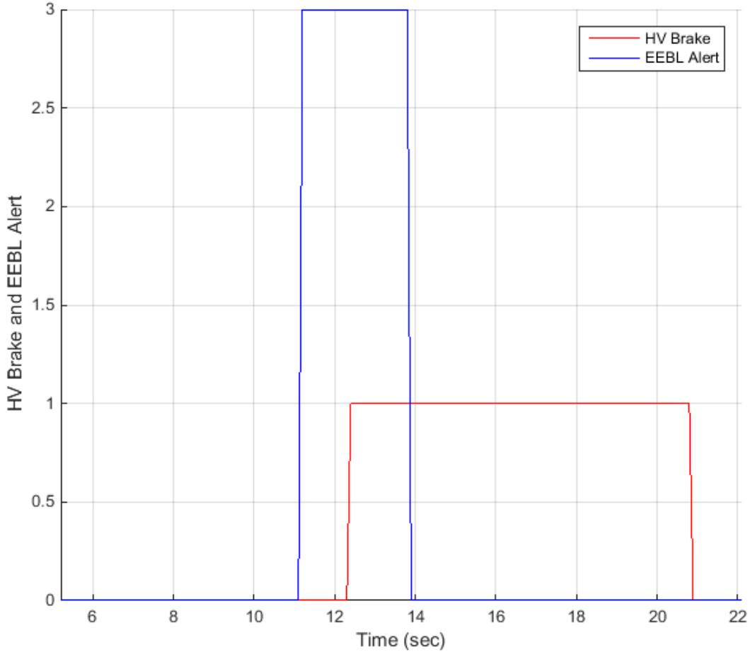
**Figure 20: Example HV Brake and EEBL Alert Traces for an EEBL-7 Test**
