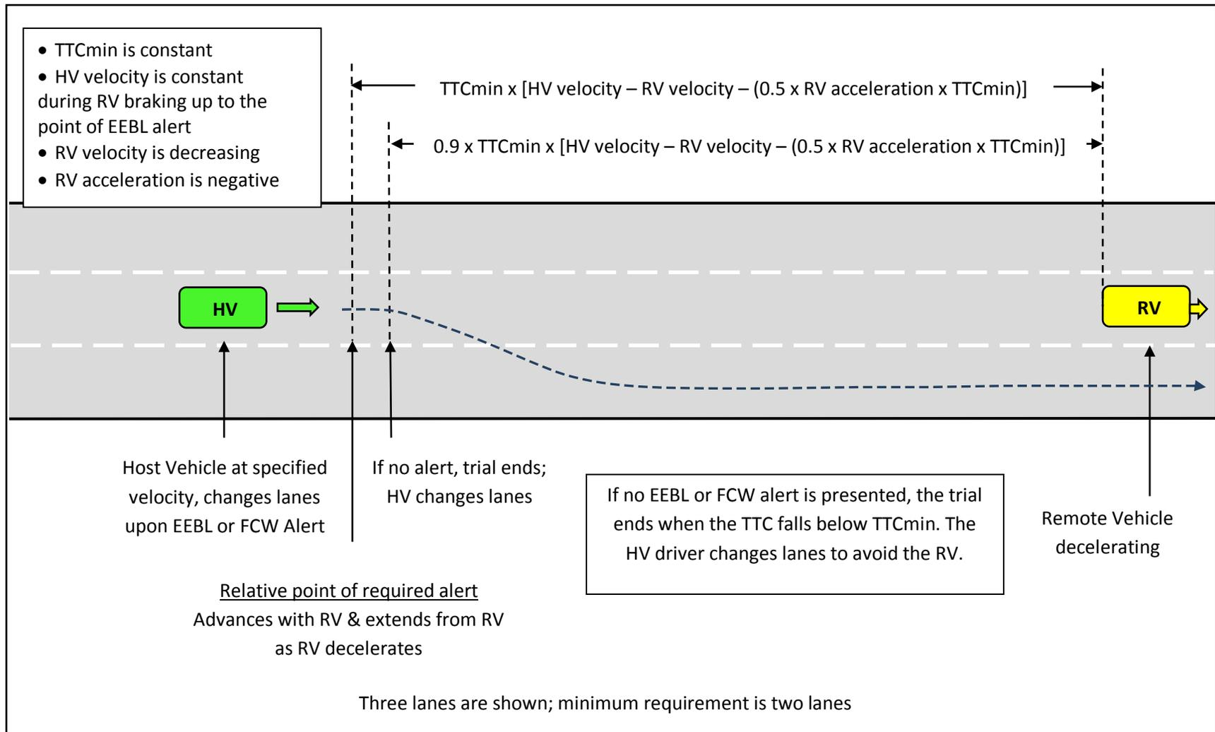
**Figure A-17 - EEBL-8 Test Course Graphic, Test Procedure End of Trial (not to scale)**
