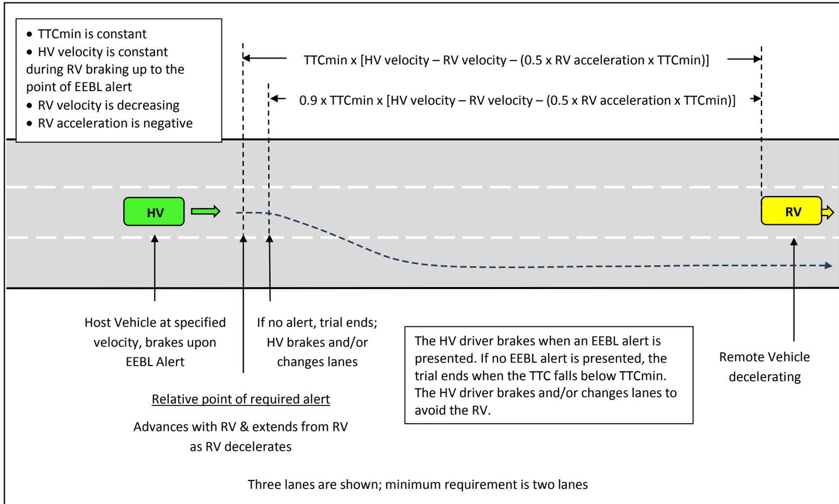
**Figure A-15 - EEBL-7 Test Course Graphic, Test Procedure End of Trial (not to scale)**
