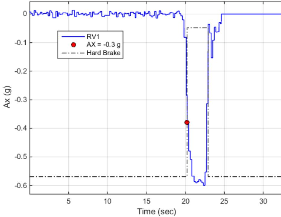
**Figure 5: Example Mack Hard Brake Deceleration Threshold =  $0.3\text{ g}$  - Test 1720**
