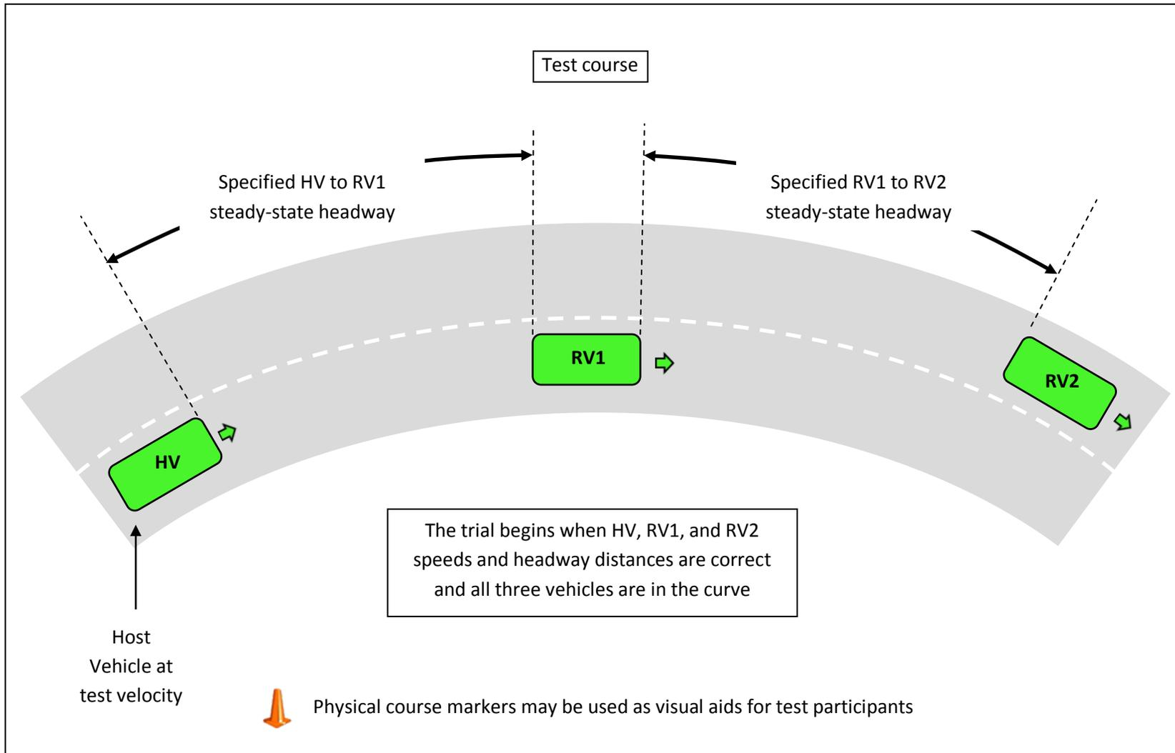
Figure A-12 - EEBL-6 Test Course Graphic, Initial Conditions (not to scale)
