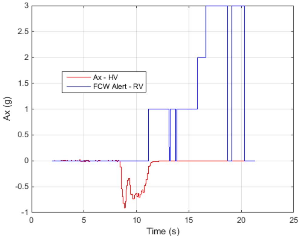
**Figure 11: HV (Blue Cascadia) Deceleration and RV (Red Cascadia) FCW Alert - Example EEBL 2 Results – Test 1540**
