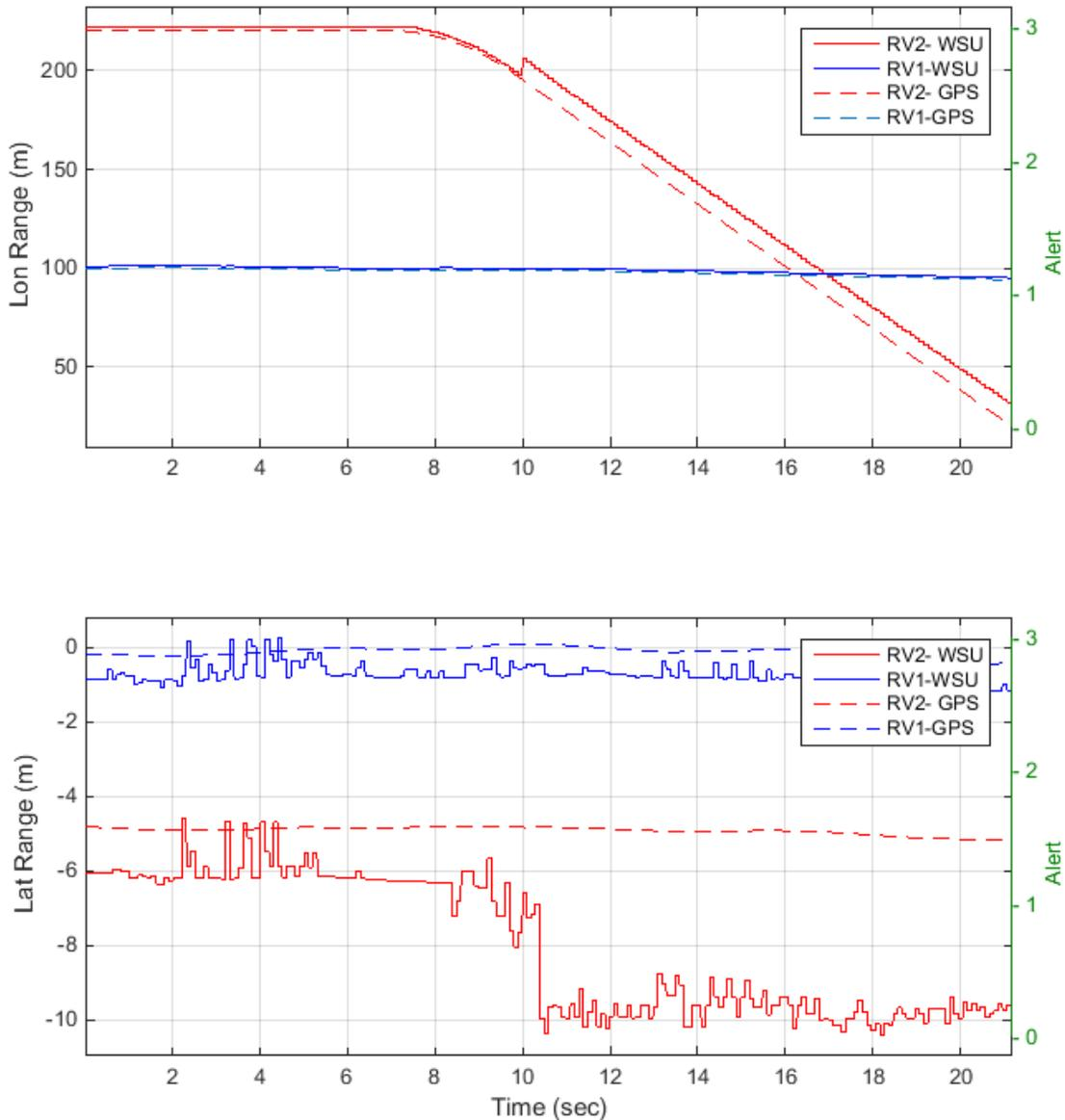
**Figure 13: Example EEBL 4 Results – No EEBL Alert, Test 1713, RV2 = Mack With 40’ Shipping Container**
