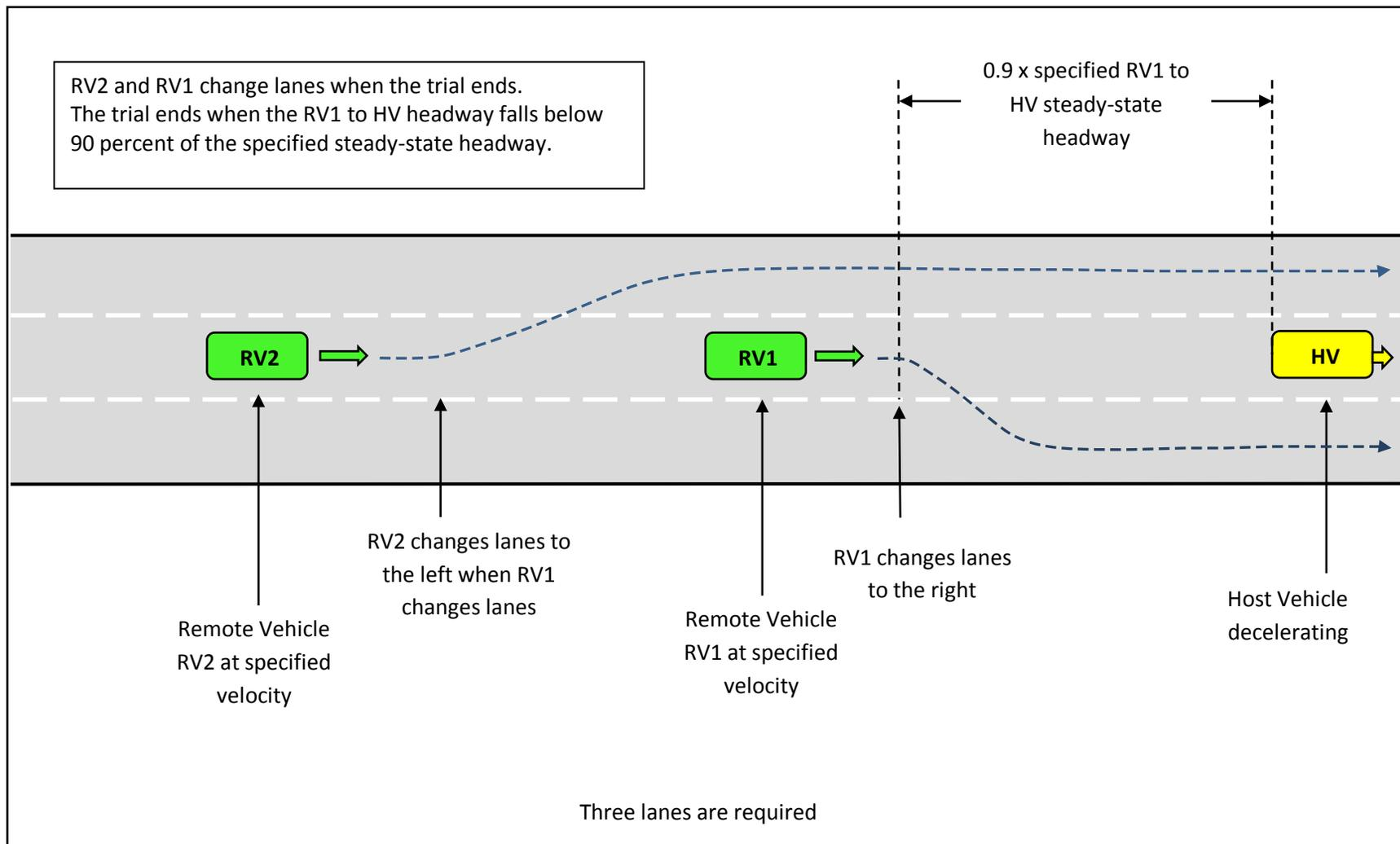
**Figure A-5 - EEBL-2 Test Course Graphic, End of Trial (not to scale)**
