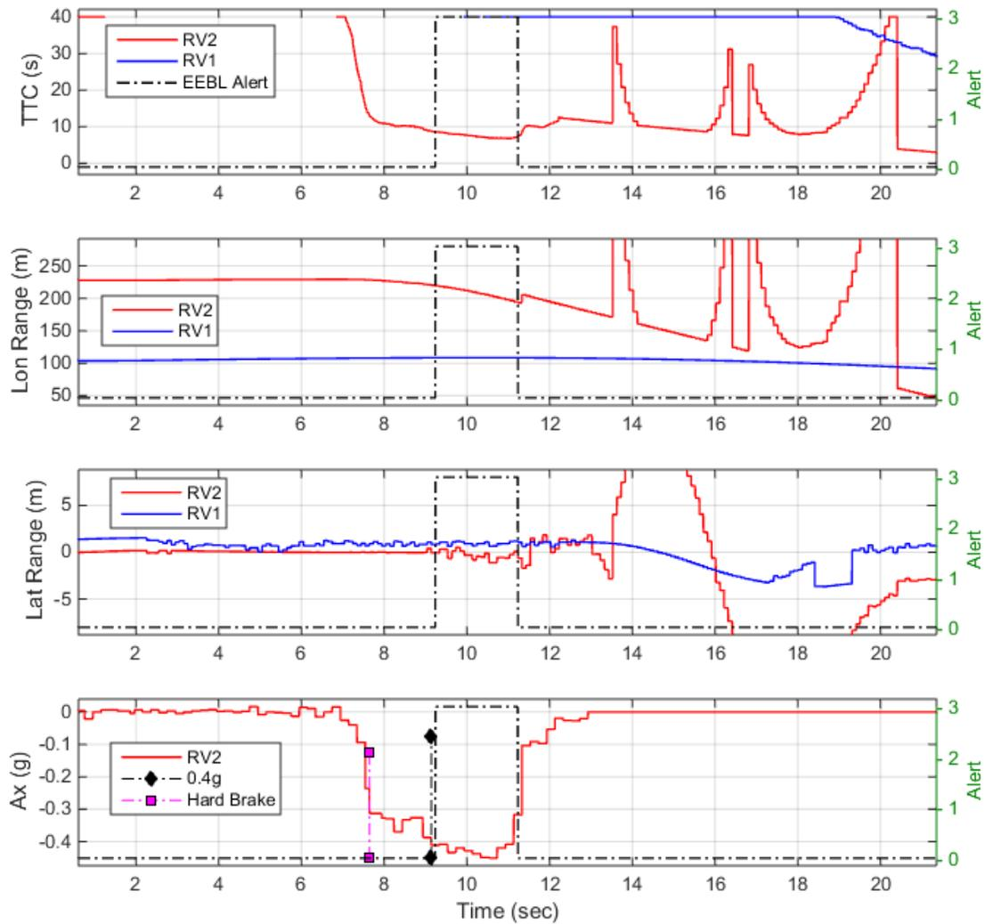
**Figure 9: EEBL Alert Shortly After 0.4 g Braking Level but Delayed From Hard Brake Event Flag – Test 1687**
