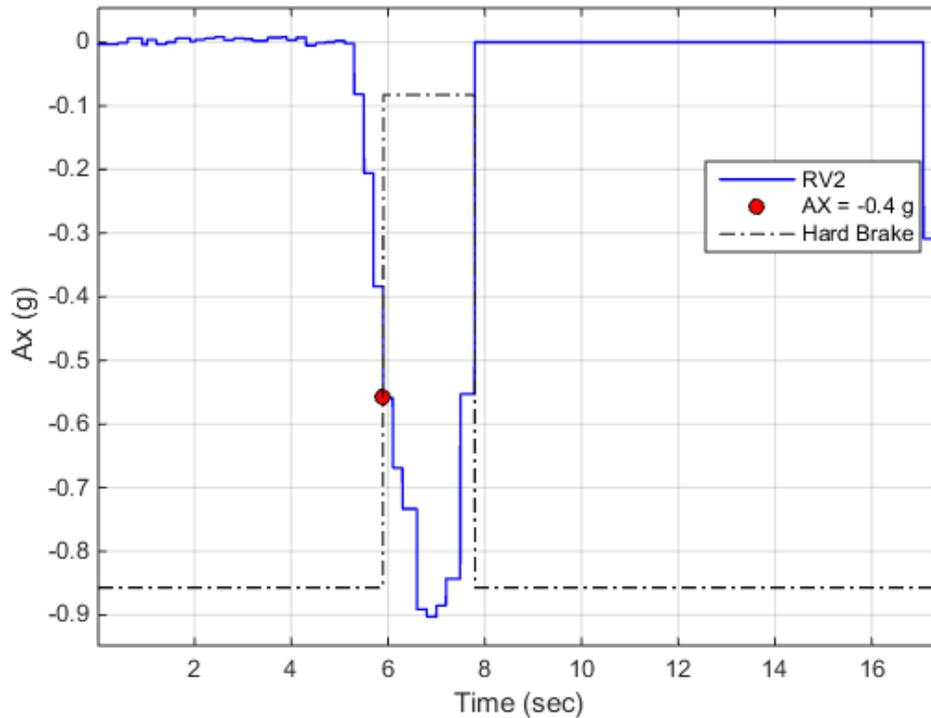
**Figure 6: Example Honda Odyssey Hard Brake Deceleration Threshold = 0.4 g - Test 1251**
