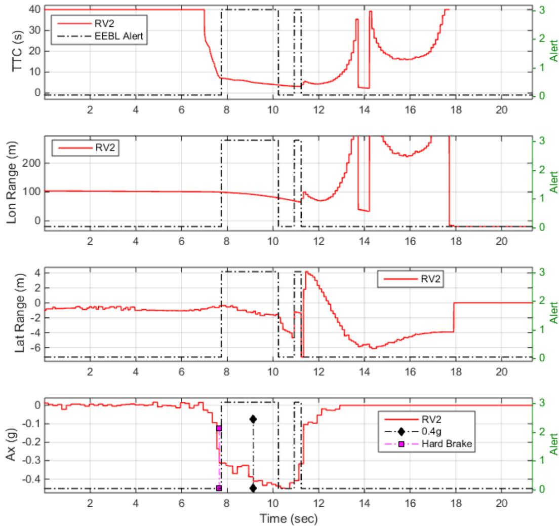
**Figure 10: EEBL Alert Shortly After Hard Brake Event Flag (Blue Cascadia Acting as HV) – Test 1687**
