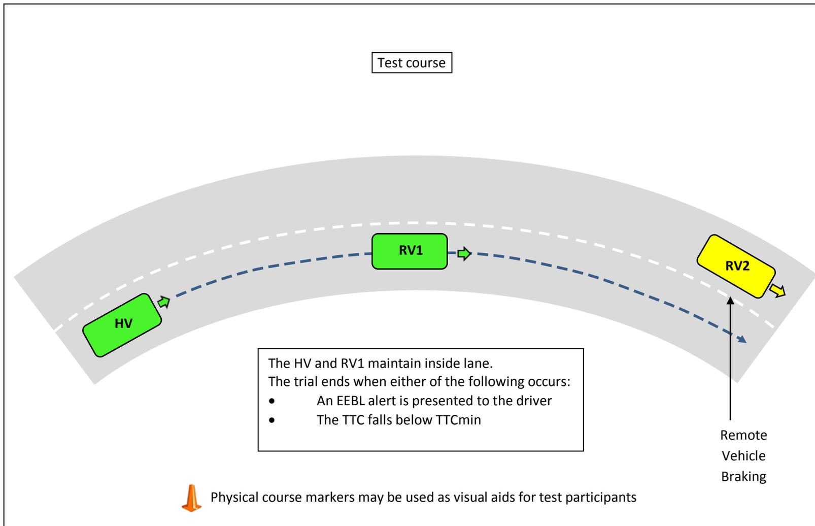
**Figure A-13 - EEBL-6 Test Course Graphic, End of Trial (not to scale)**
