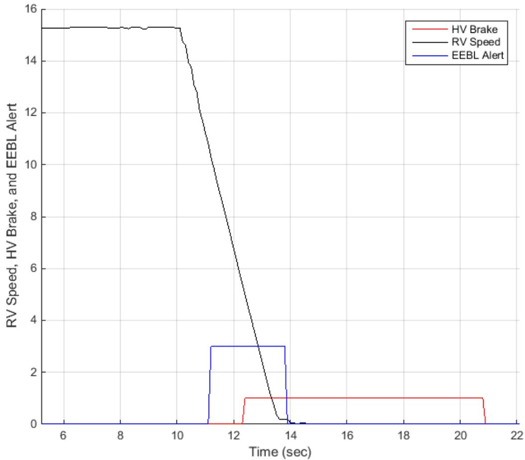
**Figure 21: Example RV Speed, HV Brake, and EEBL Alert Traces for an EEBL-7 Test**
