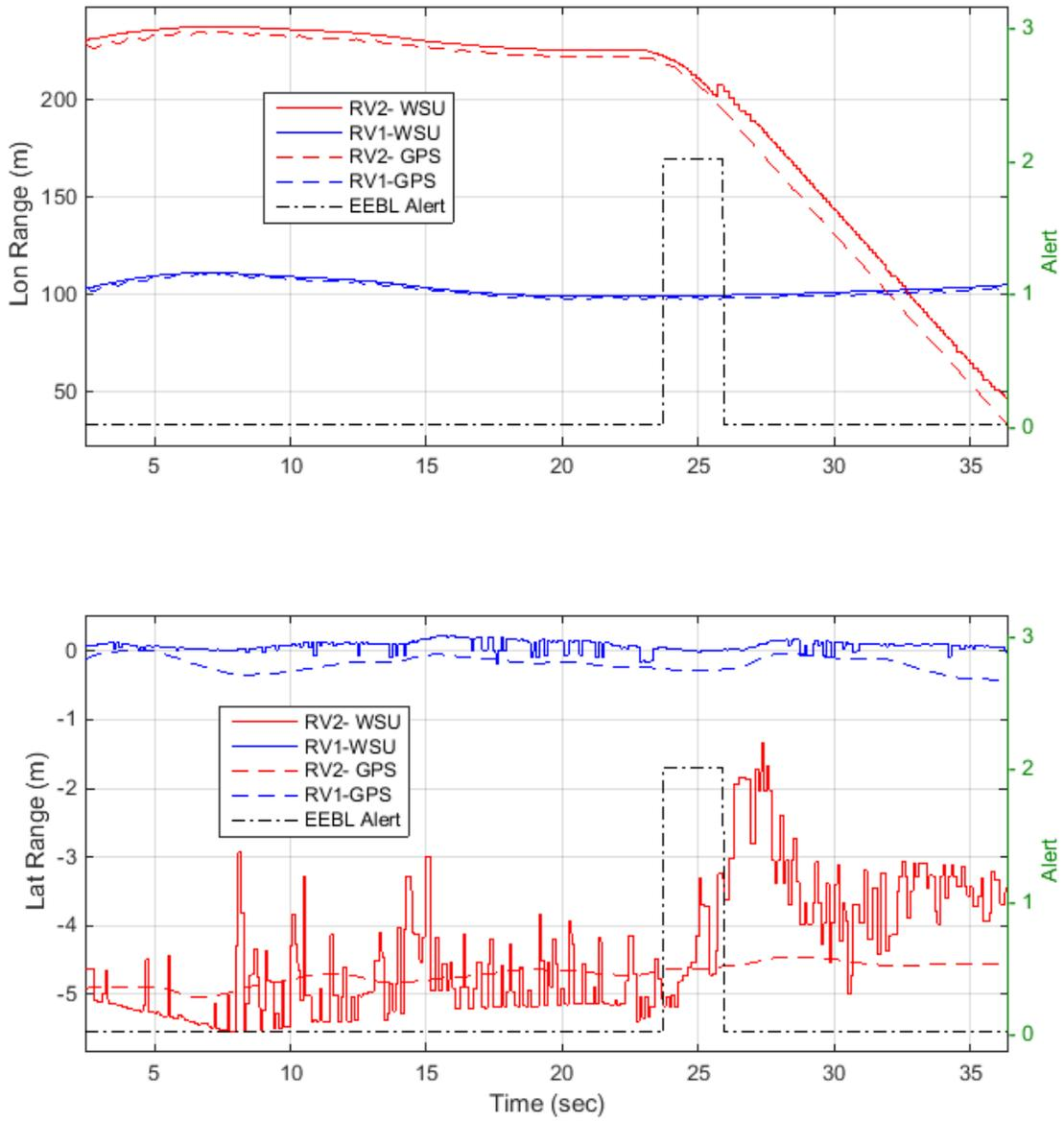
**Figure 12: Example EEBL 4 Results –EEBL Alert, Test 1729, RV2 = Mack With 28’ Doubles**
