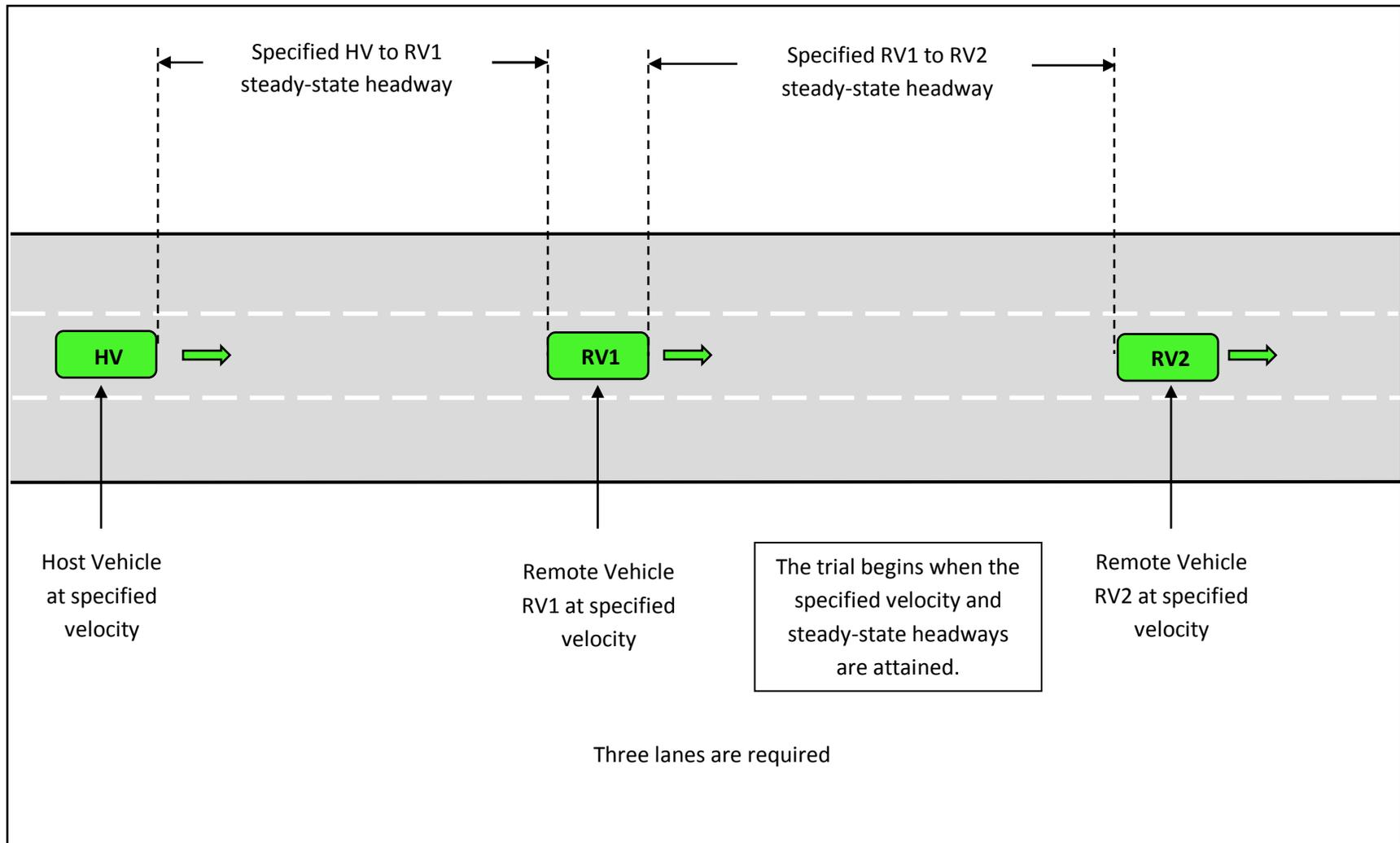
Figure A-2 - EEBL-1 Test Course Graphic, Initial Conditions (not to scale)
