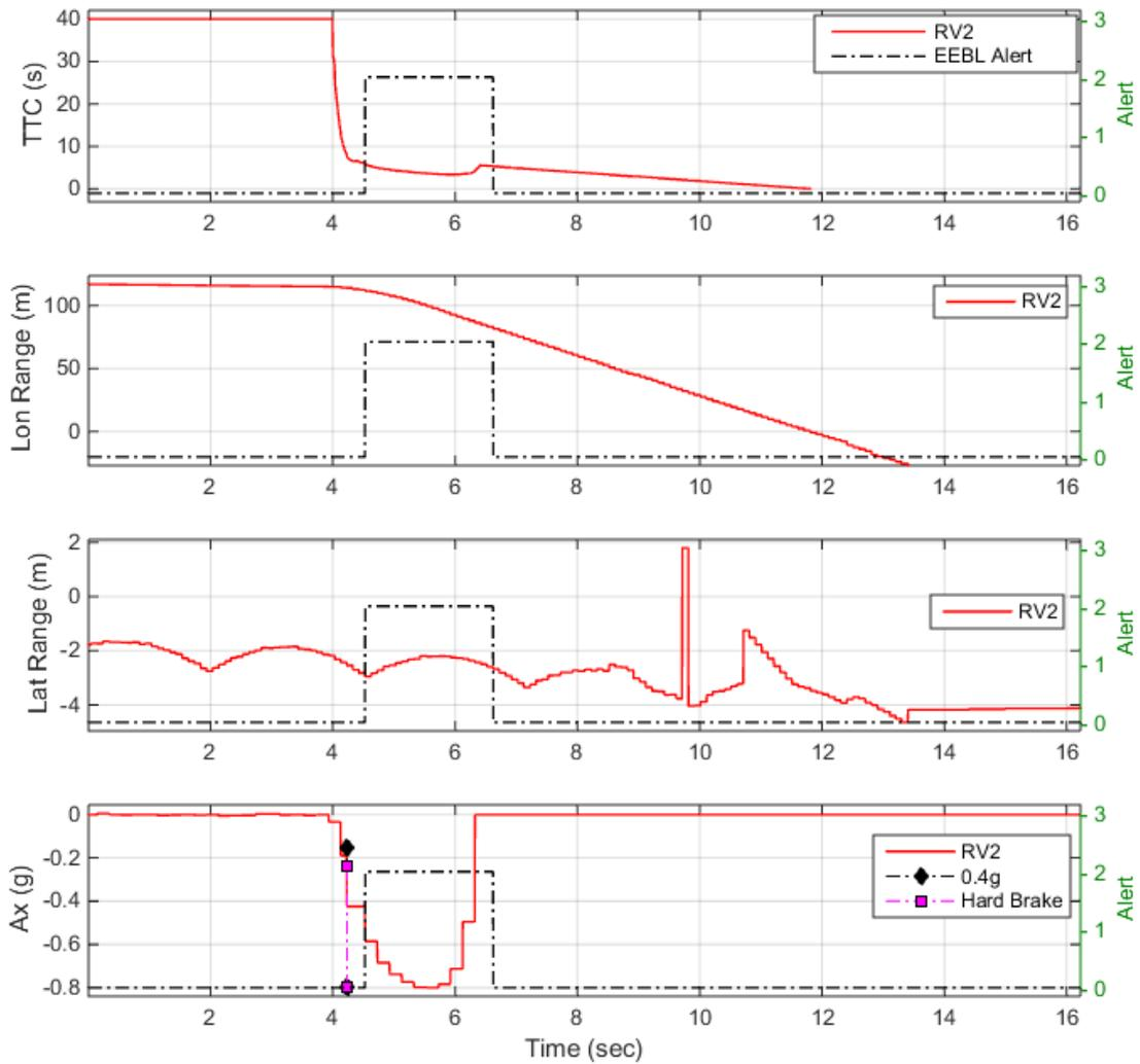
**Figure 17: Example EEBL-6 Results – RV1 Acting as HV Inside EEBL Alert Range – Test 1256**
