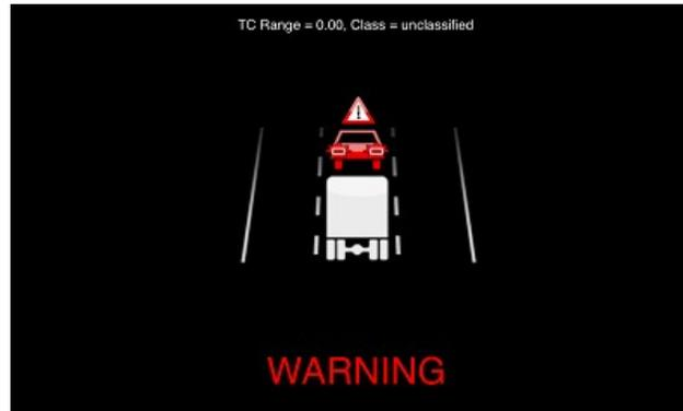
**Figure 3: EEBL Warning Level 3 Alert [2]**
