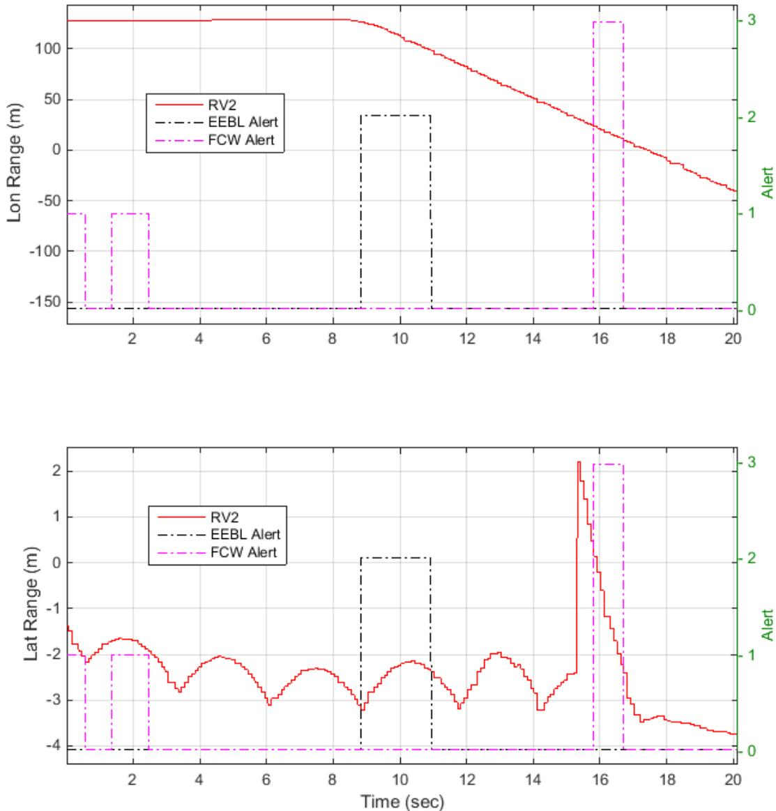
**Figure 19: Example False FCW Alert After EEBL Alert – Test 1255 (RV1 as HV)**
