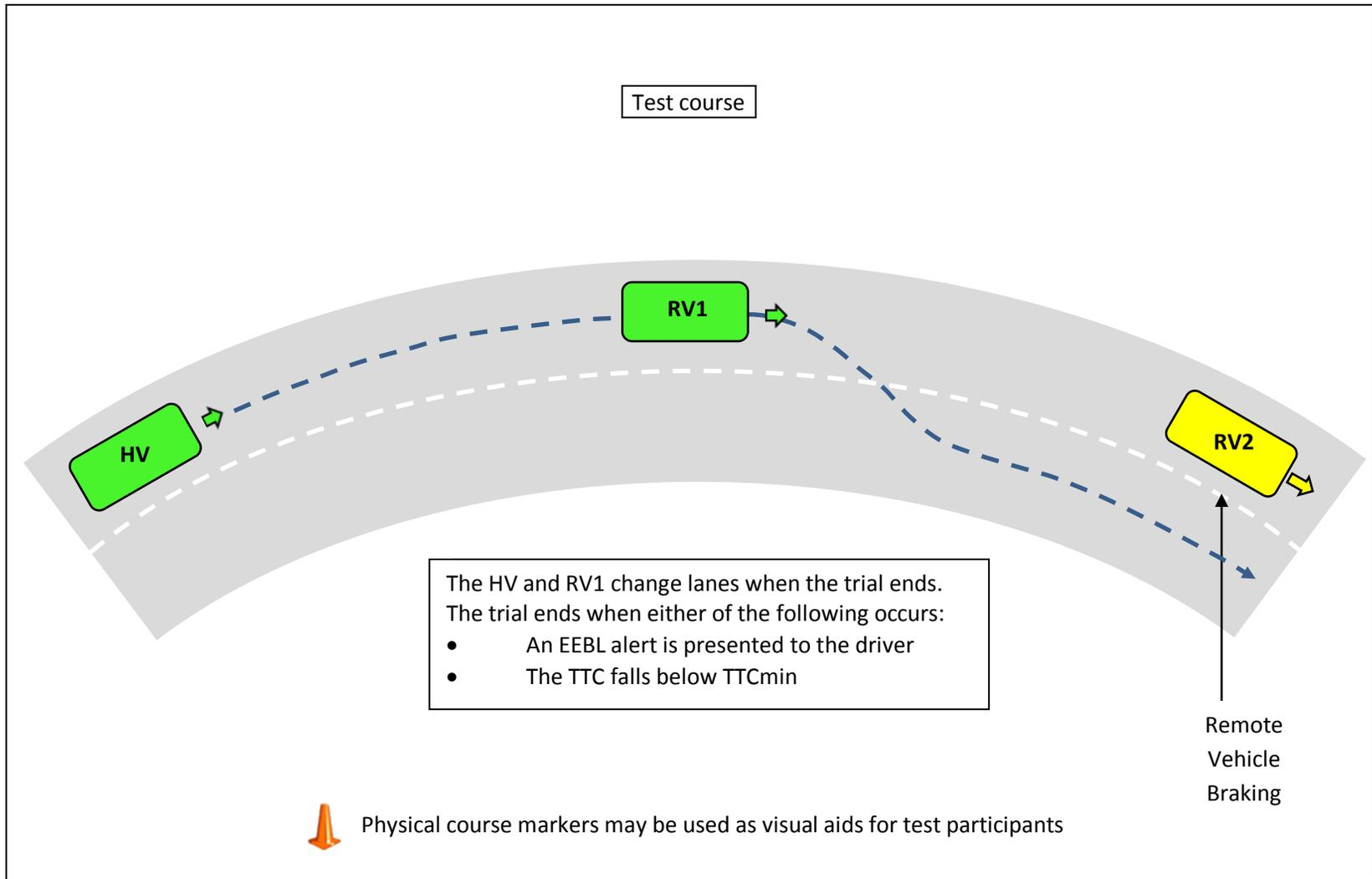
**Figure A-11 - EEBL-5 Test Course Graphic, End of Trial (not to scale)**
