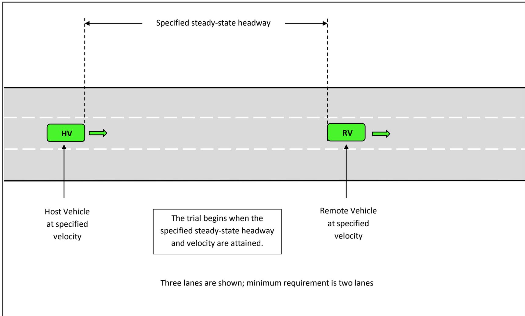
Figure A-14 - EEBL-7 Test Course Graphic, Initial Conditions (not to scale)
