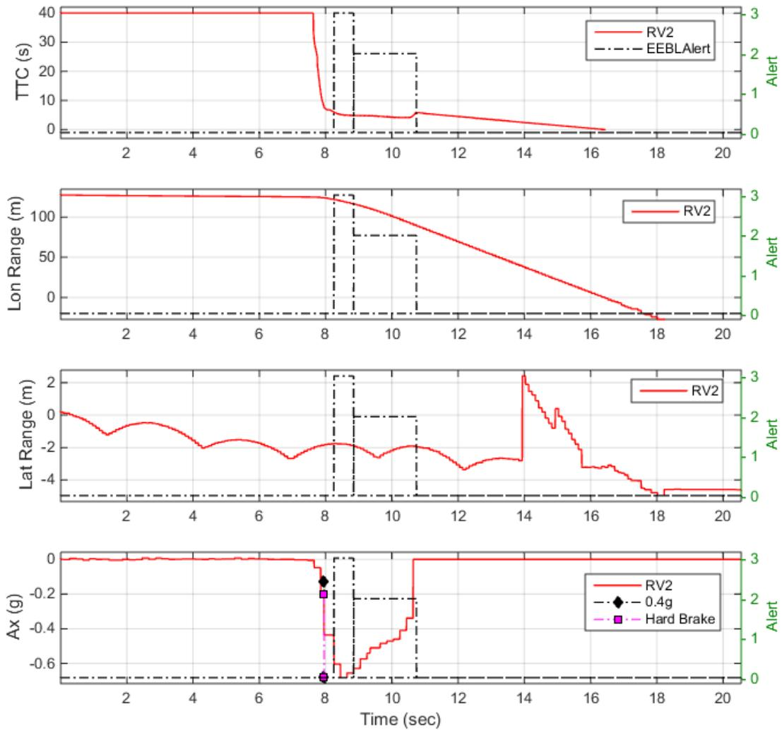
**Figure 18: False EEBL Level 3 Alert Prior to EEBL Level 2 Alert – Test 1257**
