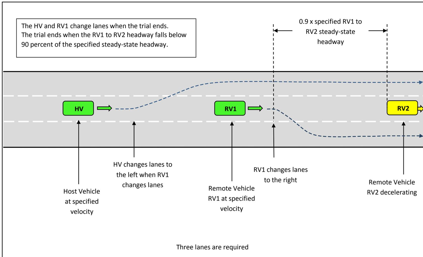
**Figure A-3 - EEBL-1 Test Course Graphic, End of Trial (not to scale)**
