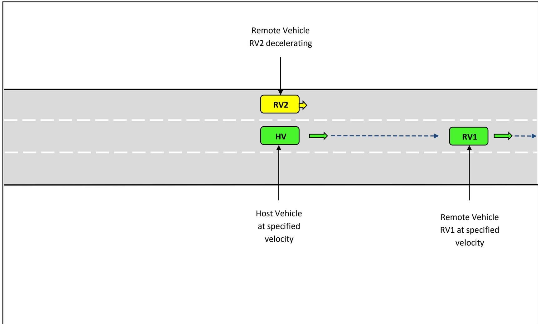
Figure A-9 - EEBL-4 Test Course Graphic, End of Trial (not to scale)
