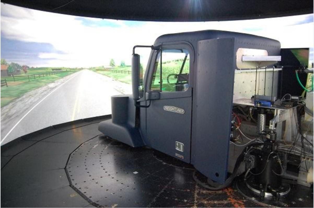
Figure 3. Freightliner Tractor Cab Mounted in NADS-1 Simulator
