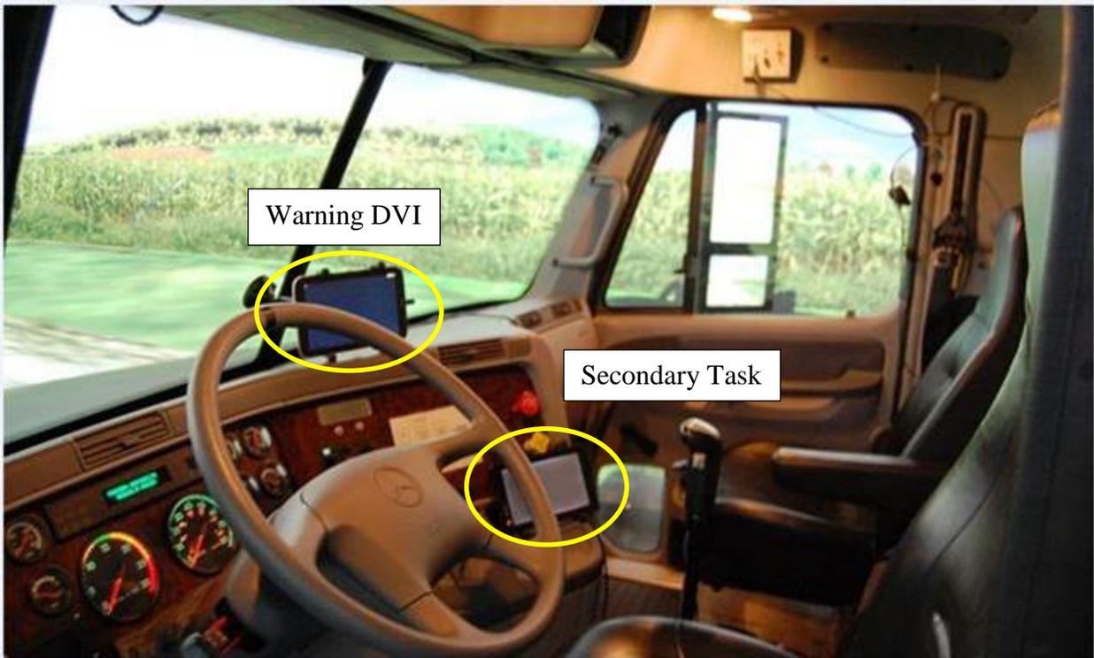
Figure 4. Freightliner Tractor Cab Interior - NADS-1 Simulator
