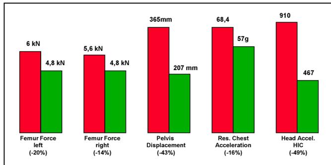
\*) Reduced head acceleration: A head contact to the wind screen was avoided because of an earlier beginning of chest rotation
