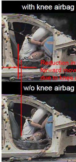
Reduction in pelvis forward movement due to knee airbag
