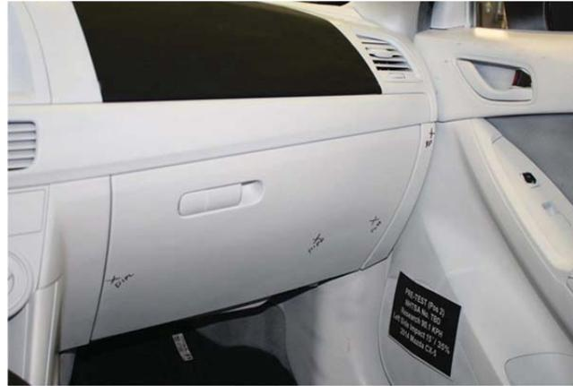
**Picture 4.39: Pre-test Center View of Passenger Knee Bolsters**
