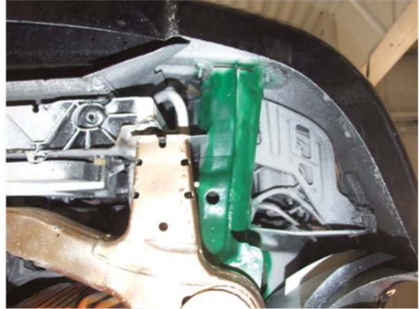
**Picture 4.27: Pre-Test left Bumper to Rail Attachment Top View**
