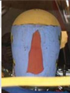
Note: The driver and passenger ATDs shall have clothes of a contrasting color to each other so that the motion of each dummy can be easily identified during video analysis.
