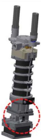
Figure 6.3. Location of neck pitch change mechanism indicator.
