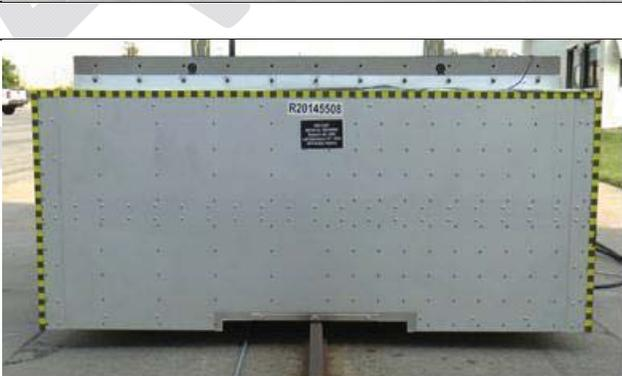
A front-side view of a white honeycomb barrier mounted on a red OMDB. The barrier has yellow and black hazard markers. A white label on the barrier reads: R20145508.                                                                                                                                                           |
