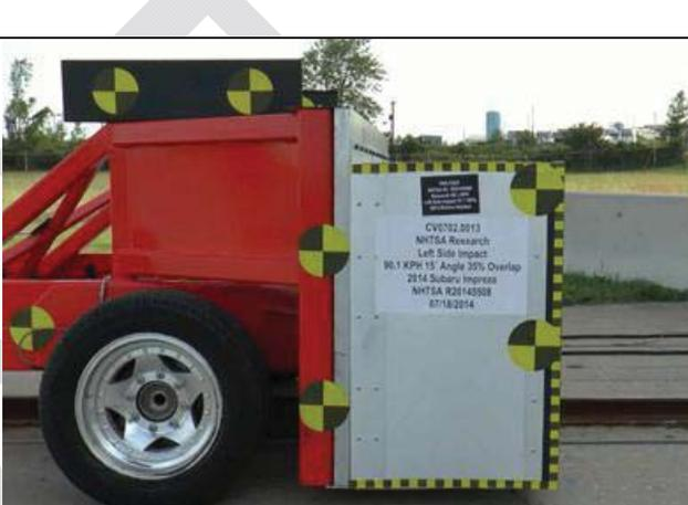
A right-side view of a red OMDB (Off-Median Barrier Device) with a white honeycomb barrier. The barrier has yellow and black hazard markers. A white label on the barrier provides test details: CVT02.2013, NHTSA Research, Left Side Impact, 90.1 KPH 15° Angle 35% Overlap, 2014 Subaru Impreza, NHTSA R20145508, 07/18/2014. |
