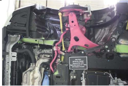
**Picture 4.21: Pre-Test Sway Bar Left Side View**
