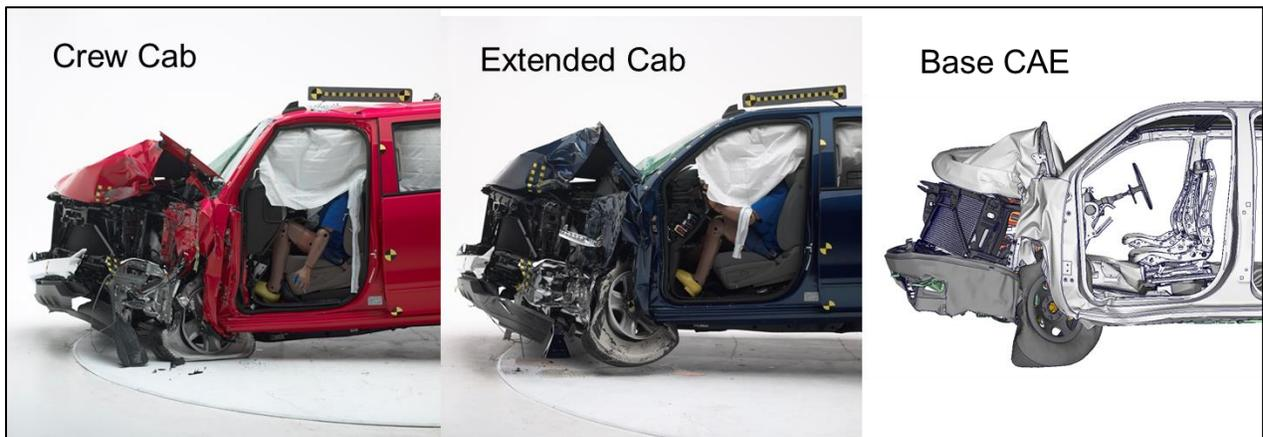
Figure 88: Test Versus CAE Base - Post-Crash Comparison
