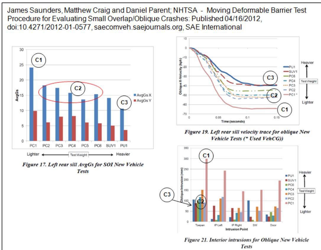
Figure 1: Vehicle Passenger Compartment Acceleration, Velocity and Interior Intrusions<sup>3</sup> (Categories C1 to C3 Marked by EDAG)
