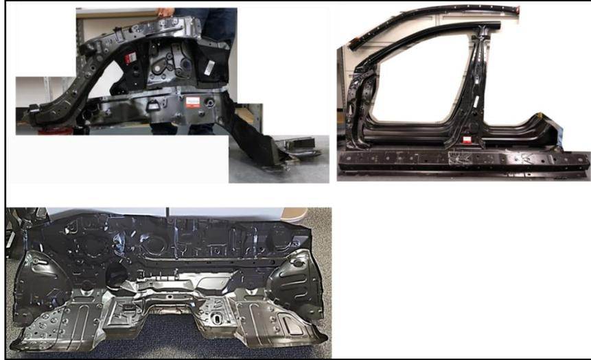
Figure 8: 2014 Honda Accord Body Structure Panels
