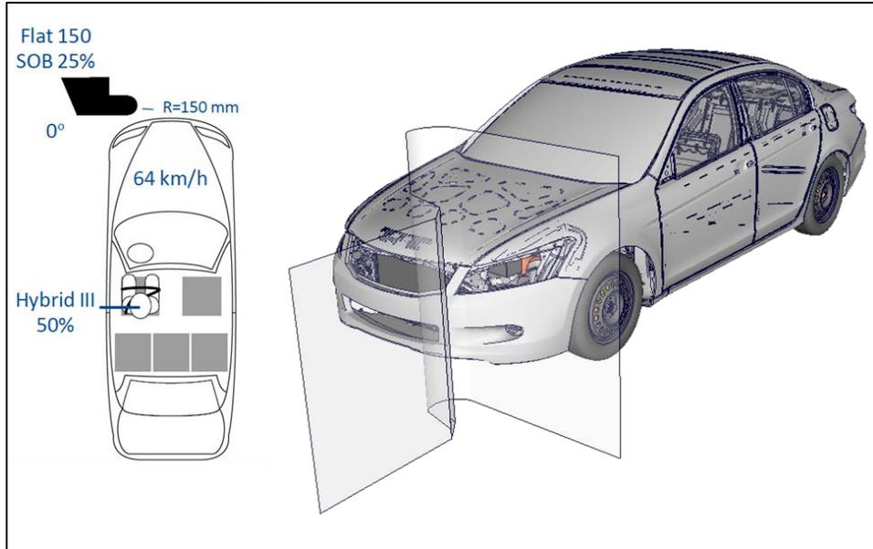
Figure 48: IIHS Small Overlap Test – Test Setup
