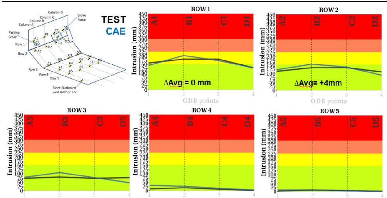
Figure 36: Test Versus CAE - Passenger Floor Pan Intrusion
