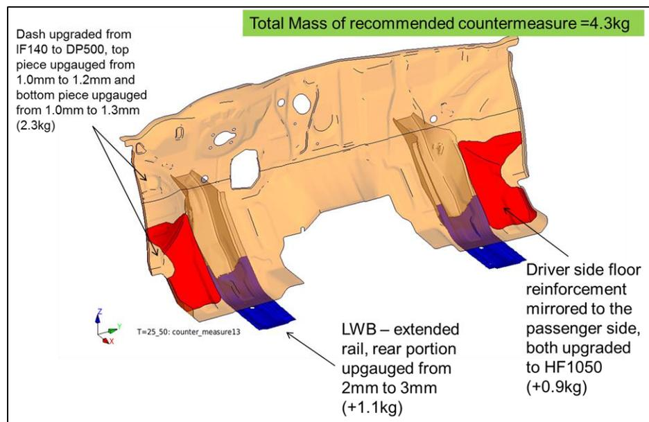
Figure 12: Structural Countermeasures to Reduce Occupant Compartment Intrusions
