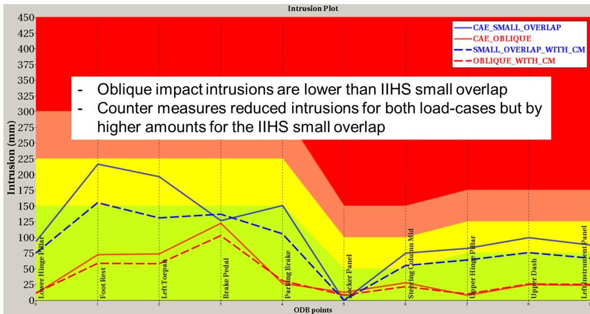
Figure 17: Structural Countermeasures: Reduce Occupant Compartment Intrusions for Oblique and IIHS Small Overlap
