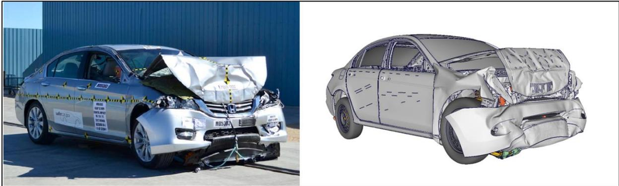
Figure 41: Test Versus CAE Model – Post-Crash Comparison
