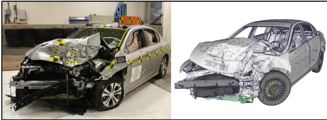
Figure 22: NHTSA Oblique Test Left – Post-Crash Comparison Test Versus CAE Baseline
