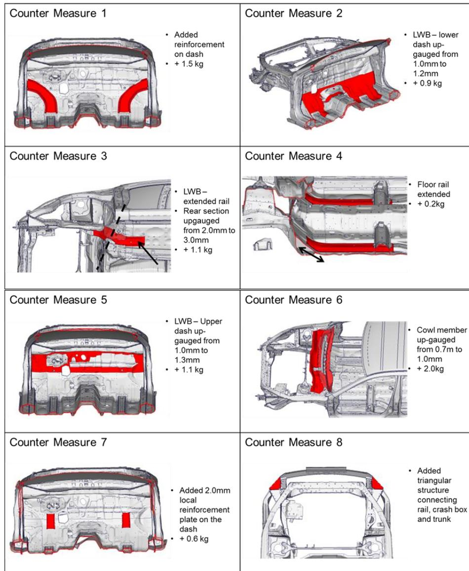
Figure 10: Body Structural Countermeasures 1 to 8
