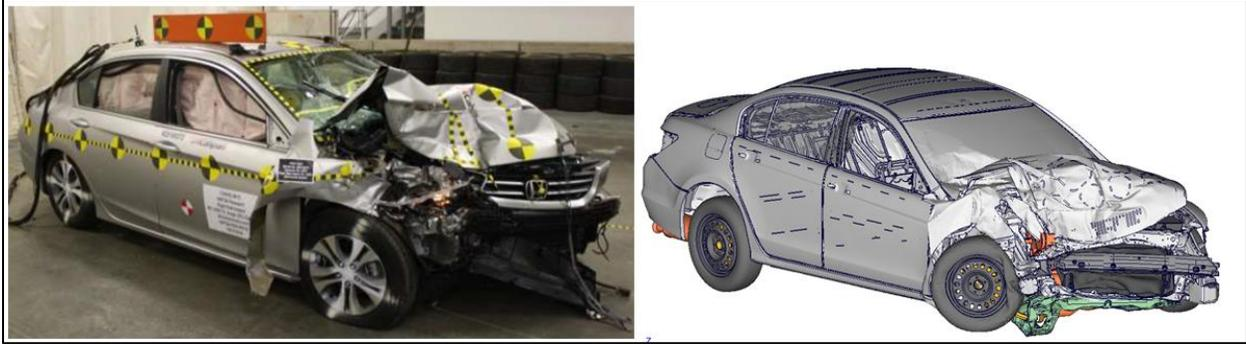
Figure 32: Test Versus CAE – Post-Crash Comparison
