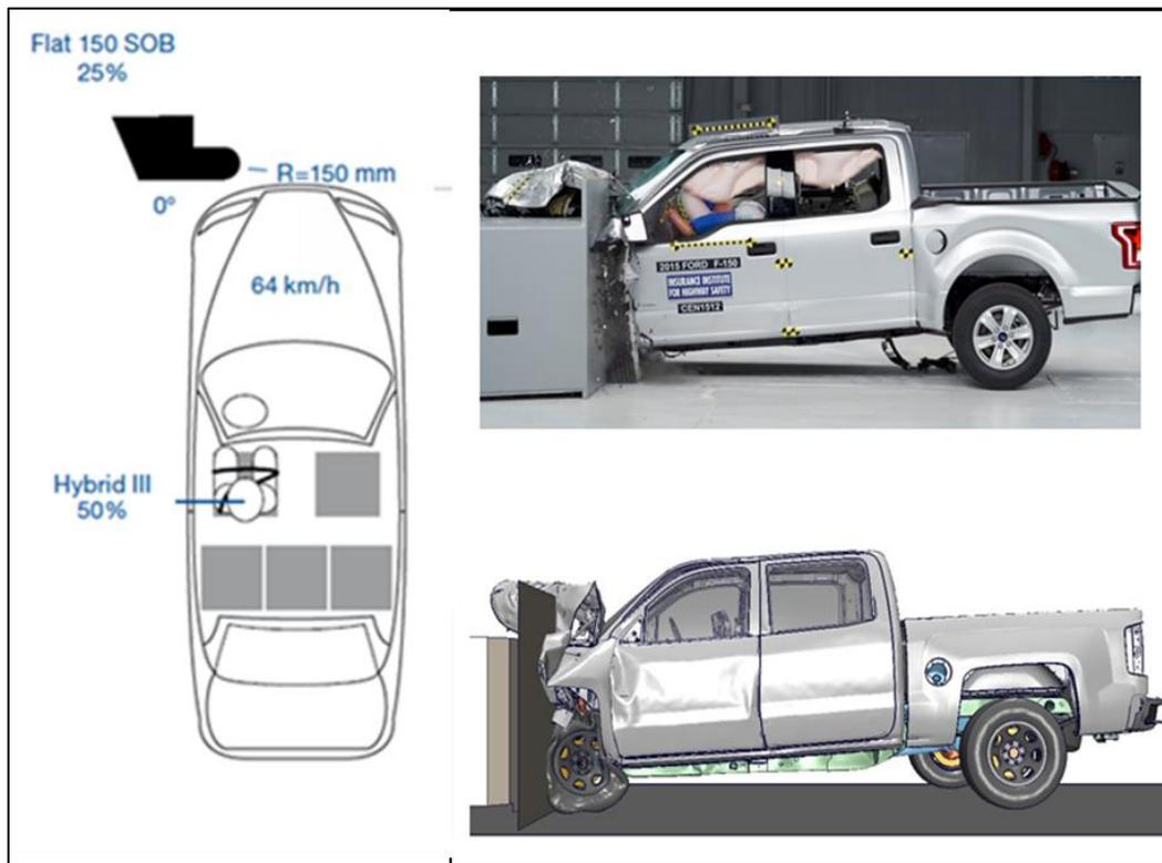
Figure 86: IIHS Small Overlap Test – Test Setup
