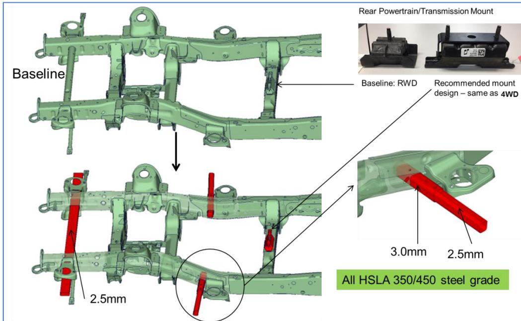
Figure 15: Structural Countermeasures to Reduce Occupant Compartment Intrusions
