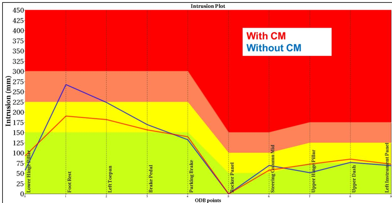
Figure 94: Without Versus With Countermeasure – IIHS Intrusion
