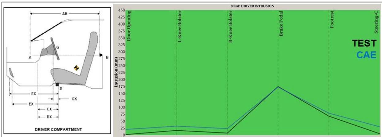
Figure 26: Test Versus CAE NCAP Driver Compartment Intrusion
