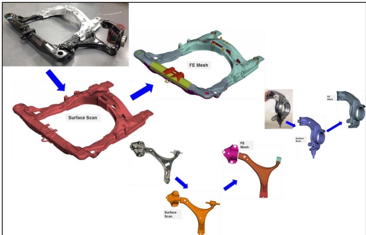
Figure 7: 2014 Honda Accord Engine Cradle and Front Suspension
