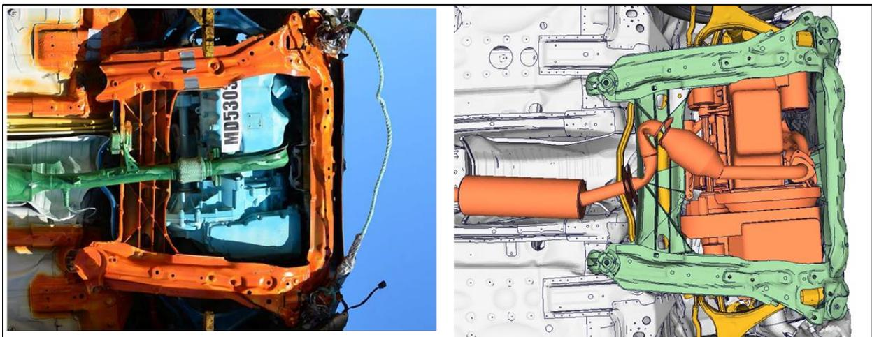
Figure 42: Test Versus CAE Model – Post-Crash Comparison
