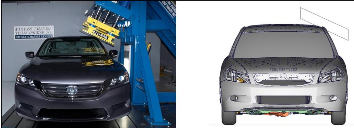
Figure 52: IIHS Roof Strength Test - LS-DYNA Model Setup
