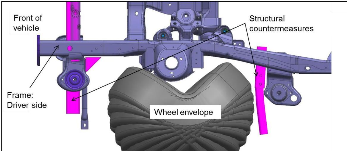
Figure 16: Structural Countermeasures to Reduce Occupant Compartment Intrusions
