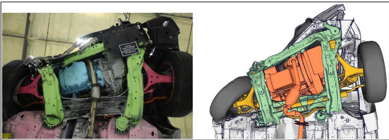
Figure 33: Test Versus CAE – Post-Crash Comparison
