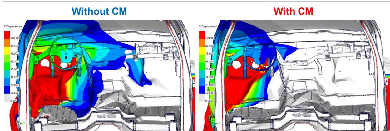
Figure 93: Without Versus With Countermeasure – Dash Panel Intrusion
