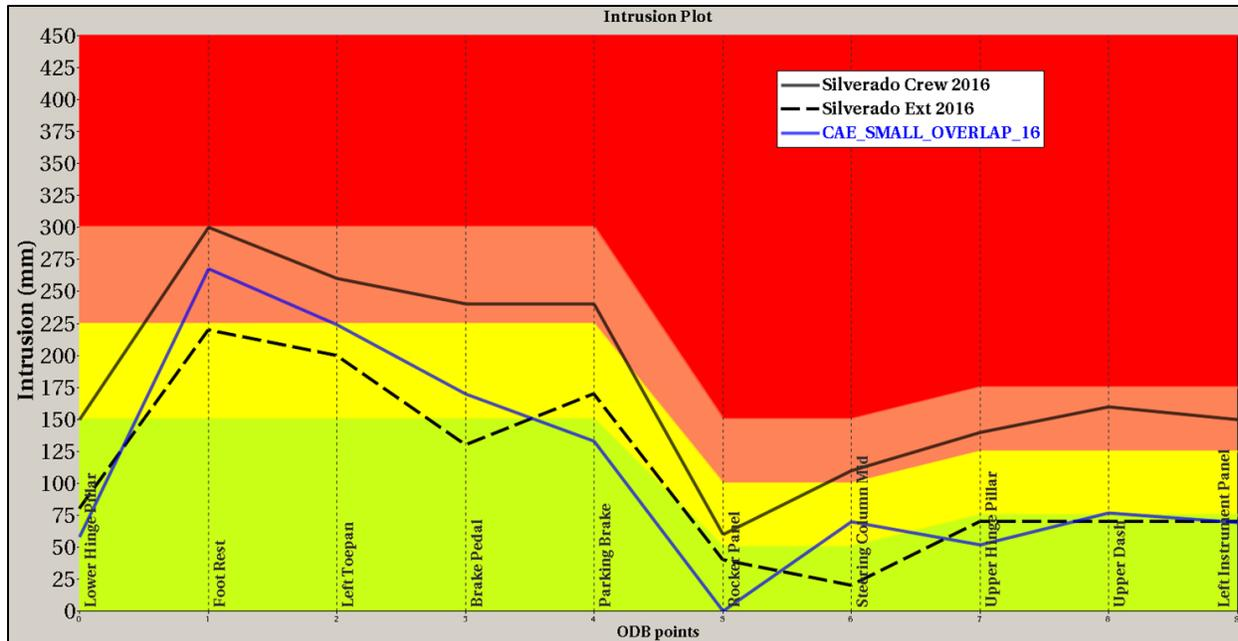
Figure 91: Test Versus CAE Baseline – IIHS Intrusion Plot
