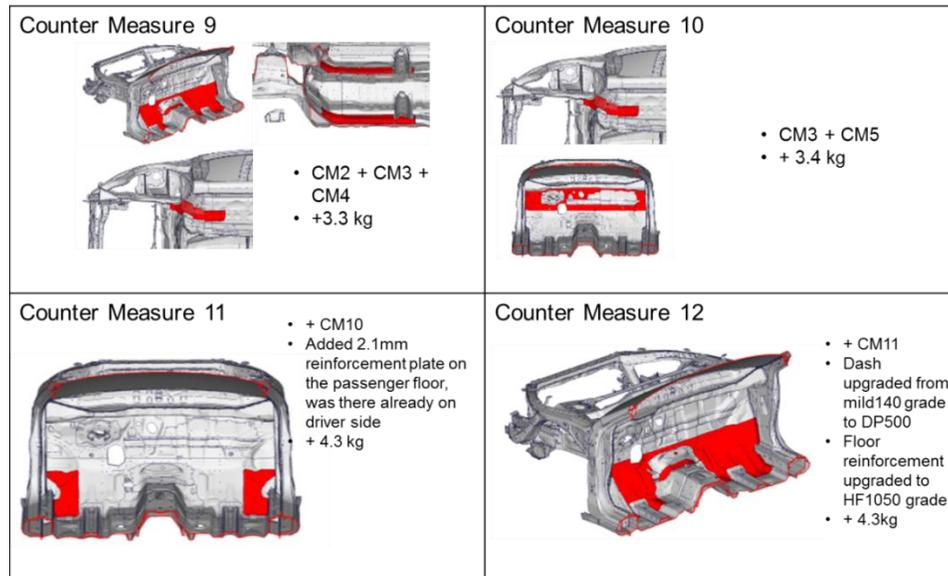
Figure 11: Body Structural Countermeasures 9 to 12
