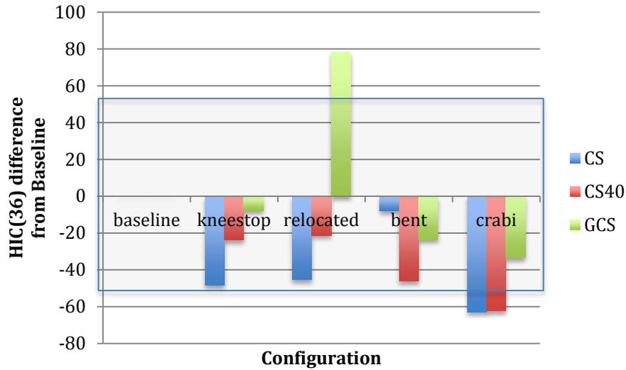
Figure 8. Differences in HIC between baseline and alternative ATD configurations (gray box shows normal range of repeatability).
