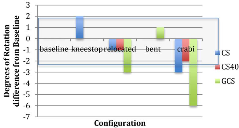
Figure 7. Differences in CRS maximum rotation from baseline condition for each model (gray box shows normal range of repeatability).
