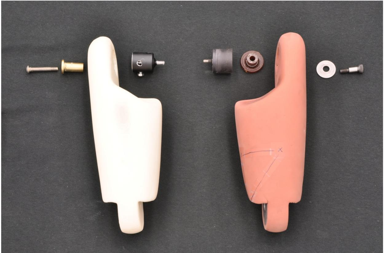
Figure A4. Ball joint (left) and standard joint (right).
