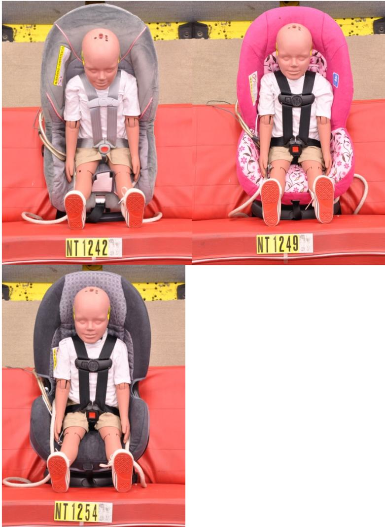
Figure A1. Elevated leg posture used with standard 3YO ATD, with knee stops removed.
