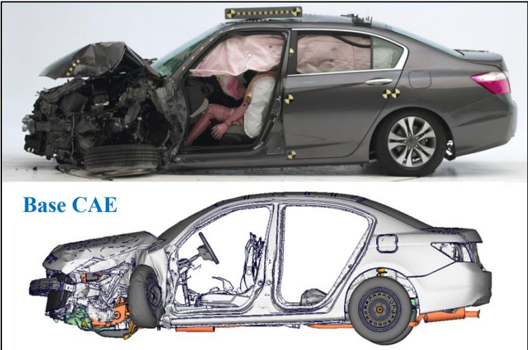
Figure 9: IIHS Small Overlap Test Versus Base CAE
