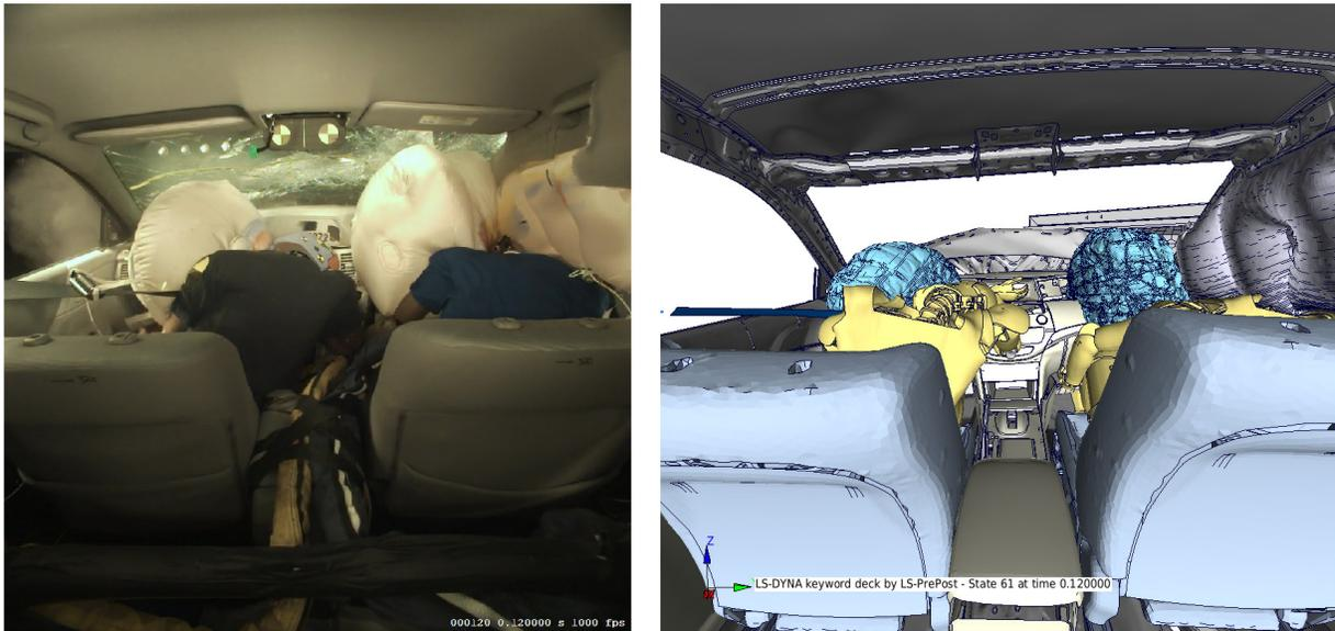
Figure 64: Test Versus CAE at 120 ms
