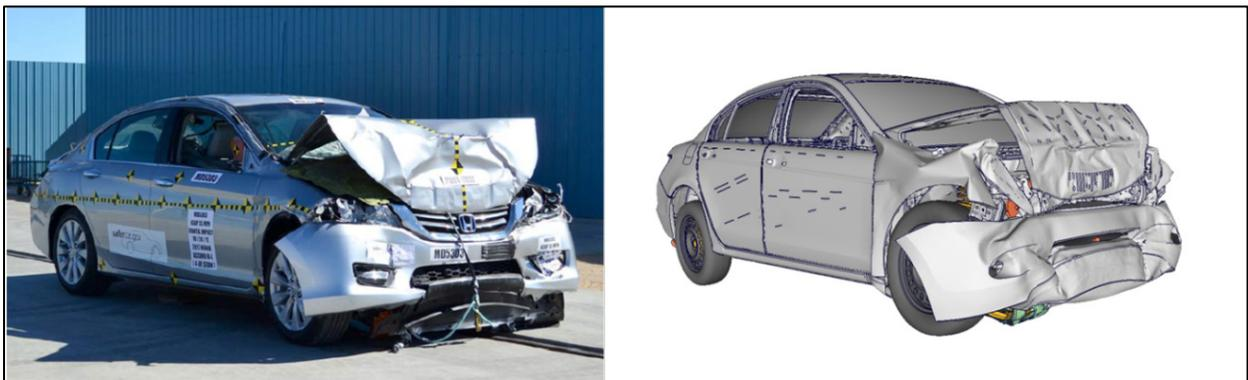
Figure 2: Test Versus CAE Model – Post-Crash Comparison
