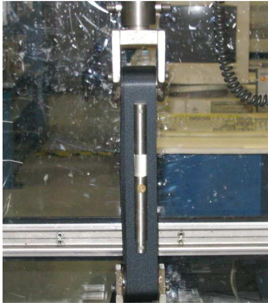
Figure 42: Webbing Elongation Test Setup
