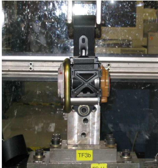
Figure 43: Retractor Pay-out (load limiter) Test Setup
