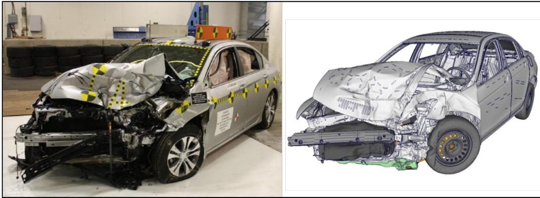
Figure 13: NHTSA Oblique Test Left – Post-Crash Comparison Test Versus CAE Baseline
