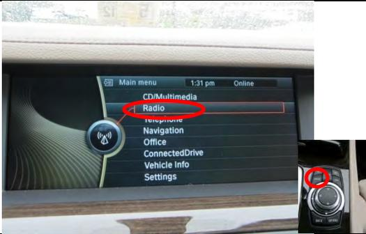
Turn Radio on by pressing the 'Radio' hard button on lower center console, located in front of the primary controller (Note: An alternate method would be to use the primary controller to highlight 'Radio' on the screen by using the rotary dial and then press in on the knob; but that would be a separate testable task, and should be tested separately).
