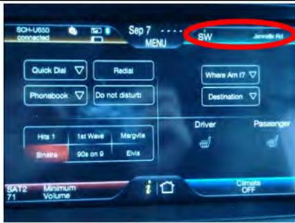
Touch green navigation bar in upper right of touch screen. (Its current label indicates direction of travel/heading and destination.)
