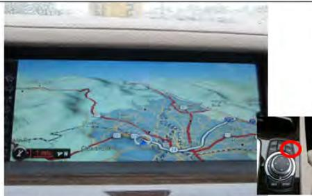
Press the ‘Nav’ button on lower center console (Note: An alternate method is to highlight ‘Navigation’ using the rotary dial, then press in knob – a separate testable task).
