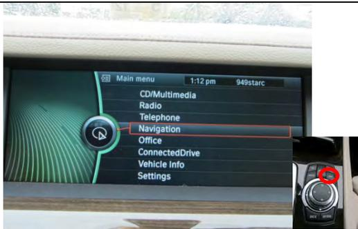
Press the "Navigation" button on lower center console. (An alternate method would be to highlight 'Navigation' using the rotary dial, then press in knob; a separate testable task).
