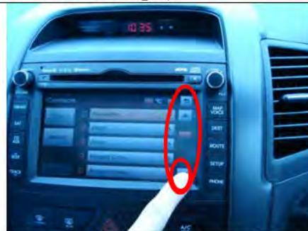
And to continue looking for the desired name, press the scroll down-arrow again (3<sup>rd</sup> time).
