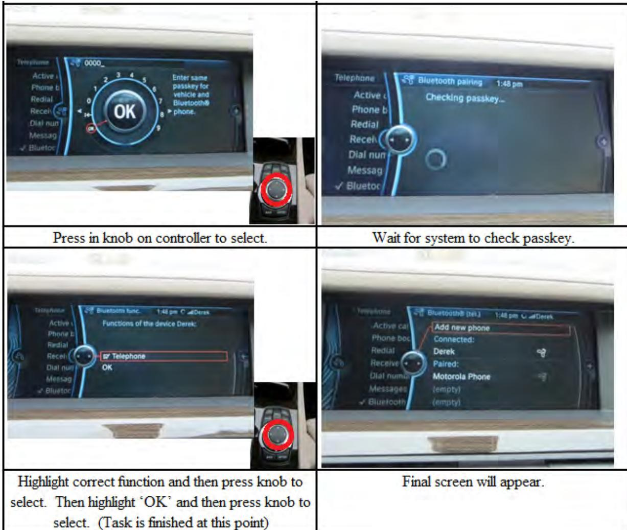
**The task end state** would be reached when the device successfully accepts connection of the handheld device.
