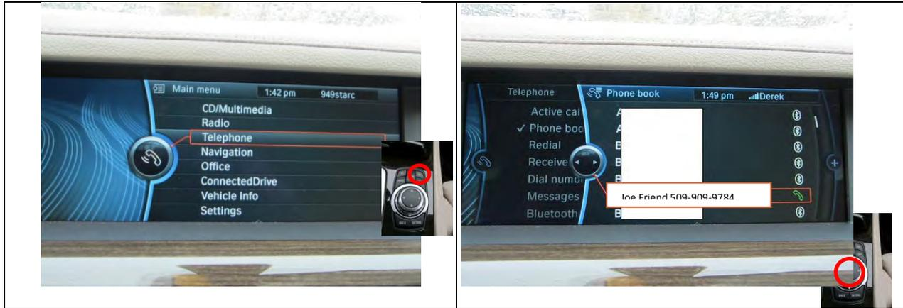
Press the “Tel” button on lower center console (or an alternate method would be to use the rotary dial to highlight “Tel” and then press in knob; but that would be a separate testable task, and need to be tested separately).
