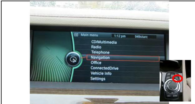
Press the 'Navigation' button on lower center console. (Again, there is an alternate way to do this, by using the rotary knob to highlight "Navigation" and then pressing in knob; a separate testable task.)
