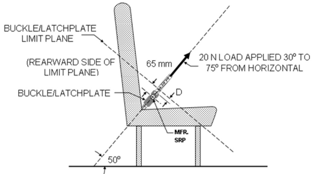
D = Shortest distance from the limit plane to the buckle/latchplate.
