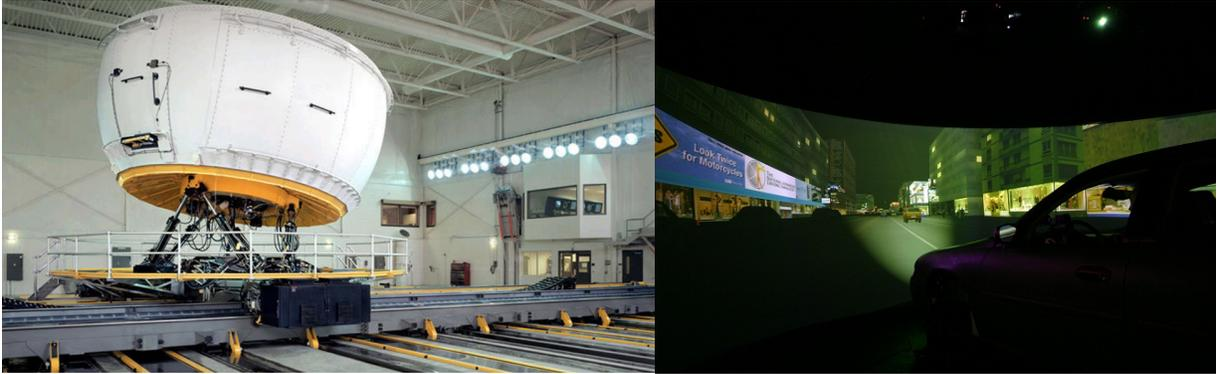
Figure 1. Representation of NADS driving simulator (left) with a driving scene from inside the dome (right).
