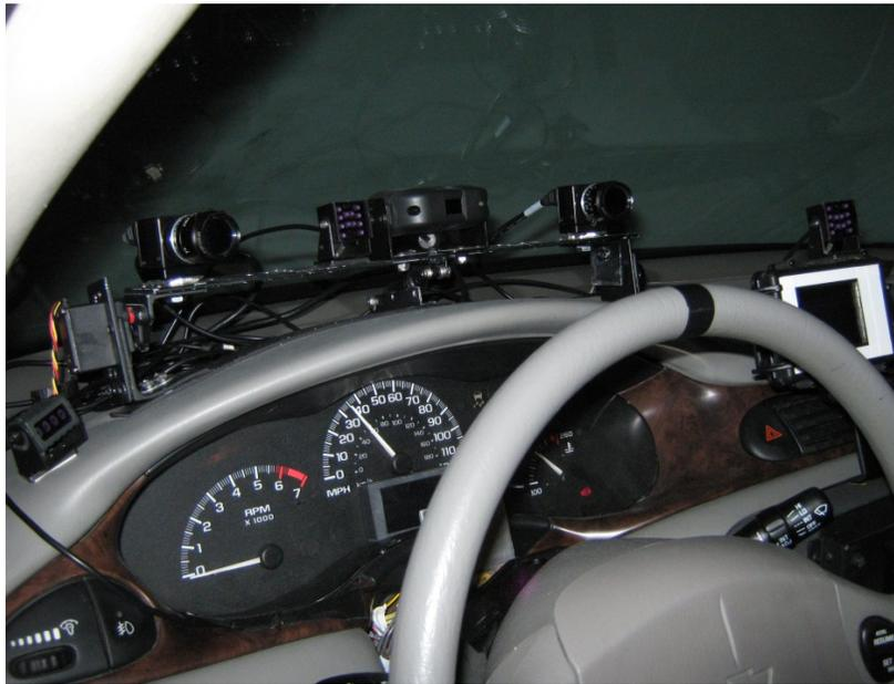
Figure 2. Face Lab cameras mounted in the Malibu cab with a separate head tracking system mounted between them.
