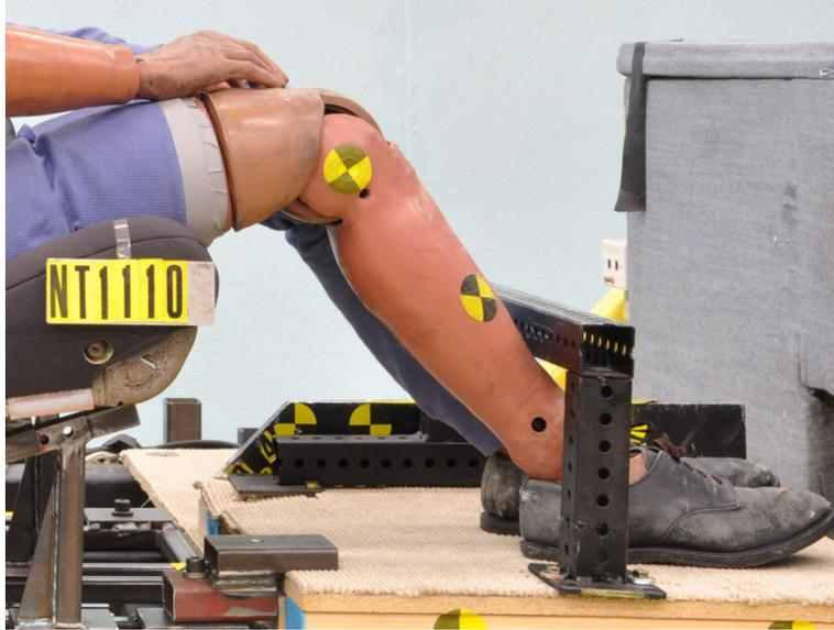
Figure 6. Hardware simulating floor and shin/vehicle seat interaction
