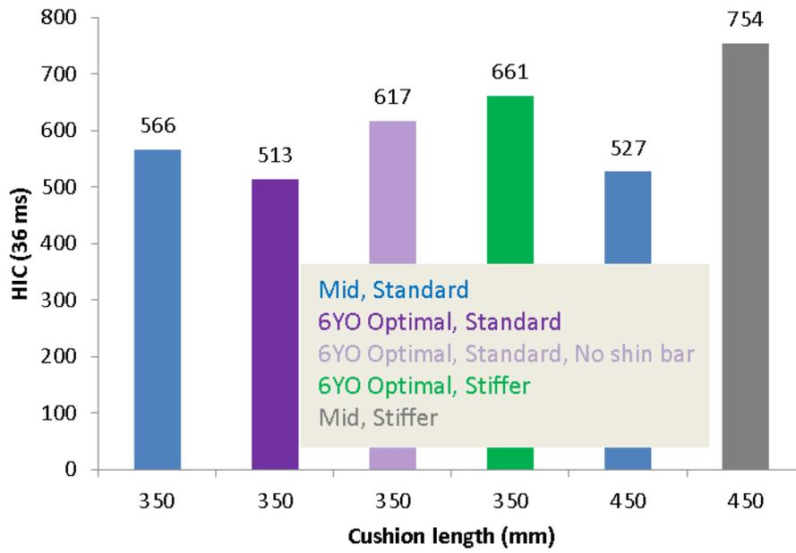
Figure 15. HIC (36 ms) values for each test condition
