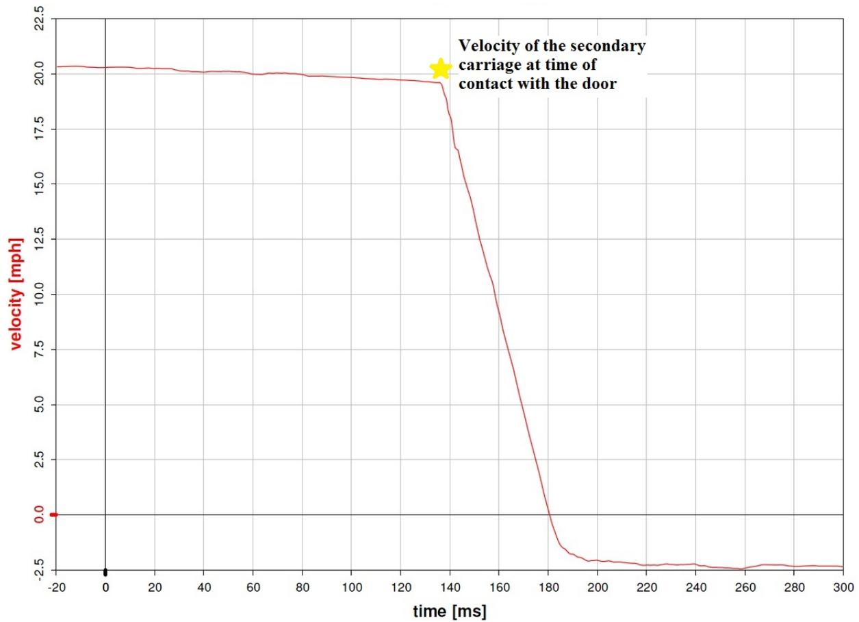
Figure A2: Integration of the secondary carriage acceleration
