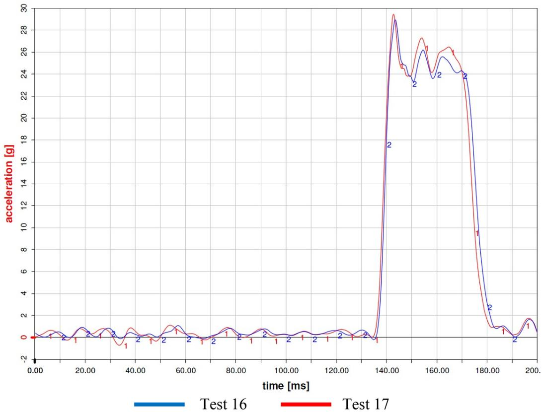
Figure 20: Secondary carriage acceleration (seat back position) for Tests 16 and 17
