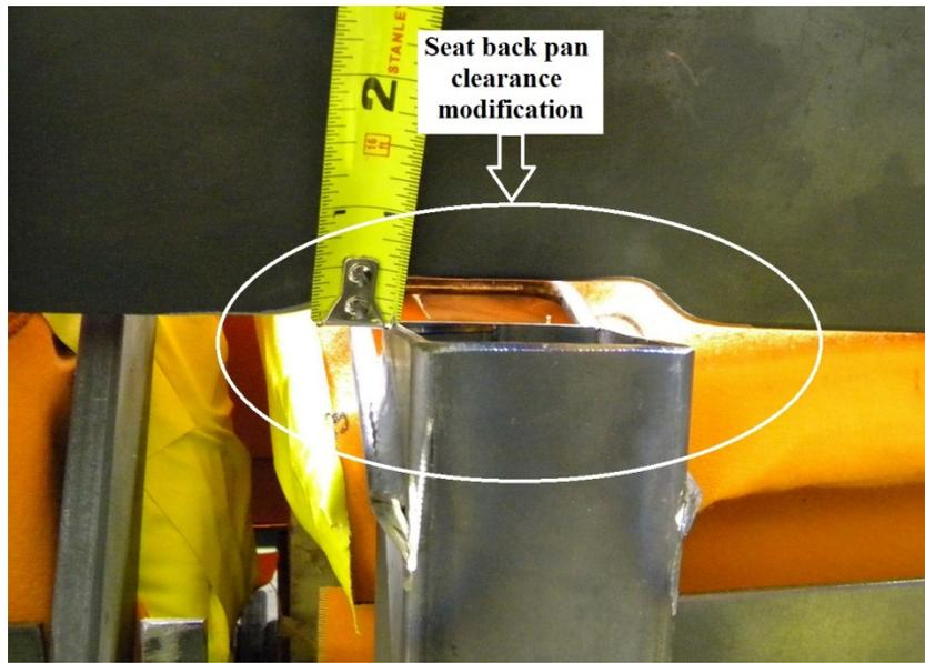
Figure 7: Modification to the seat back pan
