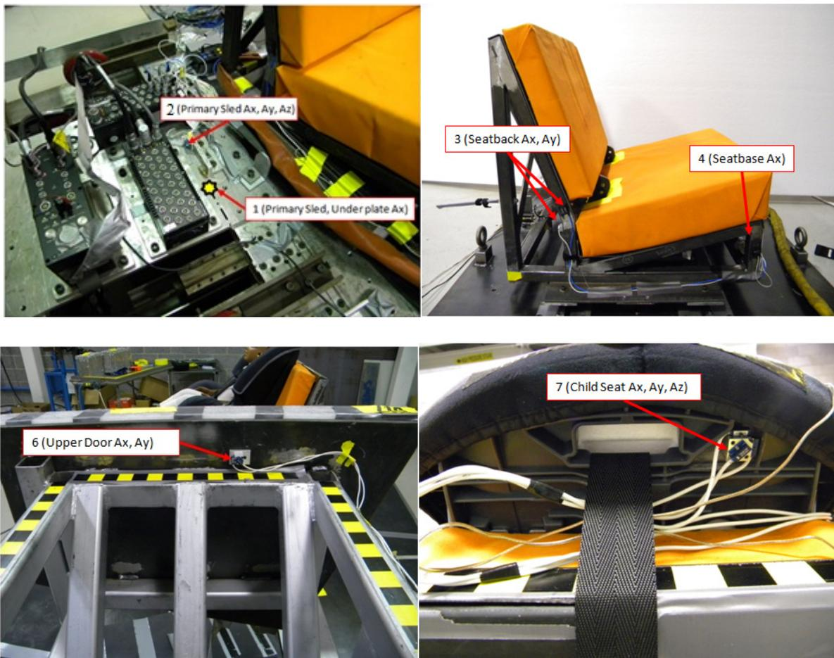
Figure 9: Instrumentation locations
