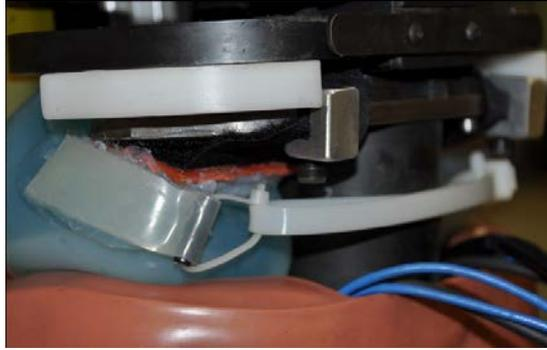
Figure 6. Method of attaching top of gel abdomen.
