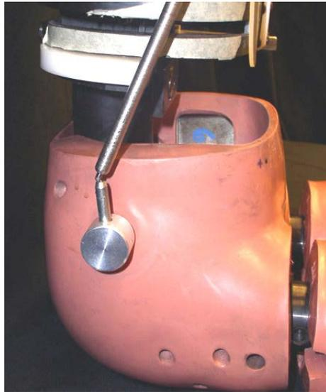
Figure 10. Illustration of hip offset tool to facilitate measurement of pelvis orientation using the FARO arm.
