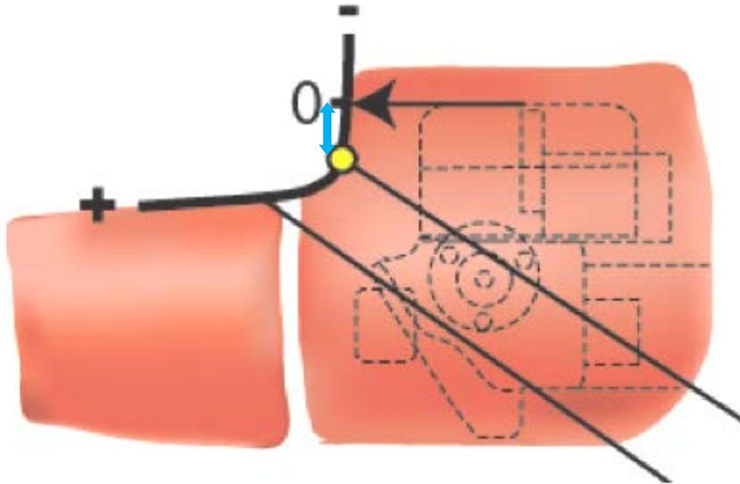
Figure 9. Illustration of lap belt score (LBS) measurement.
