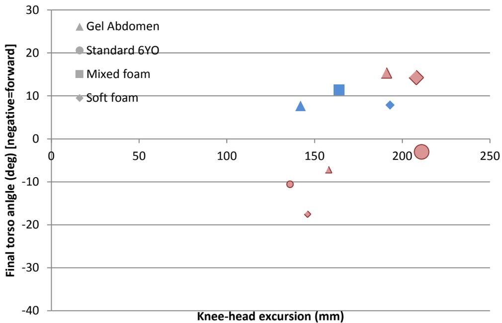
Figure 15. Final torso angle (deg) vs. knee-head excursion (mm) for standard ATD and modified ATD using gel and foam abdomens
