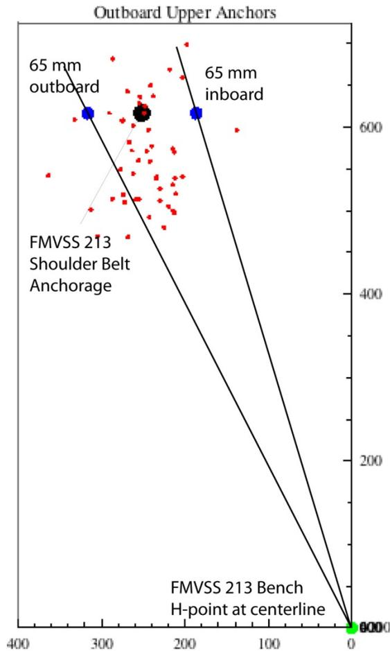
Figure 3. Front view of shoulder belt anchorage locations from vehicle rear seats (small dots) compared with FMVSS No. 213 shoulder belt anchorage and inboard and outboard shoulder belt anchorages. Origin is SAE J826 H-point on the centerline of the outboard seating position on the FMVSS No. 213 bench.
