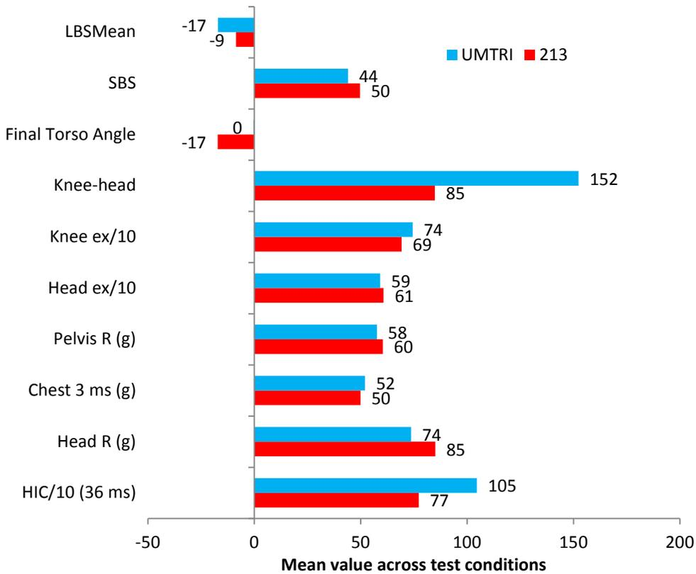
Figure 16. Mean values of outcome measures for FMVSS No. 213 and UMTRI seating procedures using the modified ATD.
