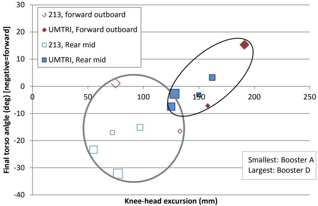
Figure 17. Final torso angle (deg) vs. knee-head excursion (mm) for tests using UMTRI (filled, black oval) and FMVSS No. 213 (open, gray oval) seating procedures under matched booster/geometry conditions with the modified ATD.
