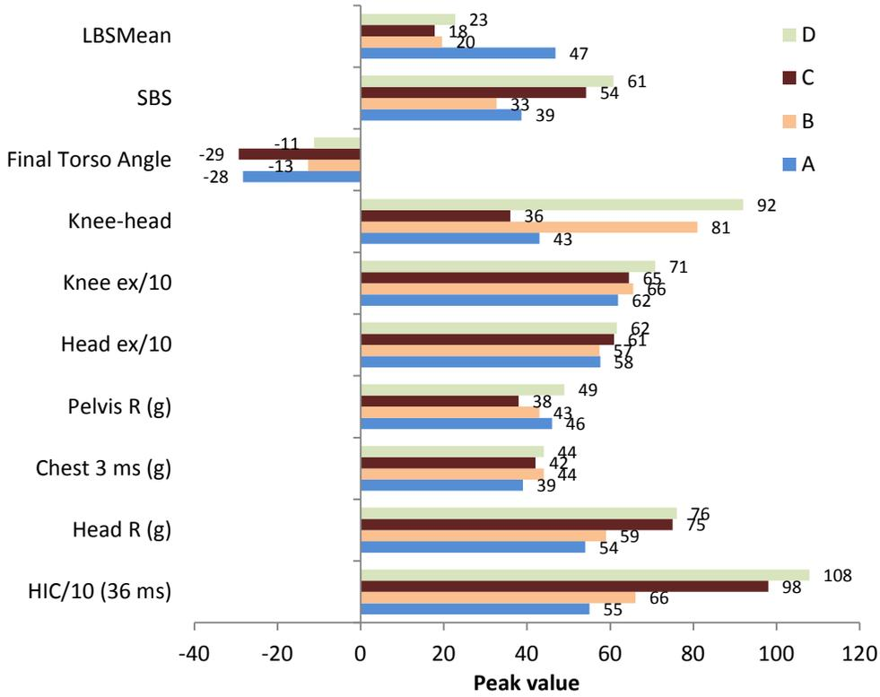
Figure 11. Peak values of outcome measures for each booster under FMVSS No. 213 baseline conditions.
