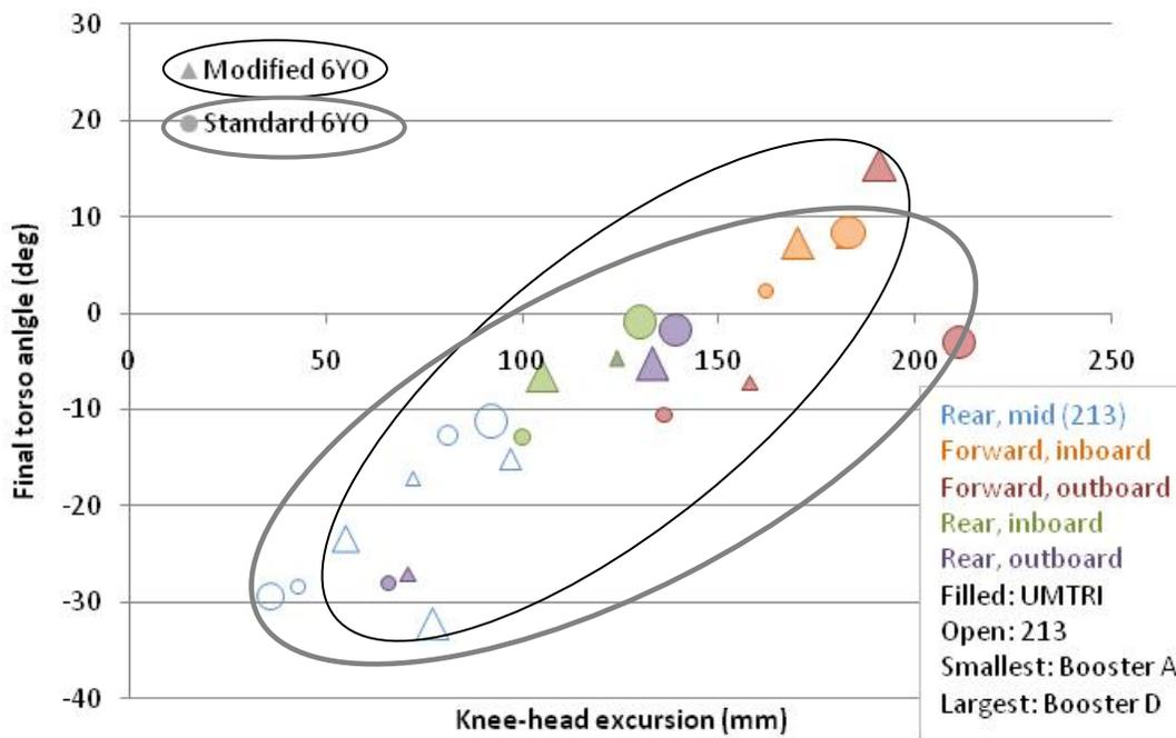
Figure 14. Final torso angle (deg) vs. knee-head excursion (mm) for standard ATD and modified ATD with gel abdomen.
