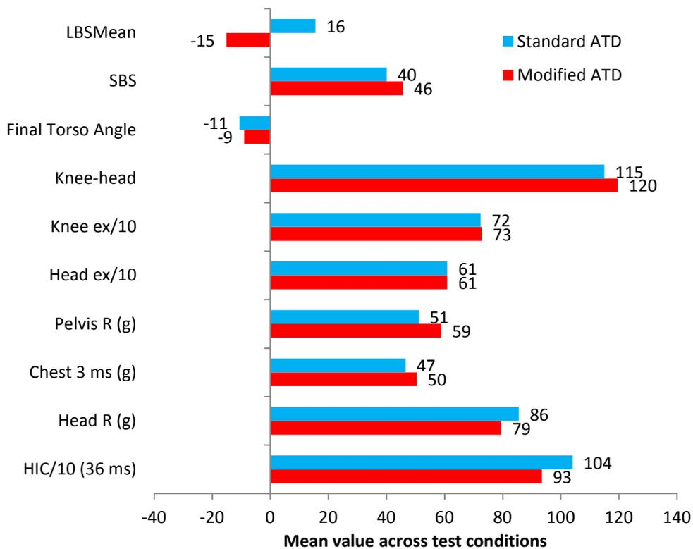
Figure 13. Mean values of outcome measures for standard and modified ATDs for all paired test conditions.
