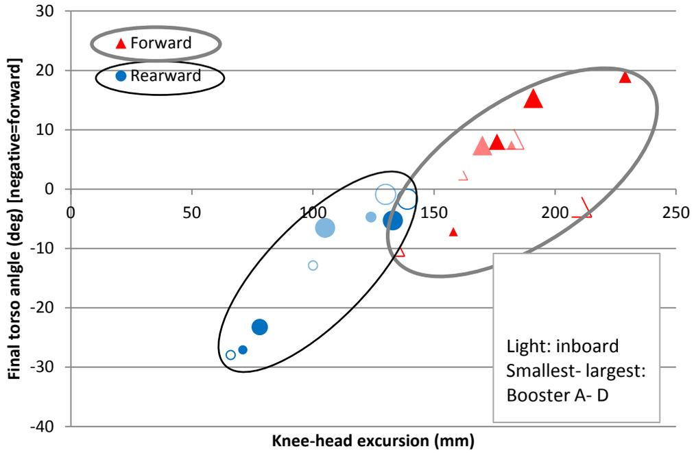
Figure 21. Final torso angle (deg) vs. knee-head excursion (mm) for forward and rearward lap belt anchorages.
