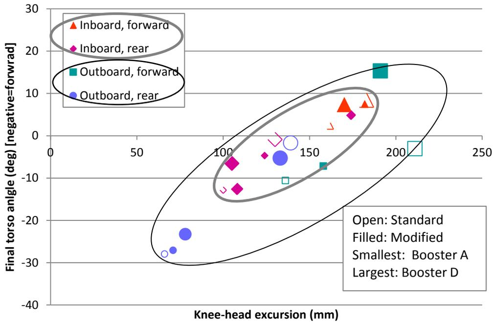
Figure 19. Final torso angle (deg) vs. knee-head excursion (mm) for under inboard and outboard shoulder belt anchorages.
