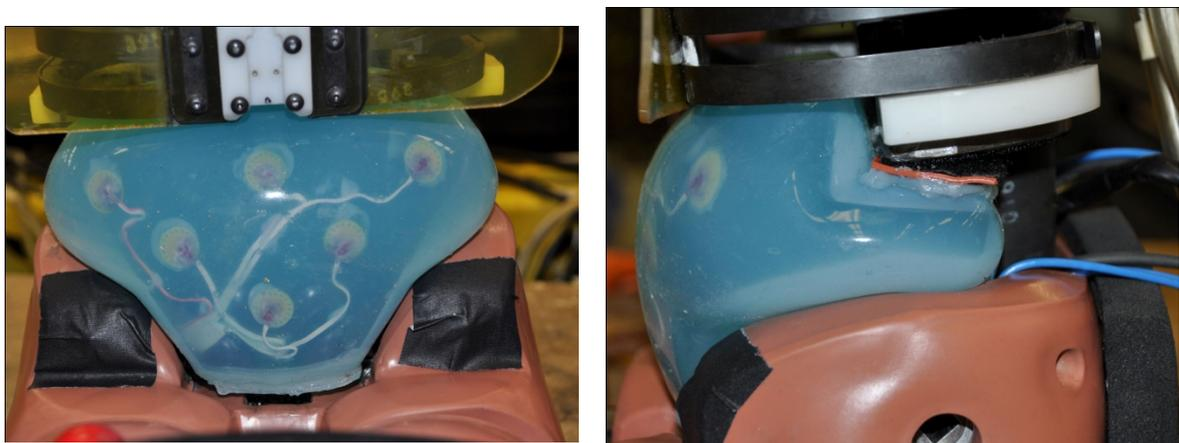
Figure 5. Gel abdomen installed in pelvis.
