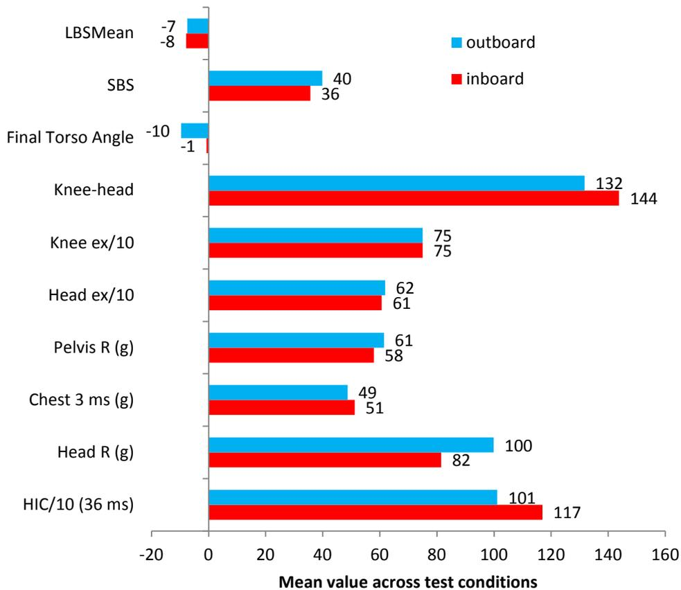
Figure 18. Mean values of outcome measures inboard and outboard shoulder belt locations.
