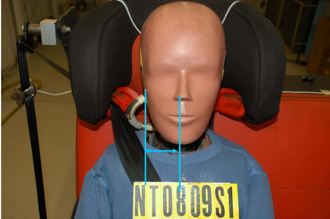
Figure 8. Illustration of shoulder belt score (SBS) measurement.
