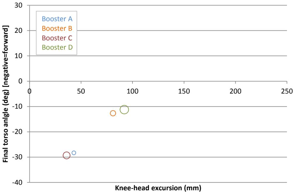
Figure 12. Final torso angle (deg) vs. knee-head excursion (mm) for baseline testing of four boosters using FMVSS No. 213 procedures.
