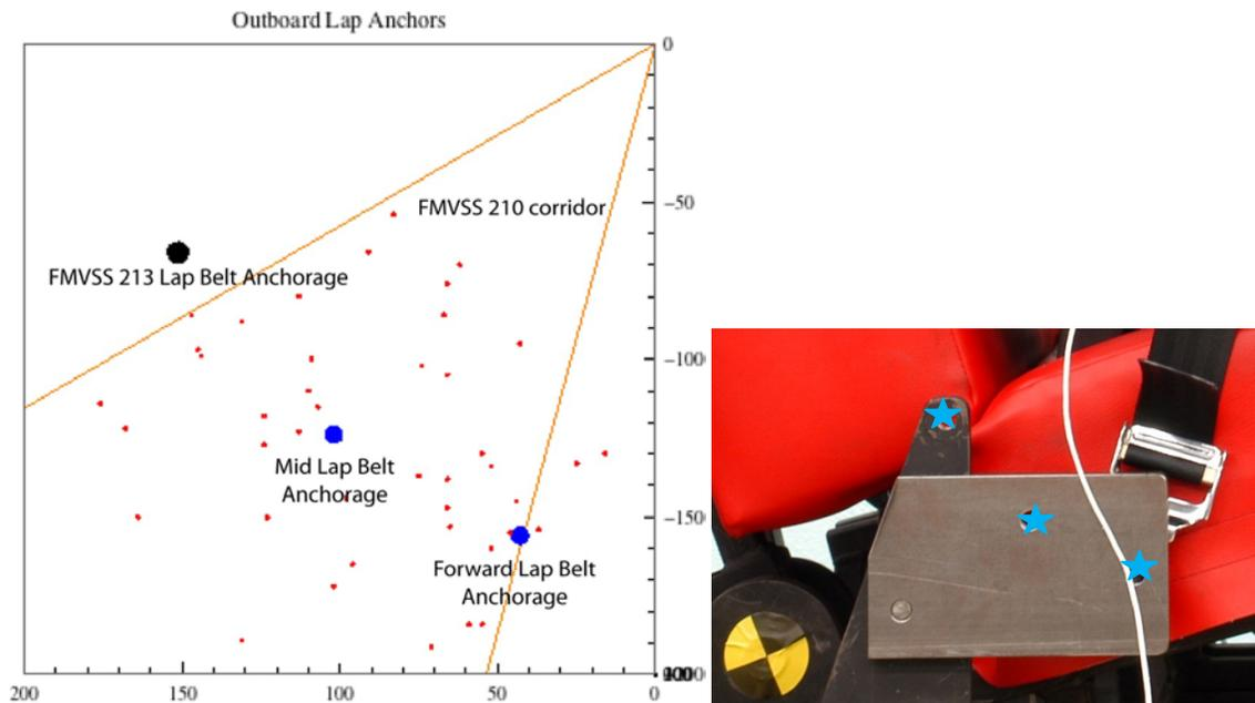
Figure 1. Side view of lap belt anchorage locations from vehicle rear seats (small dots) and anchorages selected for testing. Origin of plot is SAE J826 H-point. Forward is to the right. Photo illustrates hardware implementation with stars indicating belt anchorage locations.
