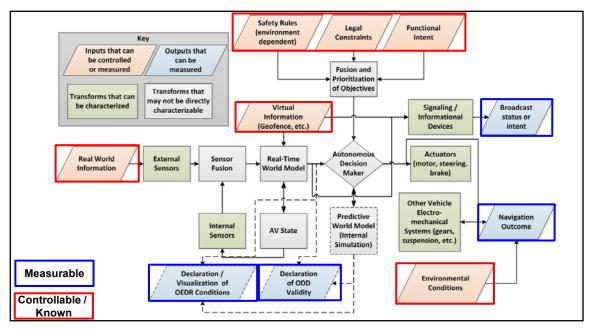
Figure 25. Notional ADS Track Testing Architecture
