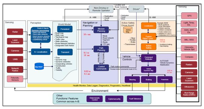
Figure 2. SAE International Autonomous Mode Functional Architecture Flow Diagram (Underwood, 2016)
