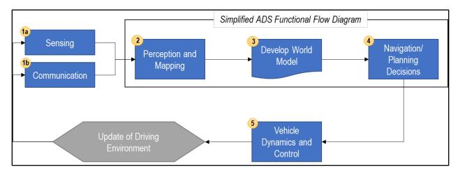
Figure 30. Simplified ADS Functional Flow Diagram
