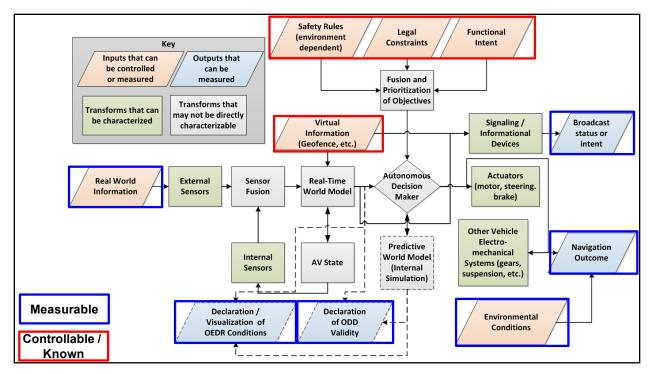
Figure 26. Notional ADS Open-Road Testing Architecture
