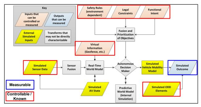
Figure 23. Notional ADS Simulation Architecture
