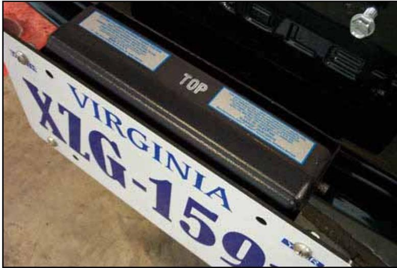
**Figure 6. Doppler Radar Antenna Mounted on the Front of a Vehicle, Covered by One of the Plastic License Plates Used for This Study**
