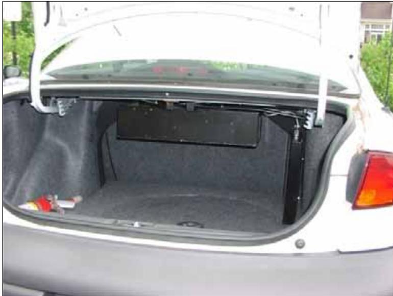
**Figure 5. The Main DAS Unit Mounted Under the Package Shelf of the Trunk**
