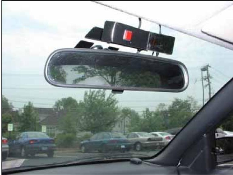
**Figure 7. The Incident Push Button Box and Driver Face/Left Vehicle Side Camera Mounted Above the Rearview Mirror**
