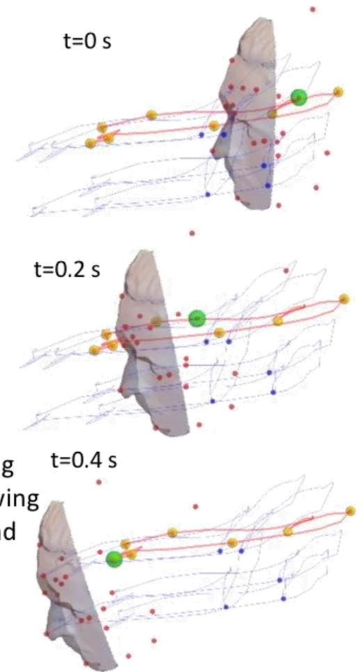
Head Tracking Output Showing Landmark and Head CG Trajectory
