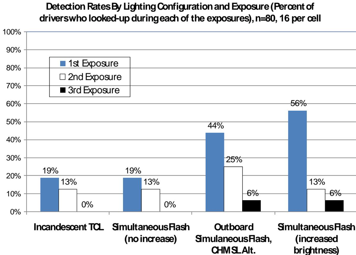
**Figure 27. Percentage of Participants Who Looked up as a Function of Lighting Configuration and Exposure. Note That for Baseline, None of the Participants Looked up on Any Exposure. (Results Are for Explanatory Purposes and May Not Be Statistically Significant Except as Previously Indicated.)**
