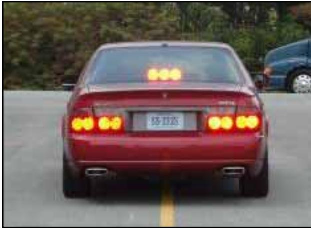
**Figure 38. Research Vehicle With the Rear Lighting Energized at the Emergency Level. (Lighting Was Subjectively “Redder” Than It Appears in the Photograph.)**
