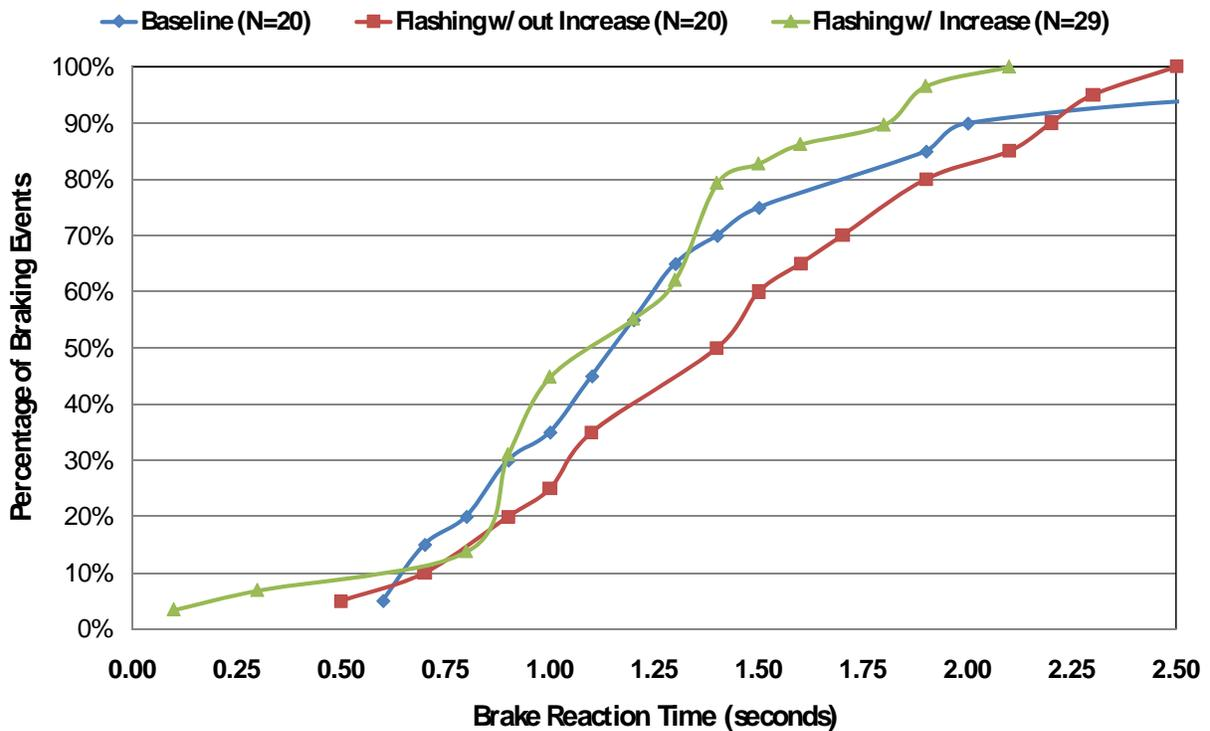
Figure 51. Cumulative Distribution of Brake Response Times (State Route Data Only)
