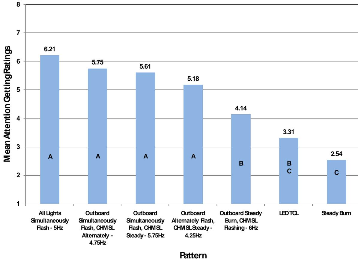
**Figure 14. Results of the Attention-Getting Ratings at 100 ft (30.5 m) Looking to the Right 30 Deg Off Axis**
