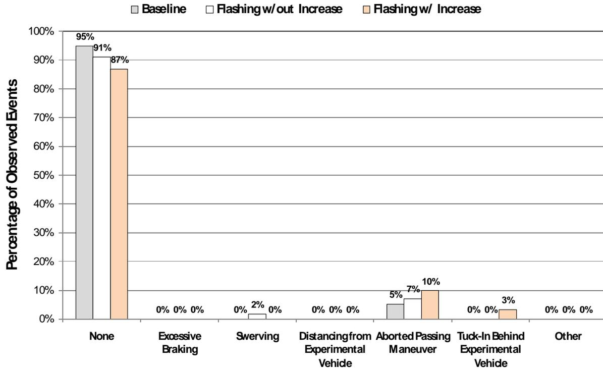
**Figure 54. Incidence of Erratic Behaviors for Adjacent Lane Trials (n=175)**
