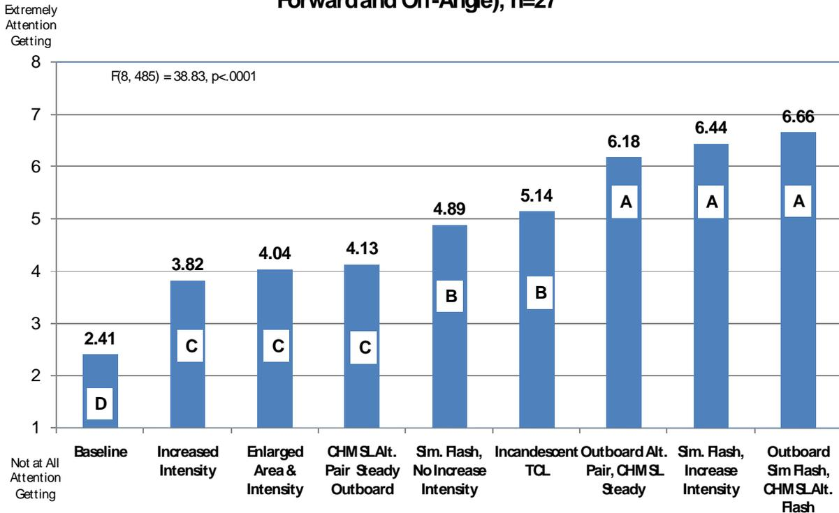
**Figure 32. Main Effect of Lighting Configuration on Attention-Getting Ratings**
