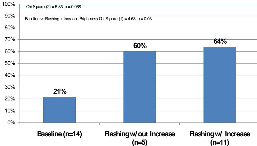
**Figure 47. Percentage of Drivers Who Braked in Response to the Brake Signal as a Function of Lighting Condition for Drivers Who Were Glancing Away at Signal Onset (n=30)**
