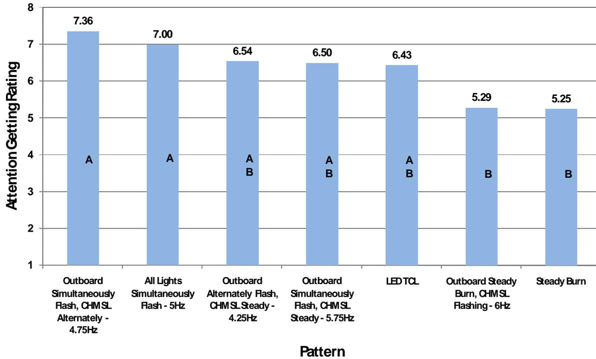
**Figure 13. Results of the Attention-Getting Ratings at 100 ft (30.5 m) Looking Directly Forward**
