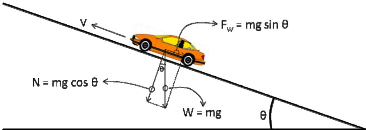
**Figure 57. Forces on a Vehicle created by an Uphill Slope**
