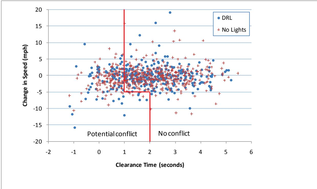
Figure 11. Potential Conflicts and Non-Conflicts for 778 Left-Turning Vehicles Based on Clearance Time and Changes in the Approaching Vehicle’s Speed (Boys Site)
