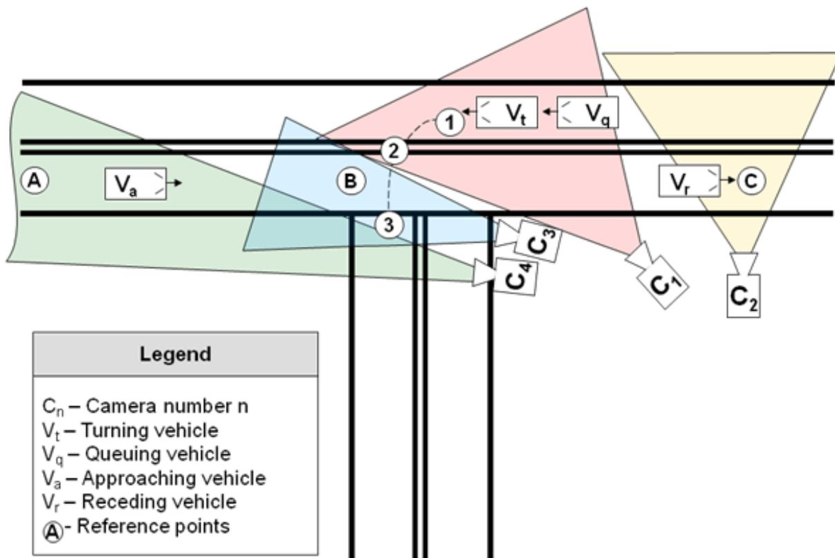
Figure 5. Simplified Plan View of an Intersection Showing Approximate Camera Coverage Zones and Reference Points
