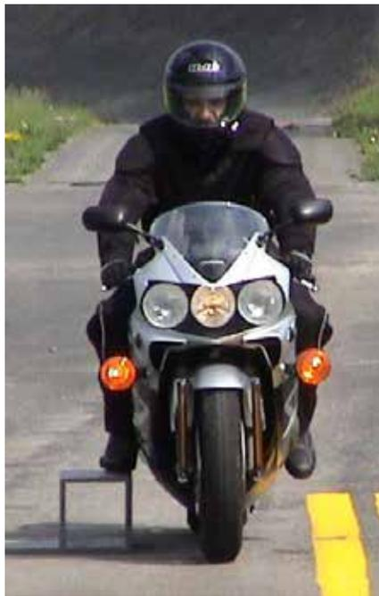
**Figure 4. Lower beam with auxiliary parking lamps**
