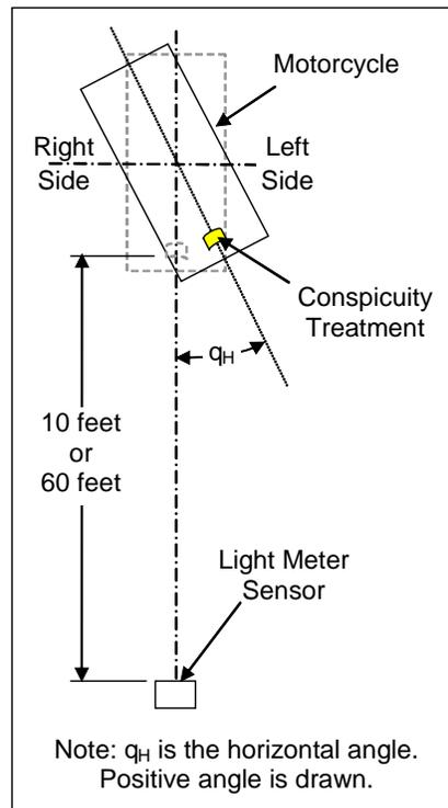
**Figure A2. Side schematic of test layouts**
