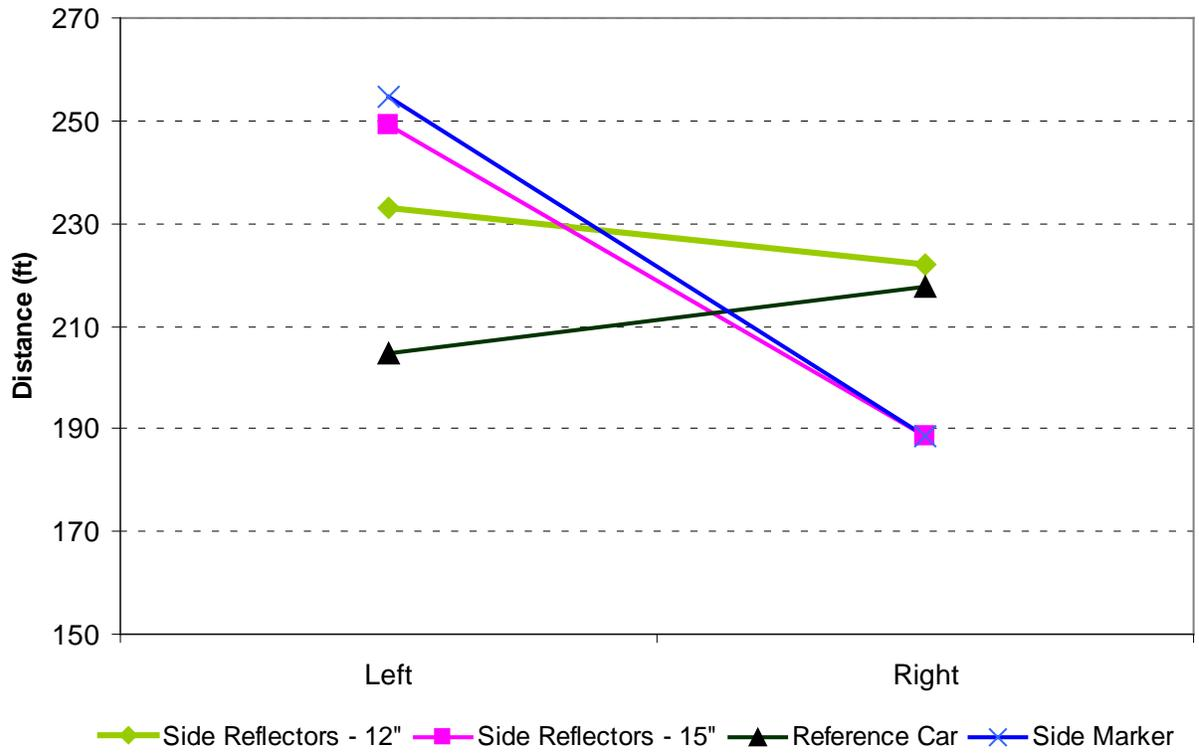
**Figure 27. Mean identification distance (feet) by direction, vehicle type**
