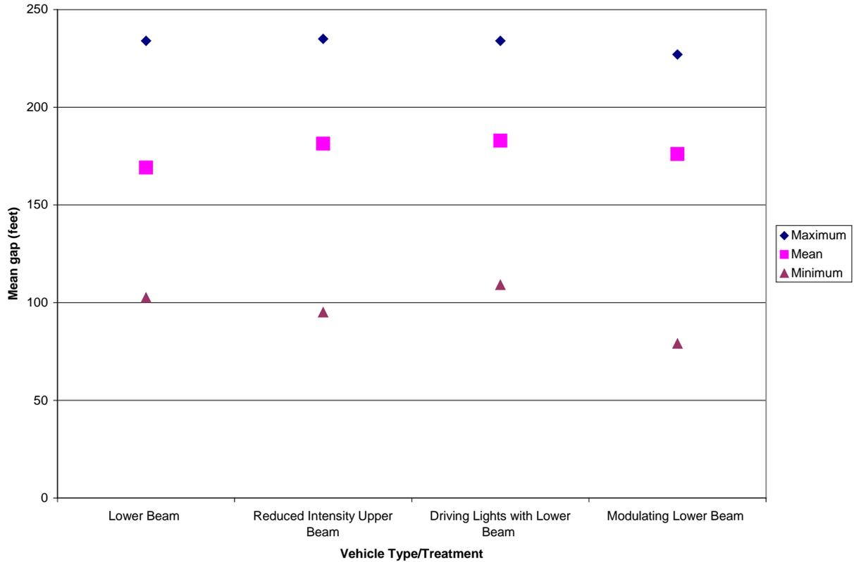
**Figure 18. Mean, maximum, and minimum gap (in feet) for all traffic by motorcycle treatment - Canada**
