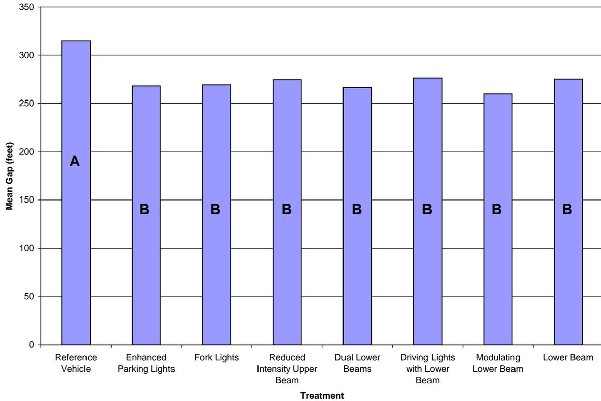
**Figure 11. Mean gap by conspicuity treatment for the test track study**
