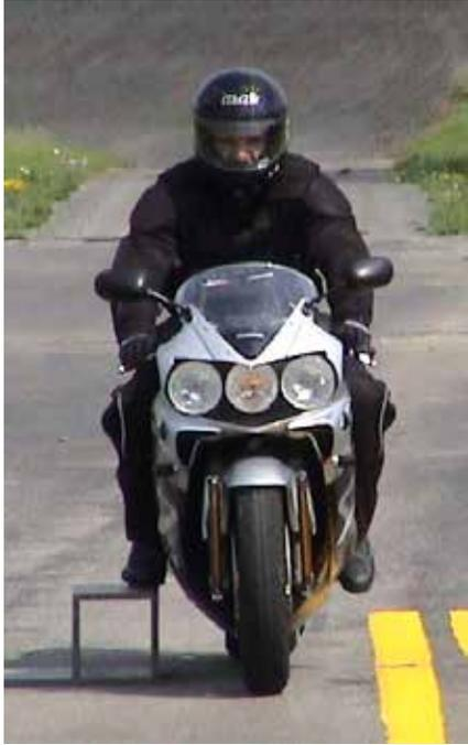
**Figure 2. Modulating lower beam**
