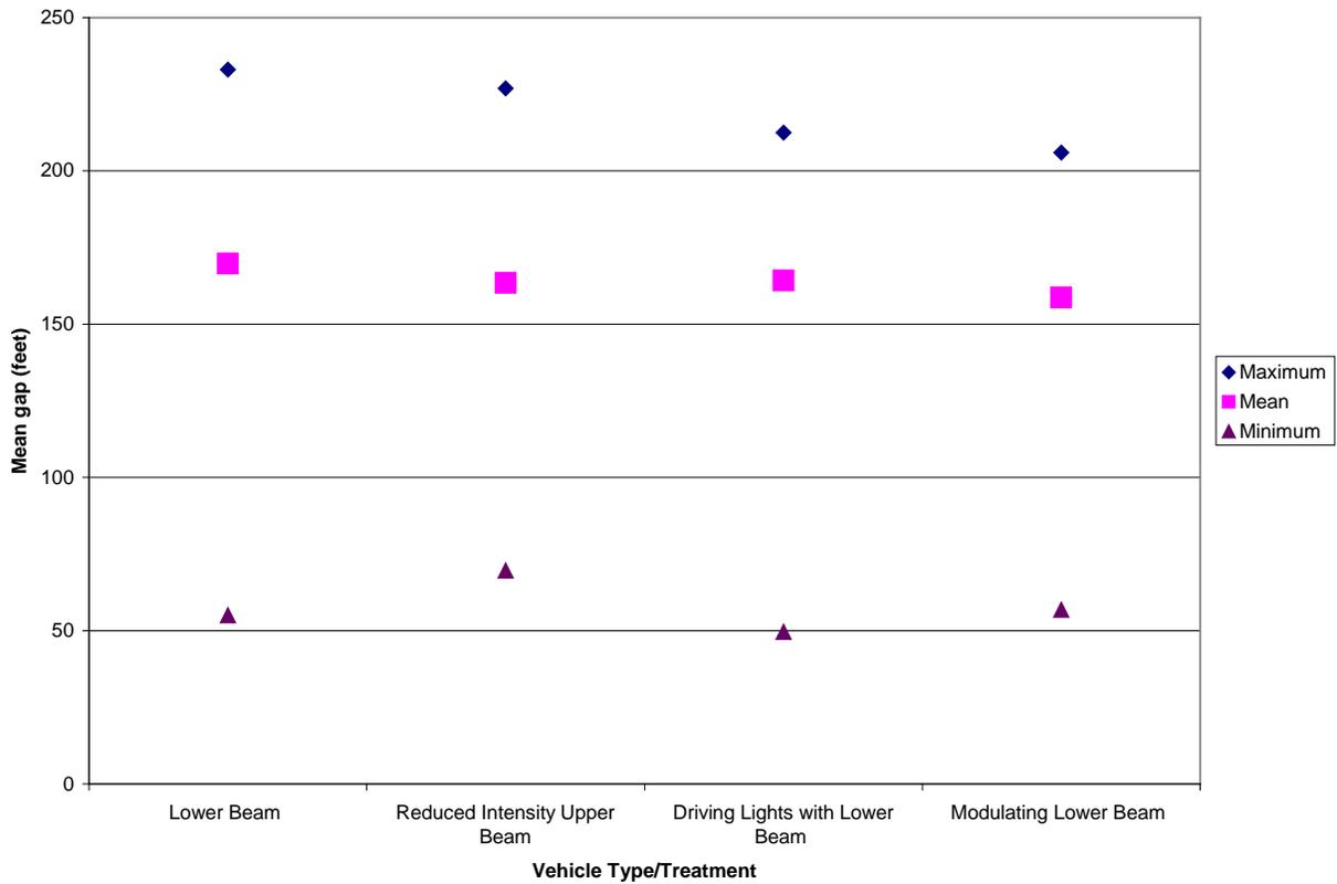
**Figure 17. Mean, maximum, and minimum gap (in feet) for all traffic by motorcycle treatment – United States**
