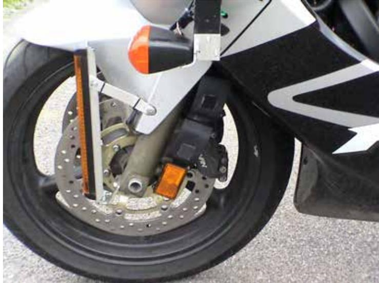
**Figure 23. Side retro-reflectors, 12” mounting location**
