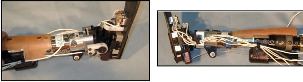
**Figure 4.3** - Foot Accelerometer and X-axis potentiometer routing
