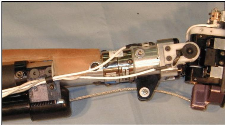
**Figure #4.2** - Tibia Uniaxial Accelerometers
