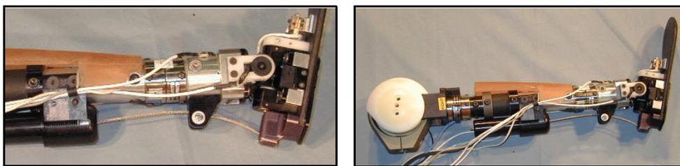
**Figure 4.4** - Y & Z Potentiometer Wire Routing
