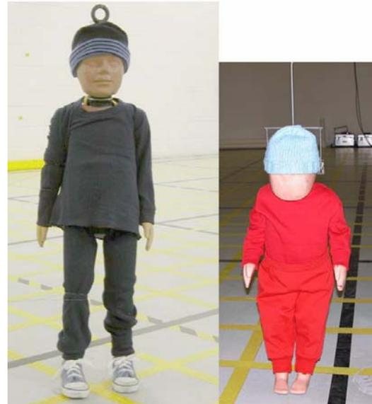
Figure 3. Photographs of ATDs used in testing
